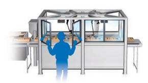
Safely-Limited Position (SLP) of the drive allows the machine to keep running.
