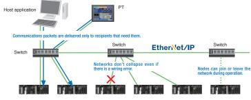
Star topology using Ethernet switch technology
