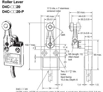
VCTF cable, VCTF oil-resistant cable: 0.75 mm², 4 conductor, Finishing O.D. 7.6 dia. SJT(O) cable: 0.83 mm², 4 conductor, Finishing O.D. 8.6 dia. D4C-□□20-P (Weather-resistant Models)
