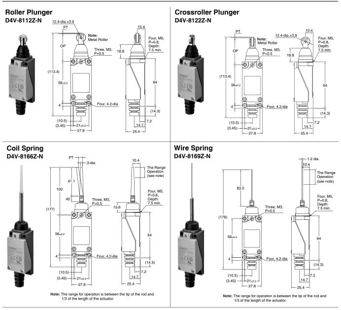
Note: Unless otherwise specified, the tolerances are ±0.4 mm for the above dimensions for each model.
