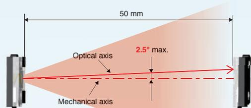
The offset between the optical axis and mechanical axis is within  $\pm 2.5^\circ$ , so a sufficient incident level can be achieved merely by aligning the mechanical axis at installation.
