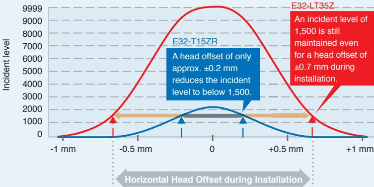
\*1. Installation distance between heads: 50 mm, Installation distance between head and slit: 5 mm, Slit diameter at emitter and receiver: 0.5 mm each (Thickness: 10 mm), and E3NX-FA11 Fiber Amplifier Unit (HS mode).
