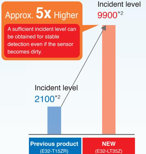
\*2. Digital incident level for the following conditions: Installation distance between heads: 50 mm, Installation distance between head and slit: 5 mm, Slit diameter at emitter and receiver: 0.5 mm each (Thickness: 10 mm), and E3NX-FA11 Fiber Amplifier Unit (HS mode).
