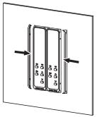
4. Secure the End Cover so that the double-sided tape is firmly attached.
