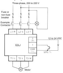
Do not operate motors that exceed the allowable capacity with G3Js connected in parallel. Doing so may result in malfunctions.
