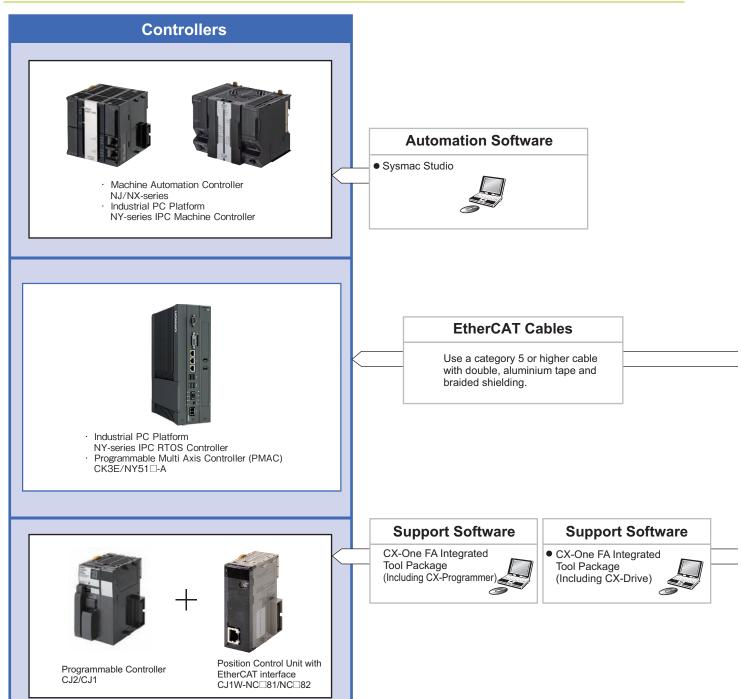
Note: PMAC is an abbreviation for Programmable Multi Axis Controller.
