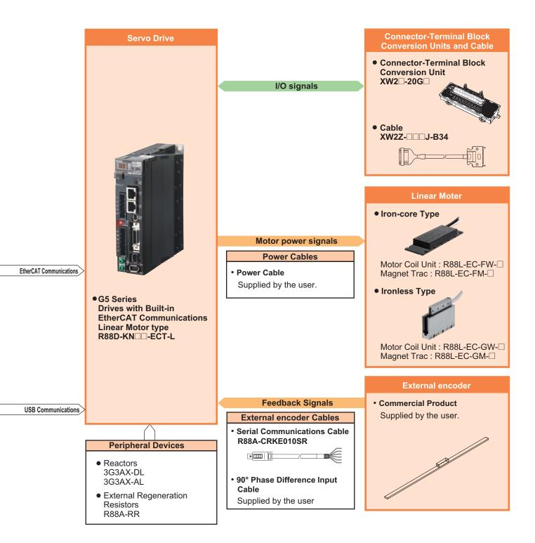
G5-series AC Servomotors/Servo Drives with General-purpose Pulse Train or Analog Inputs
