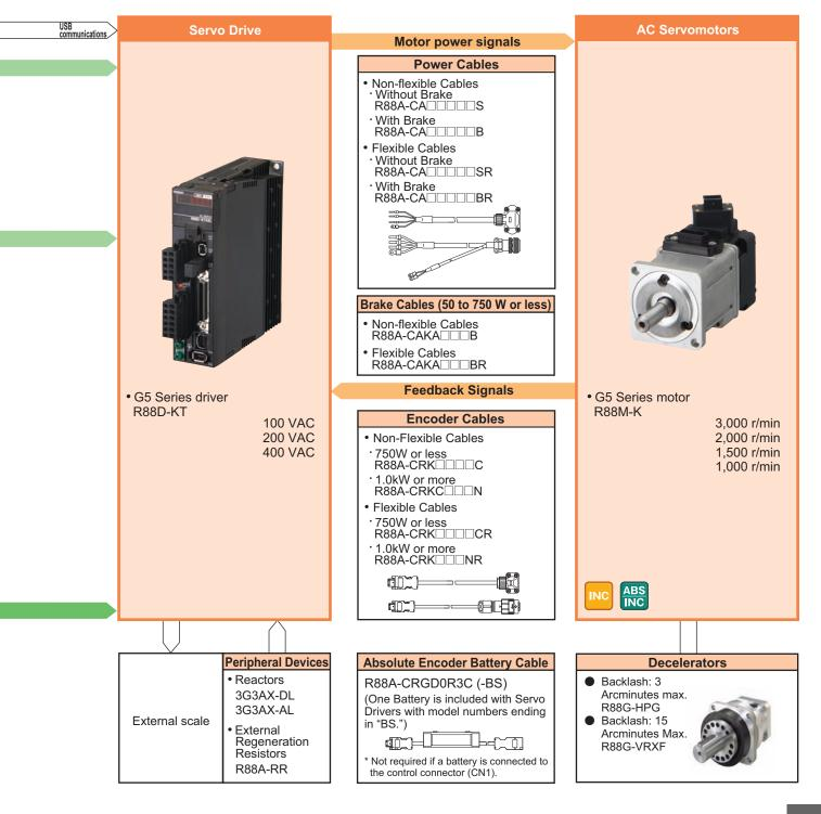
G5-series AC Servomotors/Servo Drives with Built-in MECHATROLINK-II Communications
