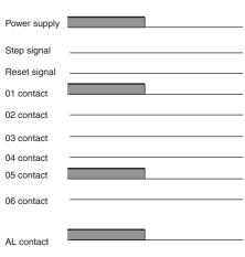
If an internal contact of the G9B is incorrectly turned ON by the internal relay driving element that drives the internal contact due to external noise, the G9B will reset itself to its default status (i.e., contact 01 of the G9B will be turned ON) and turn its alarm contact ON so that the ALARM indicator of the G9B will become lit. When the G9B is turned OFF, the alarm contact will turn OFF and the ALARM indicator will not be lit. In this example, contact 05 is incorrectly turned ON.
