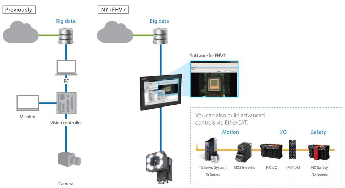
\* A separate unit is required to connect the FHV7 to EtherCAT.
