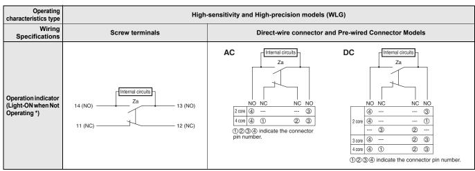
Note: Leakage current from indicator circuit may cause load malfunction (i.e., the load may remain ON). Make sure that the load operating current is higher than the leakage current. For countermeasures, refer to technical support on your OMRON website.
