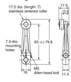
Note: Unless otherwise indicated, a tolerance of ±0.4 mm applies to all dimensions.
