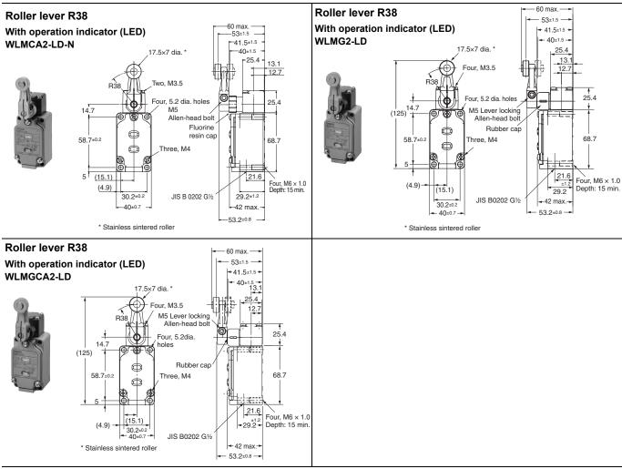
Note: Unless otherwise indicated, a tolerance of ±0.4 mm applies to all dimensions.
