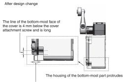
The bottom-most face of the case protrudes 4 mm from the contact surface of the cover
