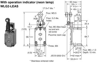
Note: The photo shows the WLG2-LDAS model.
