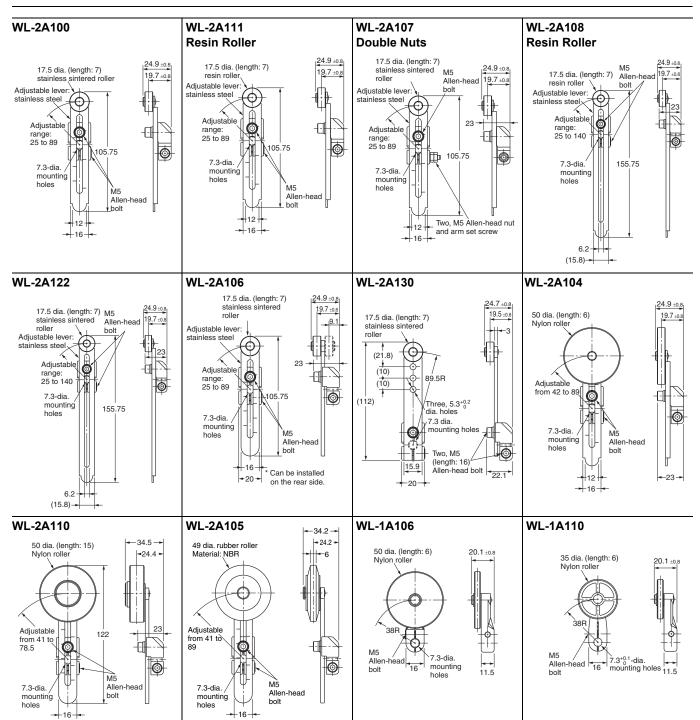
Note: Unless otherwise indicated, a tolerance of  $\pm 0.4$  mm applies to all dimensions.
