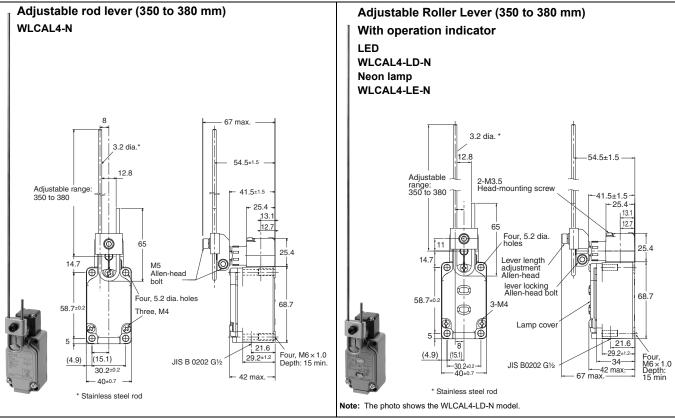
Note: Unless otherwise indicated, a tolerance of ±0.4 mm applies to all dimensions.
