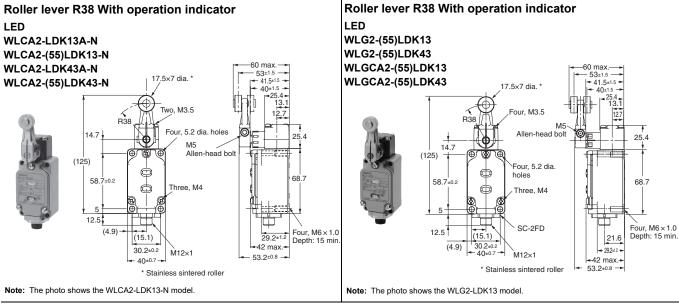
**Note:** Unless otherwise indicated, a tolerance of ±0.4 mm applies to all dimensions.
