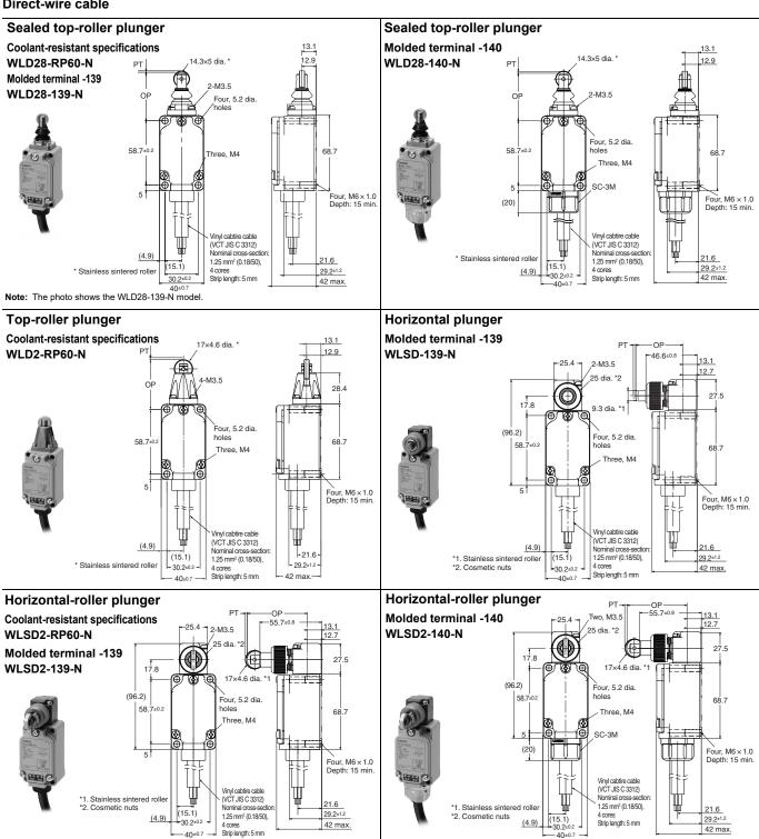
Note: Unless otherwise indicated, a tolerance of ±0.4 mm applies to all dimensions.
