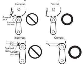
Appropriate force must be imposed on the actuator by the cam or dog in both rotary operation and linear operation. If the dog touches the lever as shown below, the operating position will not be stable.
