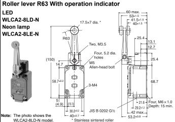
Note: Unless otherwise indicated, a tolerance of ±0.4 mm applies to all dimensions.
