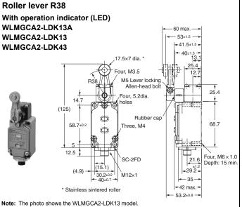
Note: Unless otherwise indicated, a tolerance of ±0.4 mm applies to all dimensions.
