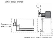
Bottom-most part of housing has a depressed shape
