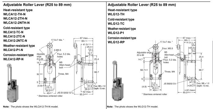
Note: Unless otherwise indicated, a tolerance of ±0.4 mm applies to all dimensions.
