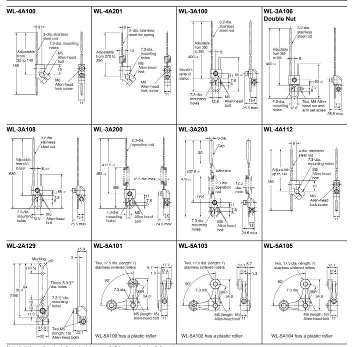
Note: 1. Unless otherwise indicated, a tolerance of  $\pm 0.4$  mm applies to all dimensions. 2. When using the adjustable roller (rod) lever, make sure that the lever is facing downwards. Use caution, as telegraphing (the Switch turns ON and OFF repeatedly due to inertia) may occur.
