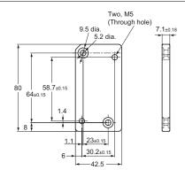
The Side mounting plate allows the actuator to be installed in the same position as the side mounting of the WL□-2N series.
