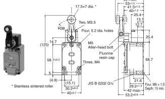
$\textbf{Note:} \ \ \mathsf{The \ photo \ shows \ the \ WLCA2\text{-}LDS\text{-}N \ model}.$
