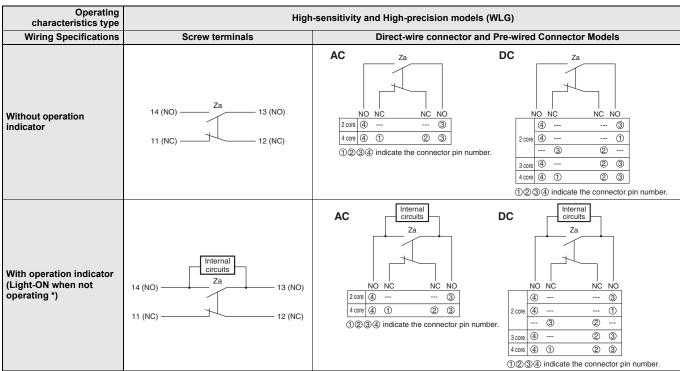
Note: Leakage current from indicator circuit may cause load malfunction (i.e., the load may remain ON). Make sure that the load operating current is higher than the leakage current.
