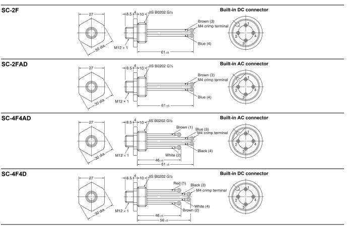
Note: 1. Each dimension has a tolerance of  $\pm 0.4$  mm unless otherwise specified.
