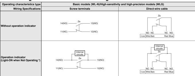
**Note:** Leakage current from indicator circuit may cause load malfunction (i.e., the load may remain ON). Make sure that the load operating current is higher than the leakage current.
