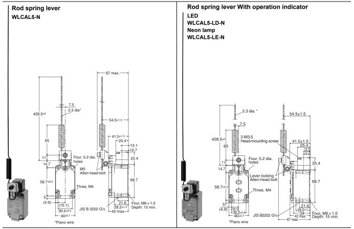
Note: Unless otherwise indicated, a tolerance of ±0.4 mm applies to all dimensions.
