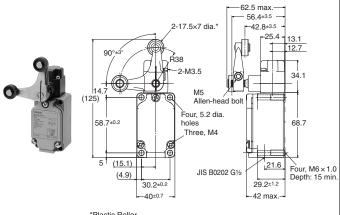
\*Plastic Roller (The WLCA32-041-N to WLCA32-044-N have stainless sintered rollers.) Note: The photo shows the WLCA32-43-N model.
