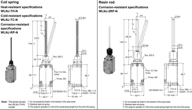
**Note:** Unless otherwise indicated, a tolerance of ±0.4 mm applies to all dimensions.
