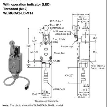
Note: Unless otherwise indicated, a tolerance of ±0.4 mm applies to all dimensions.
