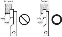
With a roller actuator, the dog must touch the actuator at a right angle. The actuator or shaft may deform or break if the dog touches the actuator (roller) at an oblique angle.
