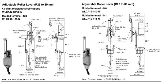
**Note:** Unless otherwise indicated, a tolerance of  $\pm 0.4$  mm applies to all dimensions.
