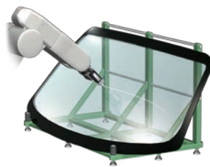
Curvature measurement of glass surfaces
