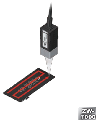
Flatness measurement of batteries
