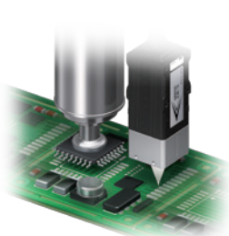
Z axis adjustment of chip mounter
