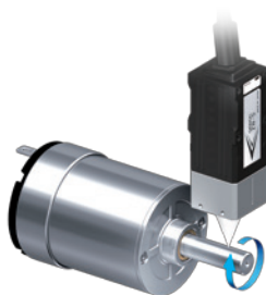
Eccentricity measurement of motors
