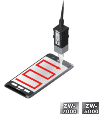
Flatness measurement of cover glass
