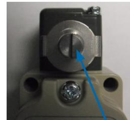
When the lever is normal, the groove is not at an angle.
