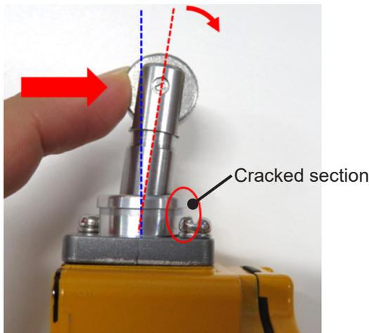
Cracks occur by being repeatedly subjected to excessive force.
