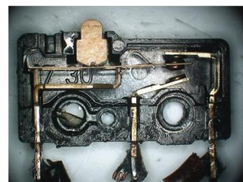
In the case example this time, as a result of analyzing the components, carbon and oxygen have been detected, and there is the possibility that oil liquid has entered inside the switch.
