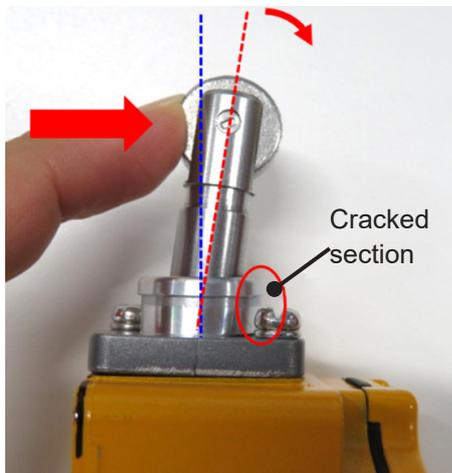
Cracks occur by being repeatedly subjected to excessive force.
