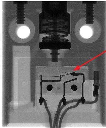
The contact is welded and detached protrusions are visible.
