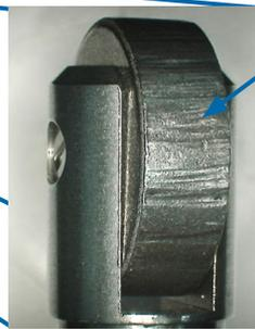
There are many pronounced dents around the entire circumference of the roller. These dents are the result of contact with the operating body under a heavy load.
