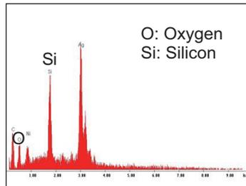
Silicon oxide detected
