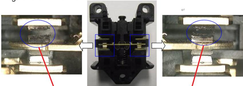
The contact is welded and detached protrusions are visible.
