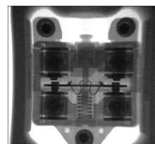
Movable piece comes loose and causes damage to the inside.
