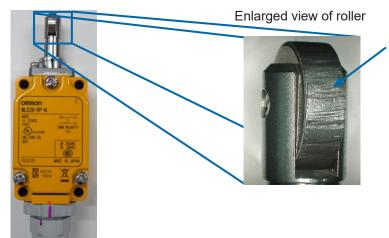
There are many pronounced dents around the entire circumference of the roller. These dents are the result of contact with the operating body under a heavy load.
