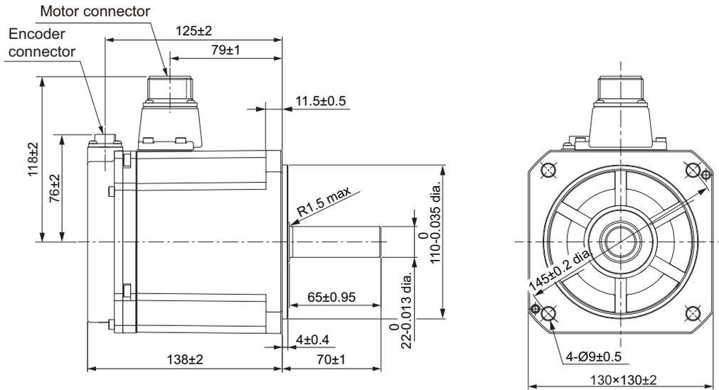
**Note** The standard shaft type is a straight shaft. Models with a key and tap are indicated with "S2" at the end of the model number.
