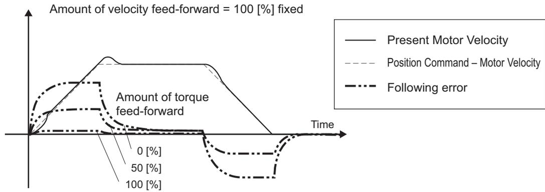
You can reduce the following error in a constant acceleration range by using the torque feed-forward.
