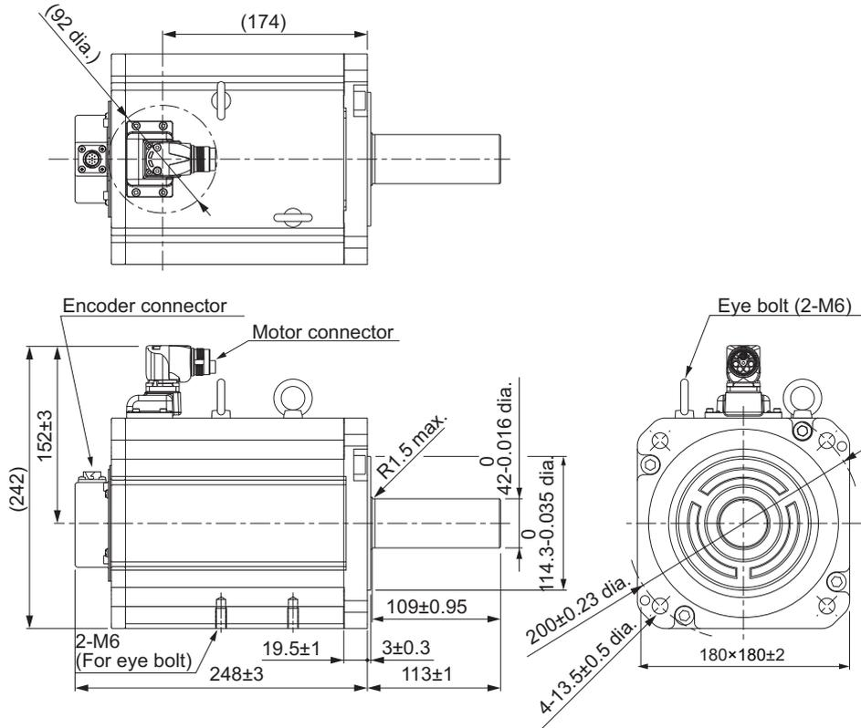
**Note** The standard shaft type is a straight shaft. Models with a key and tap are indicated with "S2" at the end of the model number.
