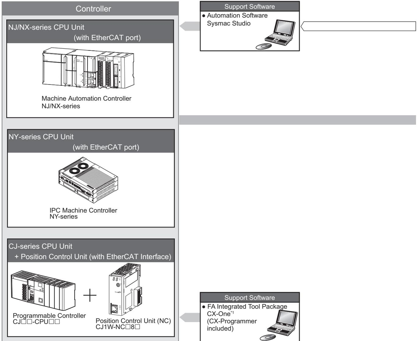
\*1. You cannot use the CX-One to make the settings of 1S-series Servo Drives with Built-in EtherCAT Communications. Obtain the Sysmac Studio.
