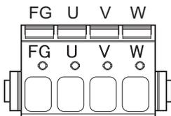
● **Main Circuit Connector E (CNE) Specifications**
