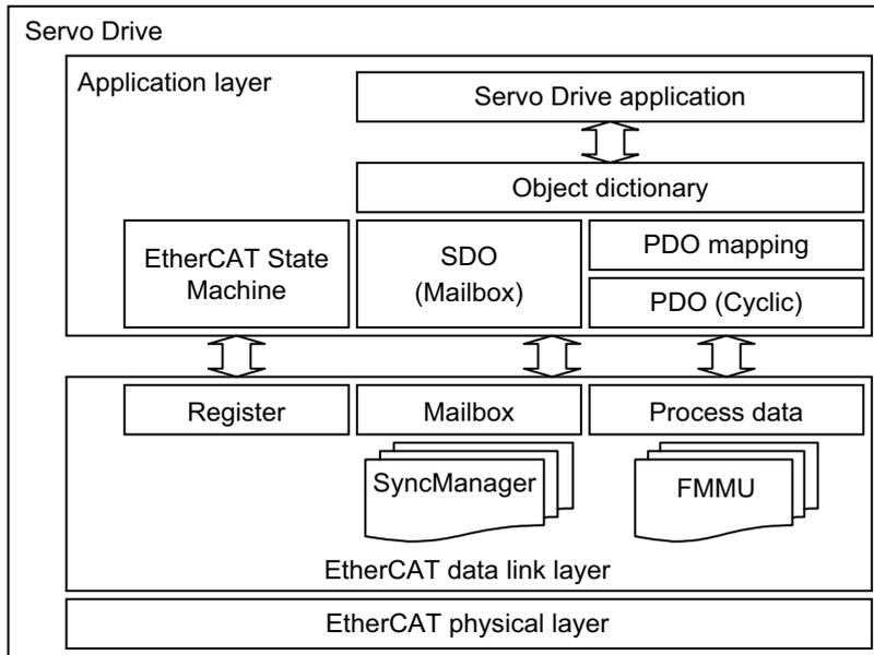
Normally, EtherCAT can transmit different protocols. 1S-series Servo Drives use the IEC 61800-7 (CiA 402) drive profile.
