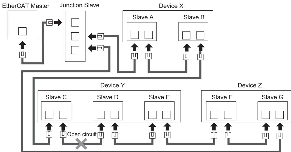
Stop Device X to Z and then turn OFF the power supply to the EtherCAT master. Fix the ring disconnection status by replacing the cable, and then turn ON the power supply to the EtherCAT master and to the devices, which returns the system to the normal communications status.
