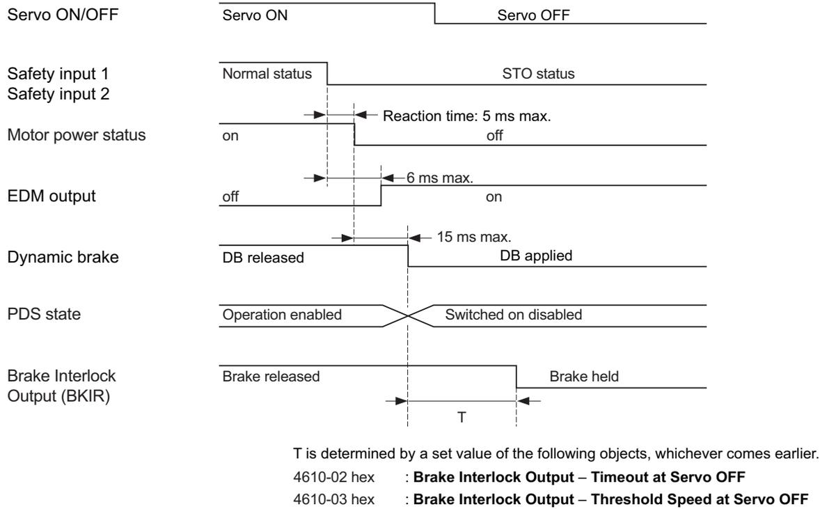
The Servo Drive goes into the STO status when either safety input 1 or 2 turns OFF. The dynamic brake operates according to the setting of the **Stop Selection – Shutdown Option Code** (3B20-01 hex).
