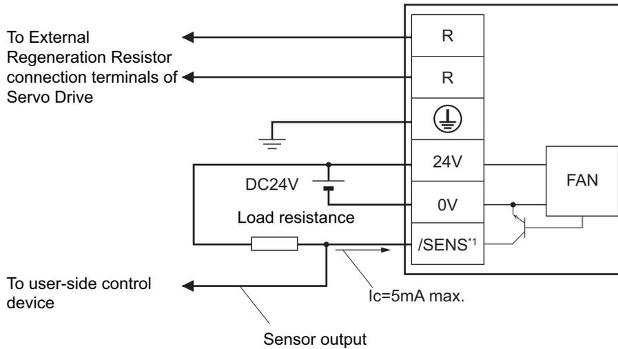
\*1. Build a system to prevent the Servomotor from operating if a fan error is detected by the /SENS signal.
