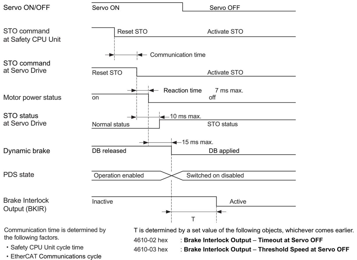
The dynamic brake operates according to the setting of the **Stop Selection – Shutdown Option Code** (3B20-01 hex).
