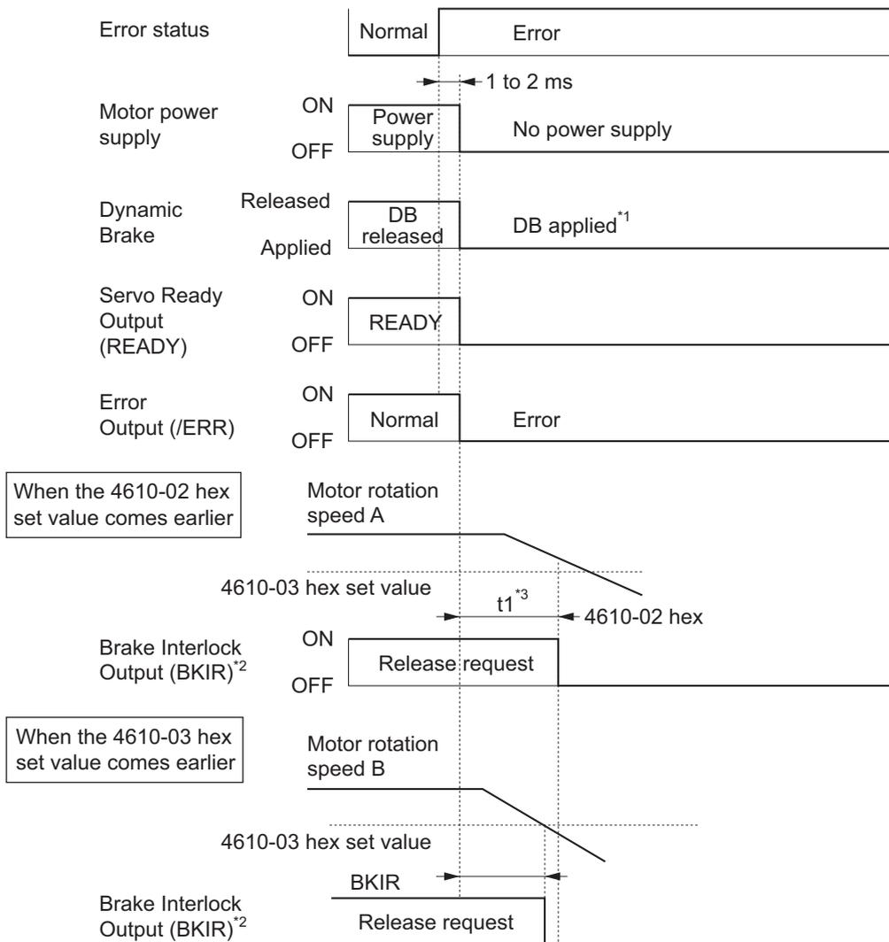
\*1. The operation of the dynamic brake when there is an error depends on the set value in the **Stop Selection – Fault Reaction Option Code** (3B20-04 hex).
