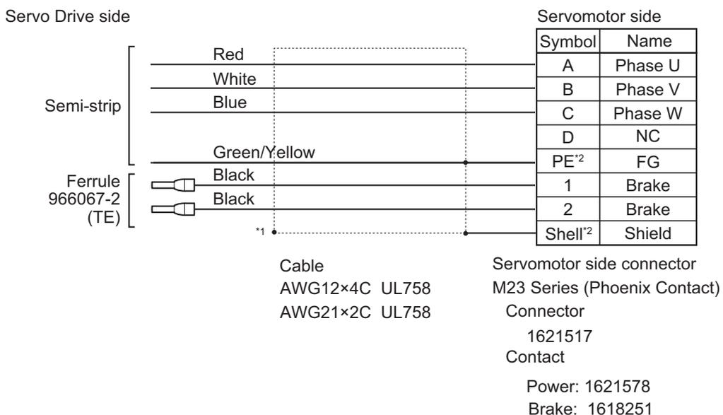
\*1. Connect the cable to the servo drive enclosure using the shield clamp.
