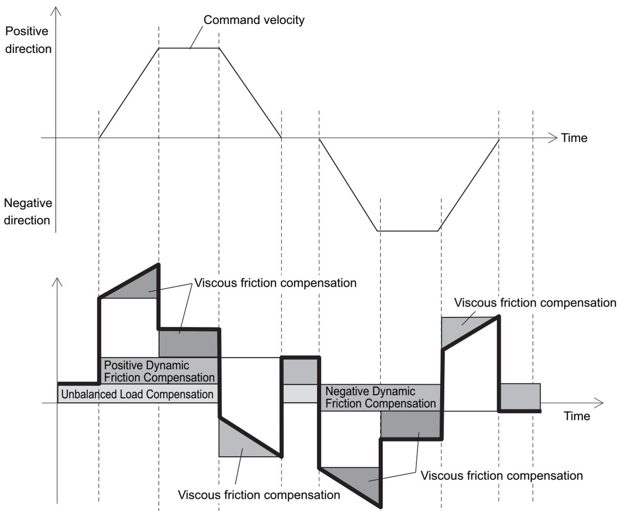
**Note** The dynamic friction compensation holds the compensation value until the command direction changes, in order to sustain the position during stabilization.
