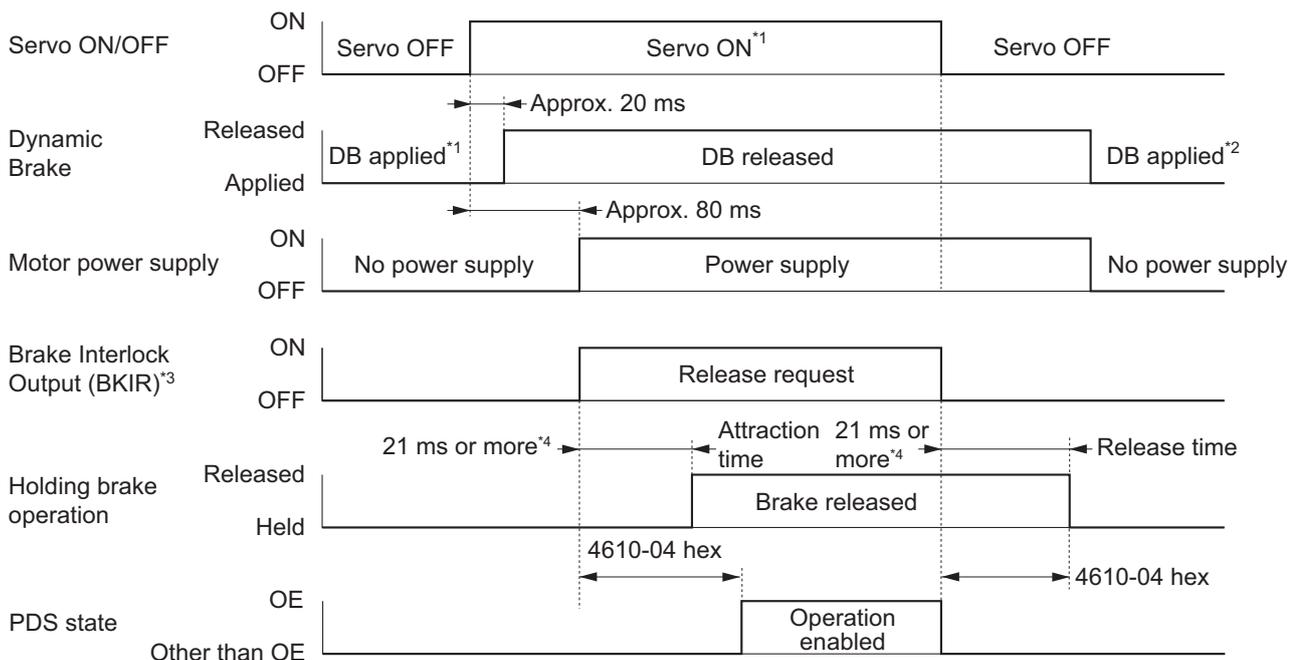
\*1. The Servo does not turn ON until the motor rotation speed drops to approximately 30 r/min or lower.
