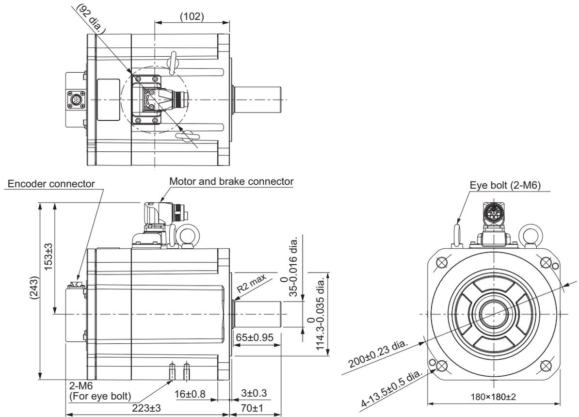
**Note** The standard shaft type is a straight shaft. Models with a key and tap are indicated with "S2" at the end of the model number.
