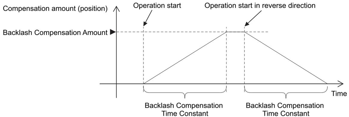
To determine the actual position of the Servomotor, the Servomotor position data acquired via EtherCAT communications is offset by the Backlash Compensation Amount.
