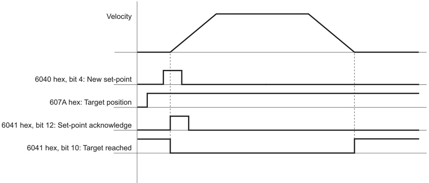
You can change the target value while PTP positioning is in progress.
