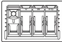
● **Main Circuit Connector E (CNE) Specifications**
