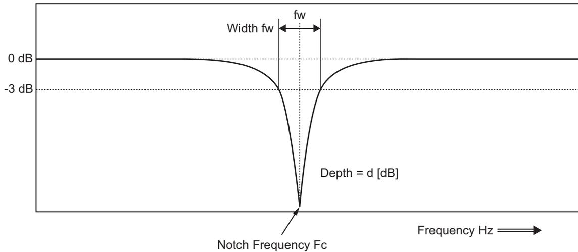
If mechanical resonance occurs, use this notch filter to eliminate resonance.
