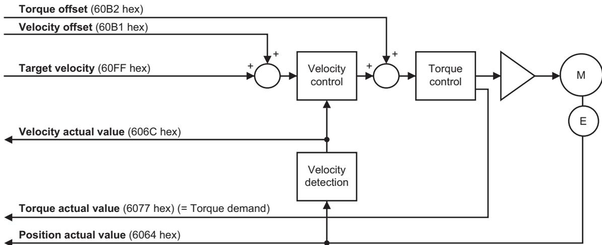
The following diagram shows the configuration of the control function of the Cyclic synchronous velocity mode.
