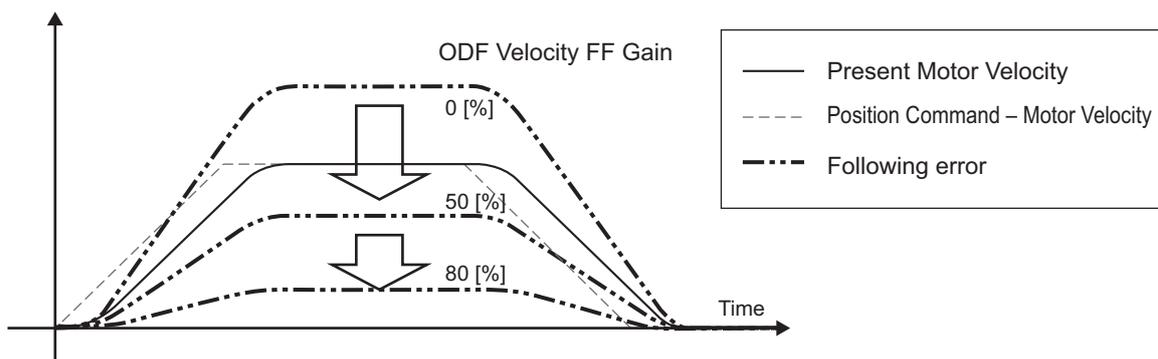
The following error in a constant velocity range gets smaller as you increase the velocity feed-forward gain.
