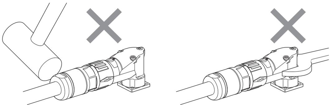
Do not pull out a cable during the change of cable outlet direction. Doing so may cause failures of a connector and a cable.
