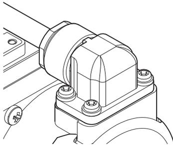
**Note** Make sure that the connector is securely fitted into place without a gap or tilt.
