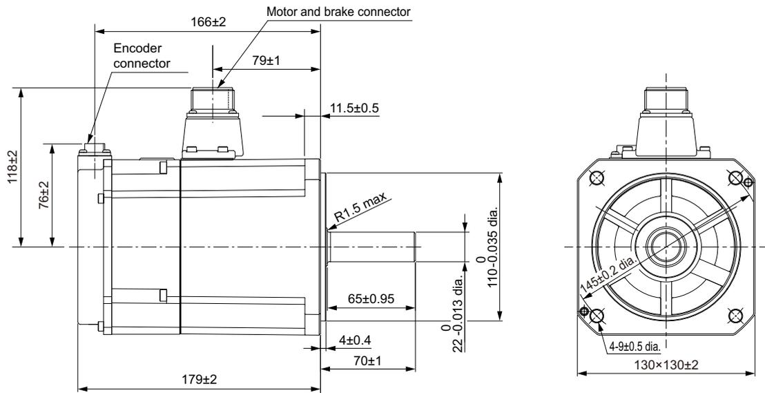
**Note** The standard shaft type is a straight shaft. Models with a key and tap are indicated with "S2" at the end of the model number.
