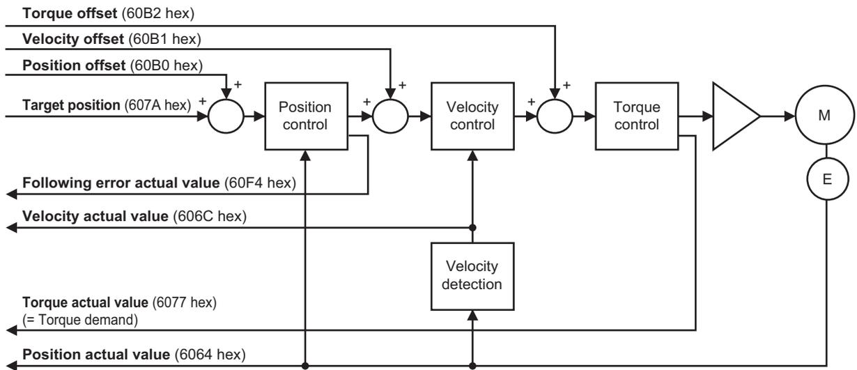
The following diagram shows the configuration of the control function of the Cyclic synchronous position mode.
