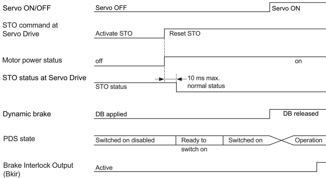
The STO is also activated if a hardware failure is detected during the self diagnosis. In this case, the STO remains active until the power is turned OFF.
