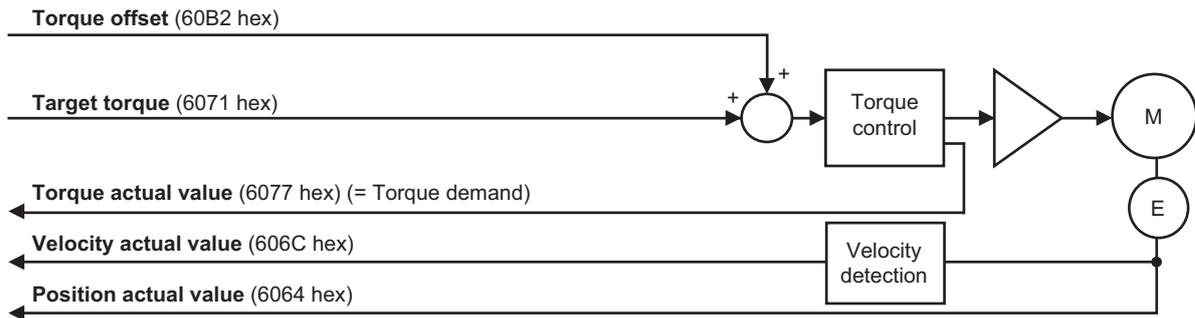
The following diagram shows the configuration of the control function of the Cyclic synchronous torque mode.
