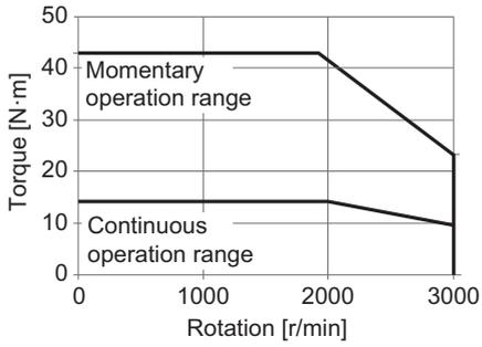
**Note** The continuous operation range is the range in which continuous operation is possible at an ambient temperature of 40°C when the Servomotor is horizontally installed on a specified radiator plate. Continuous operation at the maximum speed is also possible. However, doing so will reduce the output torque.
