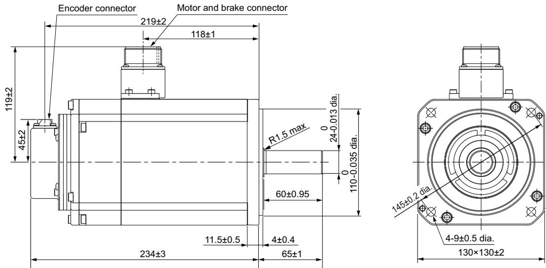
**Note** The standard shaft type is a straight shaft. Models with a key and tap are indicated with "S2" at the end of the model number.
