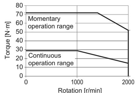
**Note** The continuous operation range is the range in which continuous operation is possible at an ambient temperature of 40°C when the Servomotor is horizontally installed on a specified radiator plate. Continuous operation at the maximum speed is also possible. However, doing so will reduce the output torque.
