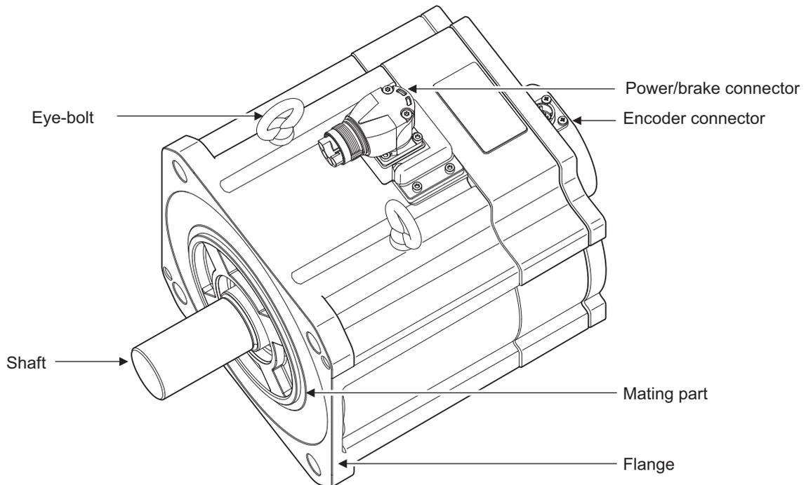
200 VAC 4 kW Servomotors (with Brake)
