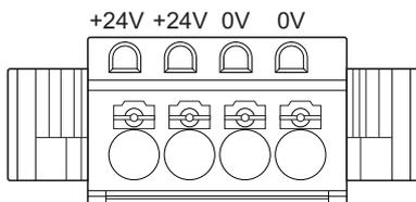
● **Motor Terminal Block (CNC) Specifications**
