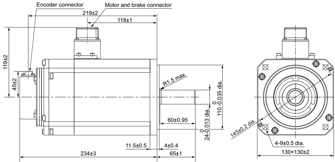
**Note** The standard shaft type is a straight shaft. Models with a key and tap are indicated with "S2" at the end of the model number.
