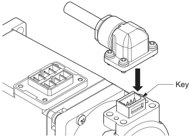
**2** Tighten the screws to fix the connector after it is fitted.
