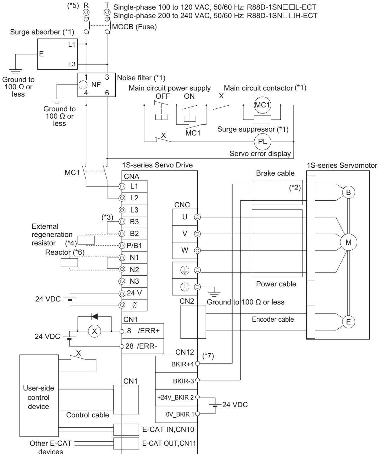
\*1. Use one noise filter for each Servo Drive. Selecting an unsuitable noise filter may result in a poor noise reduction effect. Also, a Servo Drive may produce some noise that travels through the power supply cable and causes unintended operation of other Servo Drives such as regeneration operation and Overvoltage Error.
