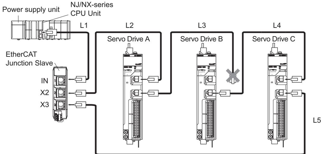
The ring disconnection status may have resulted not because an EtherCAT communications cable is disconnected, but because a communications cable is broken or short-circuited, or because a Servo Drive broke down. If the ring disconnection status occurs, immediately perform inspection and take appropriate measures. Refer to *13-5 Method for Ring Disconnection Maintenance and Inspection* on page 13-9 for details on the inspection method.
