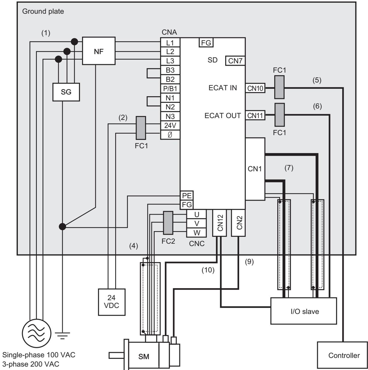
**Note** For single-phase inputs, connect between any two phases out of the following: L1, L2, and L3.
