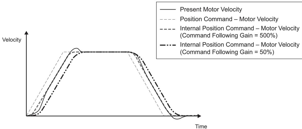
The smaller the set value of Command Following Gain is, the more the overshooting can be suppressed.
