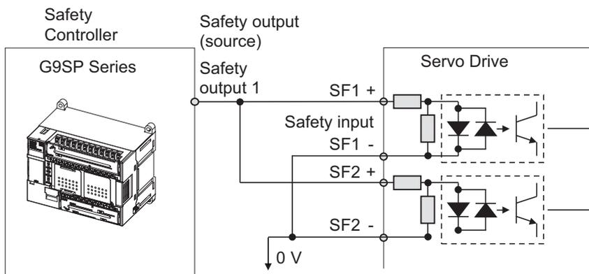
**Connection with a Safety Controller (Multiple Servo Drives)**
