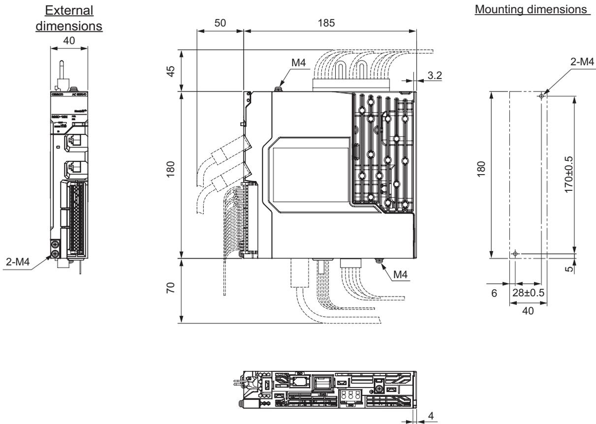
**Single-phase 100 VAC: R88D-1SN02L-ECT (200 W), Single-phase/3-phase 200 VAC: R88D-1SN04H-ECT (400 W)**
