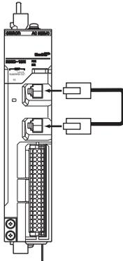
**5** Replace the identified faulty Servo Drive.
