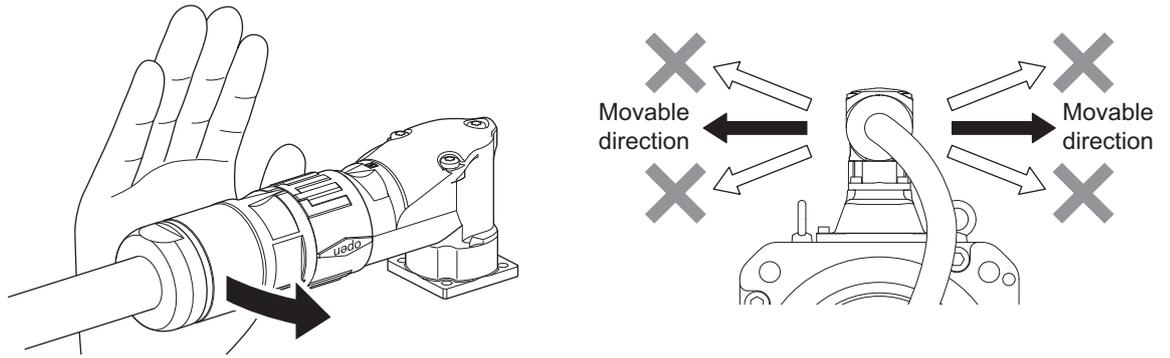
Use your hand, instead of tool, etc. when changing the cable outlet direction. Otherwise, a large amount of force is applied easily even toward not-specified direction and may cause failure of the connector.
