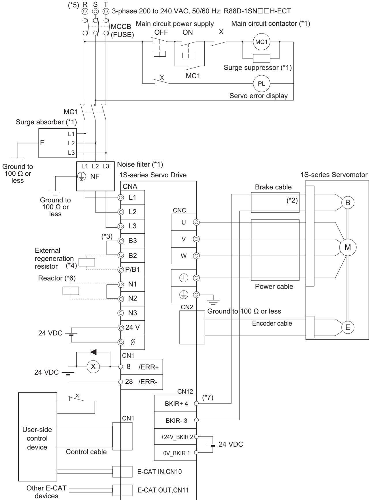
\*1. Use one noise filter for each Servo Drive. Selecting an unsuitable noise filter may result in a poor noise reduction effect. Also, a Servo Drive may produce some noise that travels through the power supply cable and causes unintended operation of other Servo Drives such as regeneration operation and Overvoltage Error.
