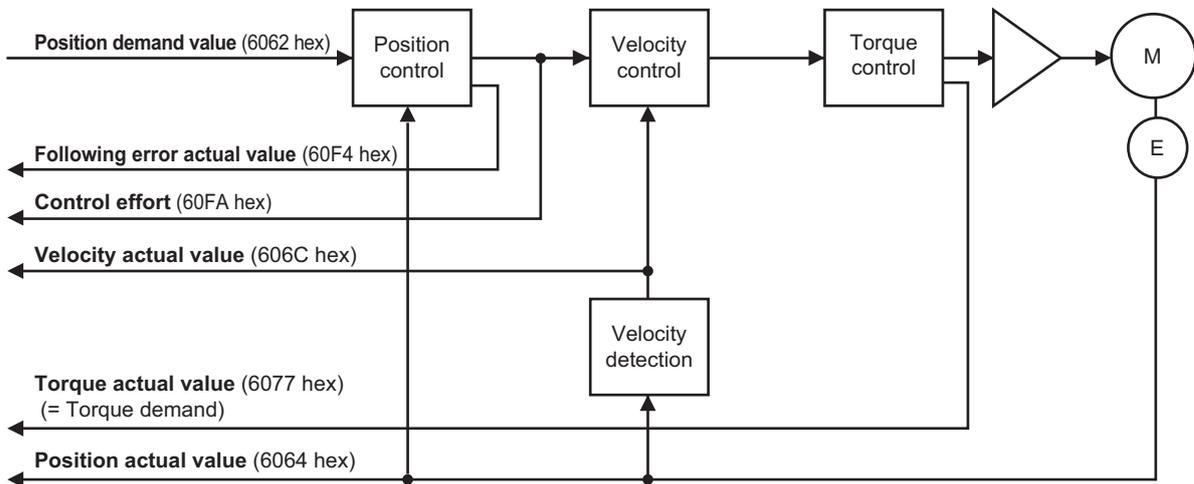
The following diagram shows the control function configuration of Profile position mode.
