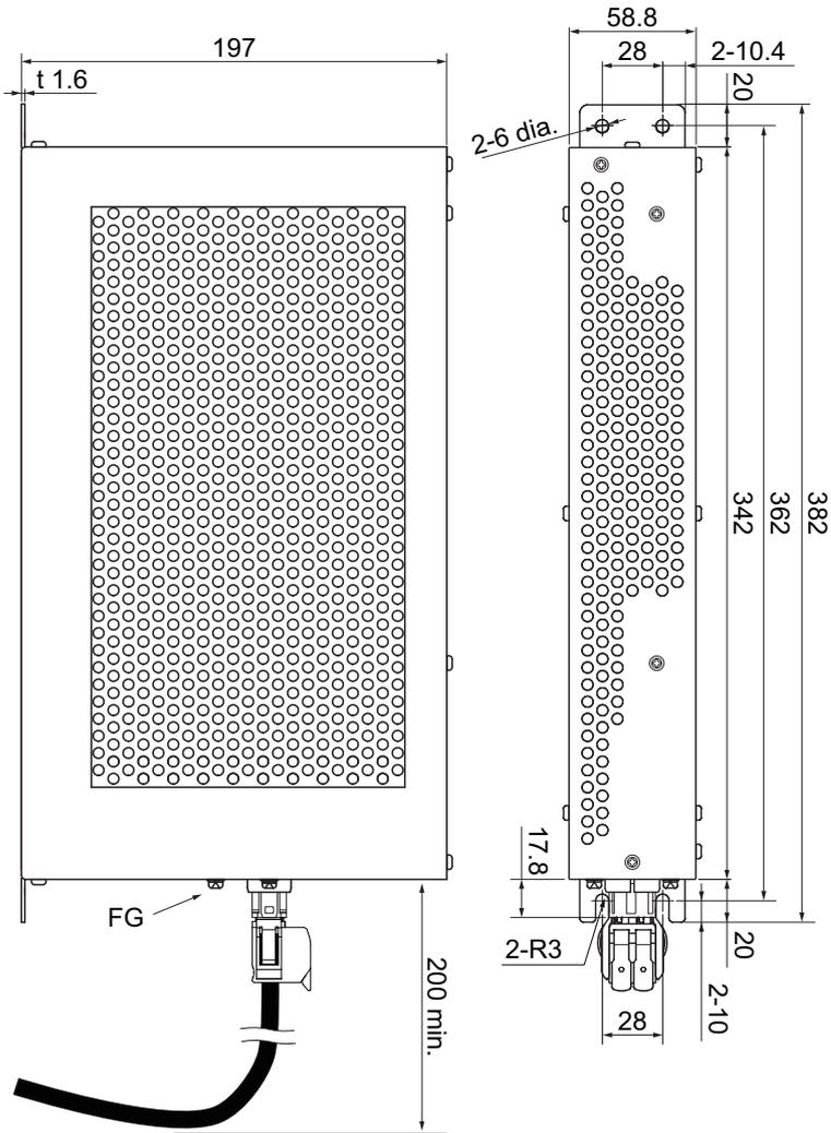
**2-4-7 Dimensions of External Dynamic Brake Resistors**
