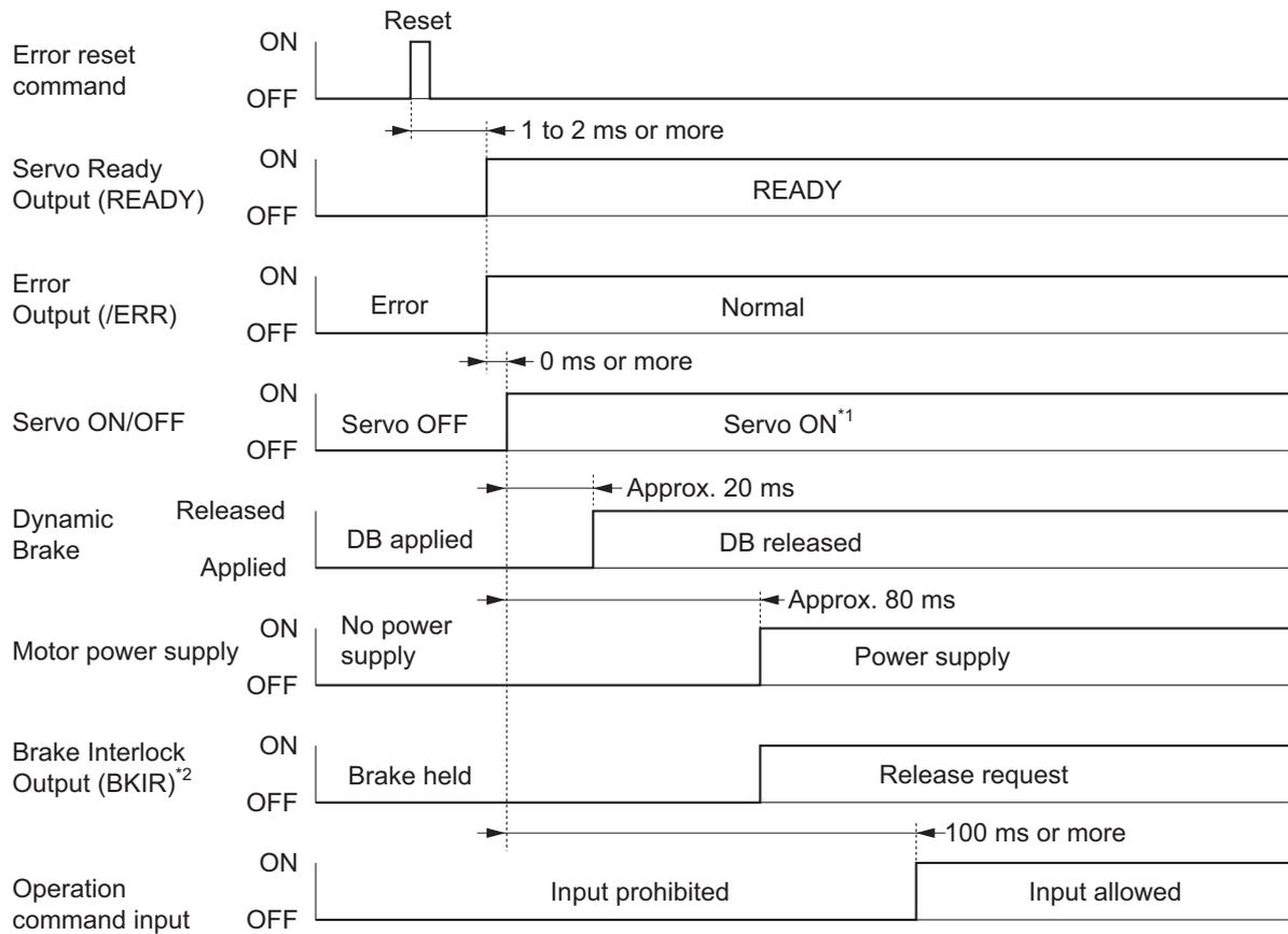
\*1. The Servo does not turn ON until the motor rotation speed drops to approximately 30 r/min or lower.
