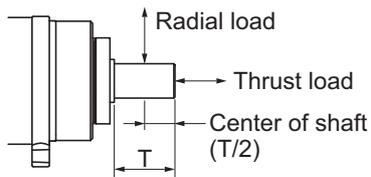
**Note 4.** The standard shaft type is a straight shaft.
