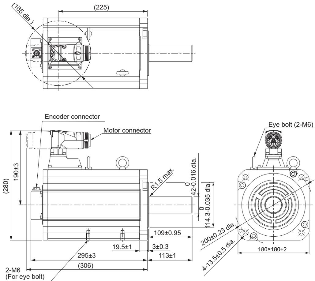
**Note** The standard shaft type is a straight shaft. Models with a key and tap are indicated with "S2" at the end of the model number.
