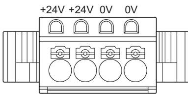
● **Motor Connector (CNC) Specifications**
