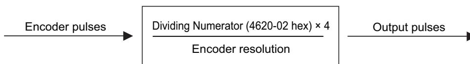
$$\text{Number of output pulses per rotation} = \text{Encoder Dividing Numerator (4620-02 hex)} \times 4$$
