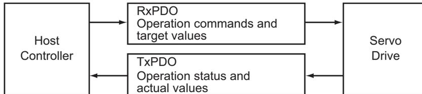
The EtherCAT application layer can hold multiple objects to enable transferring Servo Drive process data. The contents of the process data are described in the PDO mapping objects and the Sync Manager PDO Assignment objects.
