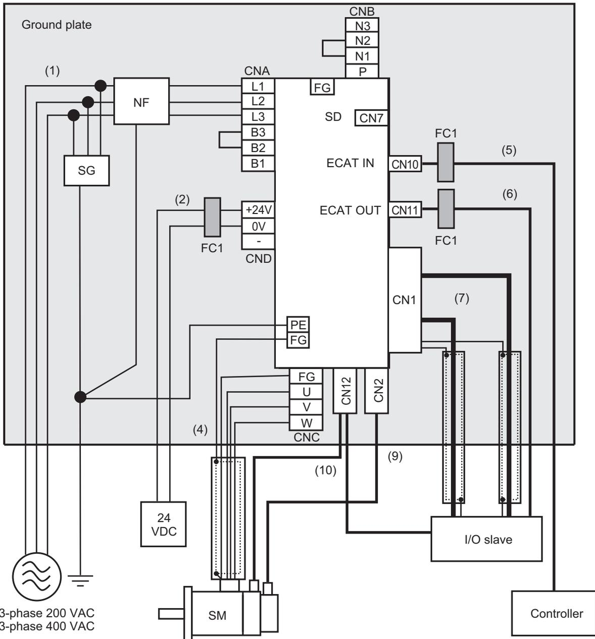
**Note** For single-phase inputs, connect between any two phases out of the following: L1, L2, and L3.
