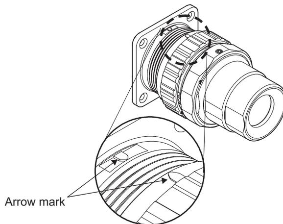
**Note** Before starting the fitting procedure, make sure that there is no dirt, foreign materials, etc. adhered to the fitting surfaces.
