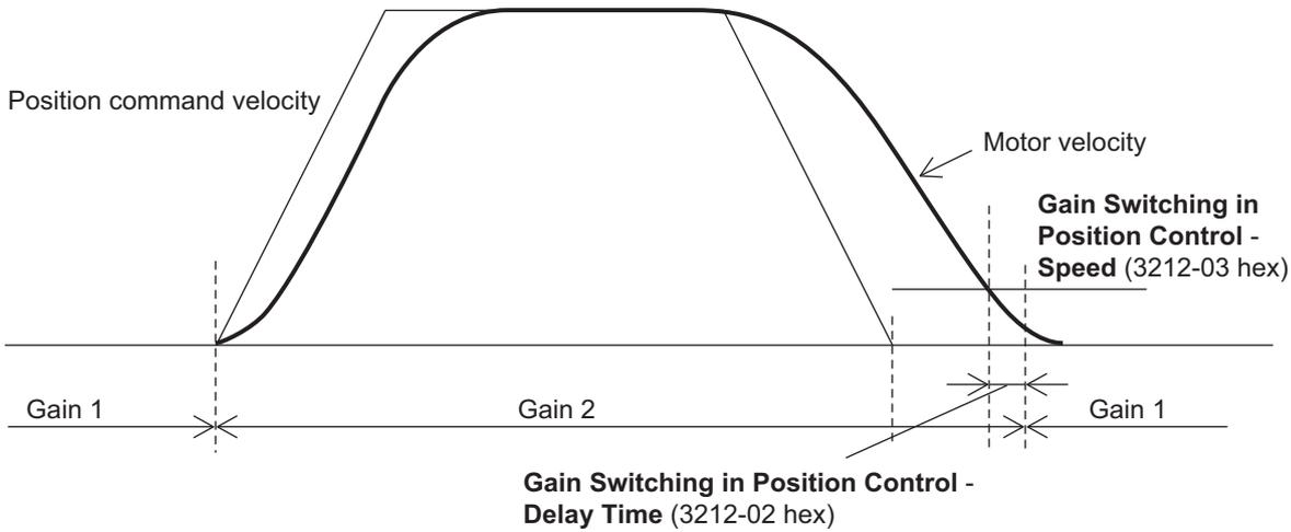
After Gain 2 switched to Gain 1, the Gain 1 is held even if overshooting occurs and the motor velocity exceeds the **Gain Switching in Position Control – Speed** (3212-03 hex).
