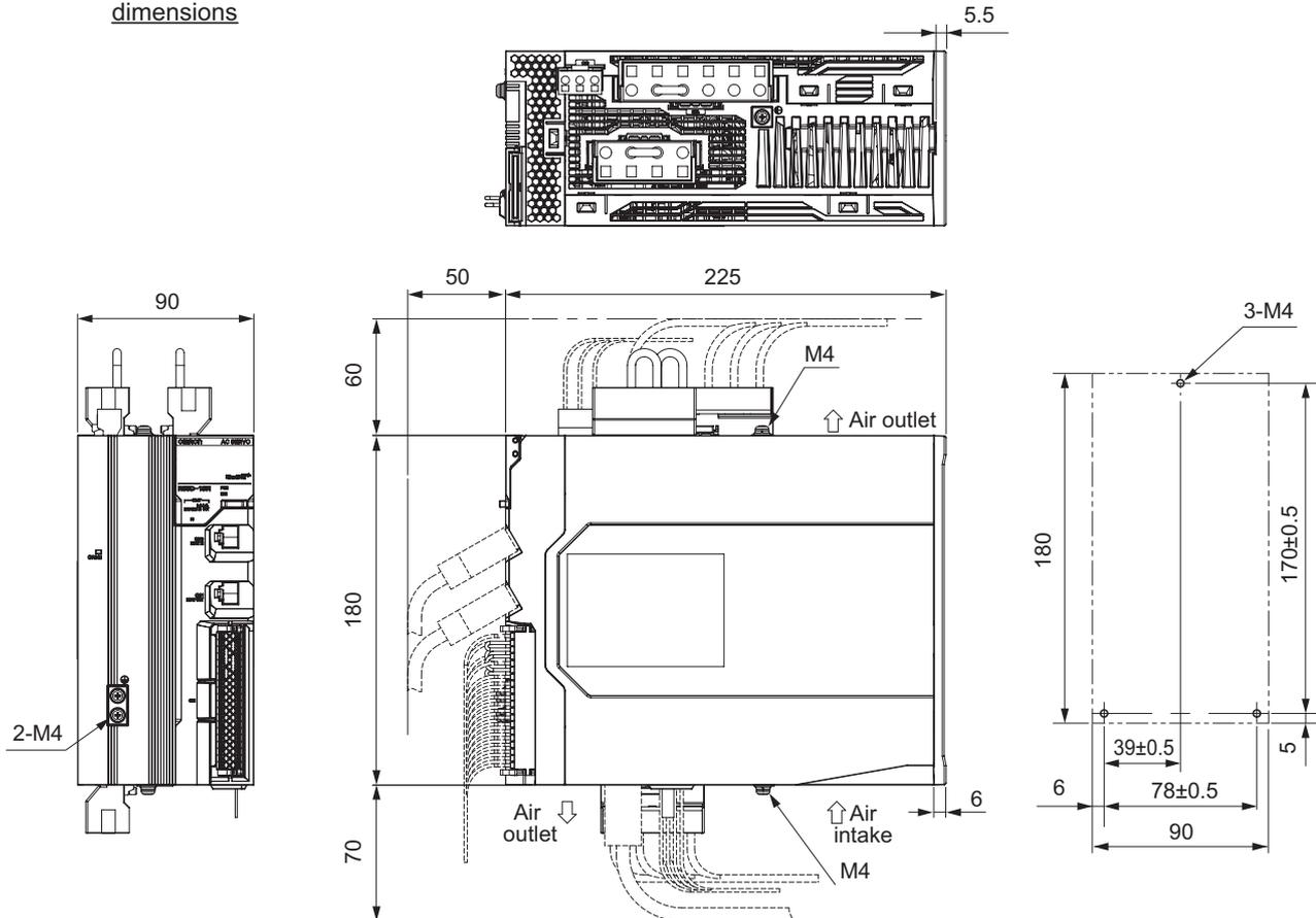
**3-phase 200 VAC: R88D-1SN55H-ECT/ -1SN75H-ECT (5.5 to 7.5 kW),
