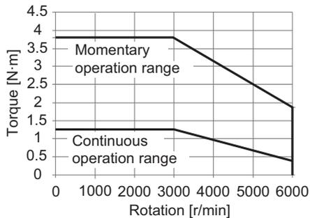
**Note** The continuous operation range is the range in which continuous operation is possible at an ambient temperature of 40°C when the Servomotor is horizontally installed on a specified radiator plate.
