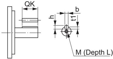
\*3. The tolerance is "h8" for R88G-HPG50□ and R88G-HPG65□.
