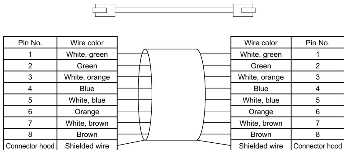
**Note 1.** Connect the cable shield to the connector hood at both ends of the cable.
