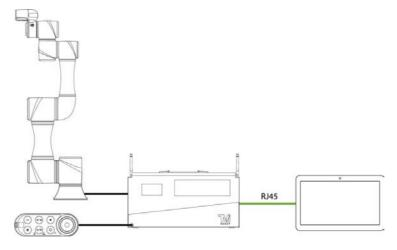
Figure 13: Wired Network Connection Method (2/2)
