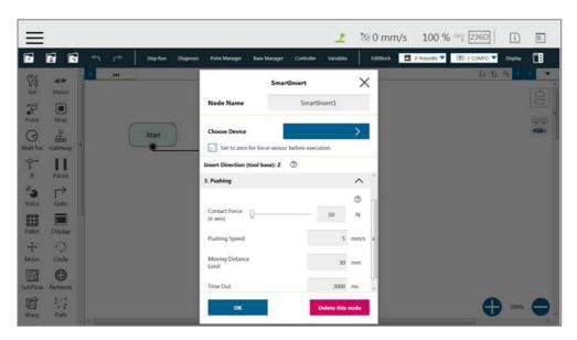
Figure 231: Pushing Parameter Interface
