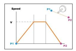
Figure 121: Speed of Line Motion
