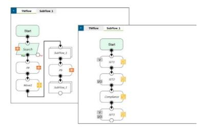
Figure 166: Subflow Node Modularization Concept
