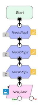
Figure 106: Create a New Base with Three Dynamic Points
