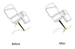
Figure 97: Tool Shift Using Keep Pose
