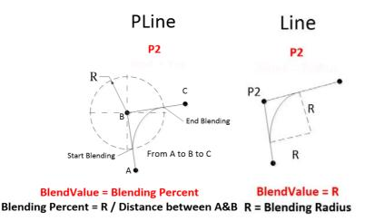
Figure 129: Set the Blending Percentage or Set the Blending by Radius
