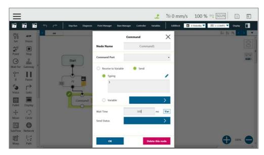
Figure 190: Set and Open Serial Port (2/2)
