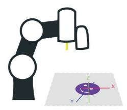
Figure 89: Servoing Vision Base is on the Camera
