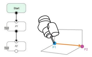
Figure 123: Line Application Example
