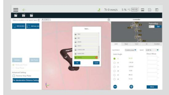
The icon before the file name denotes the operation space comes with the scenery file, and the object name and its dependent base will be shown at the top right of the 3D viewer when moving the mouse cursor on the object in the scenery file.
