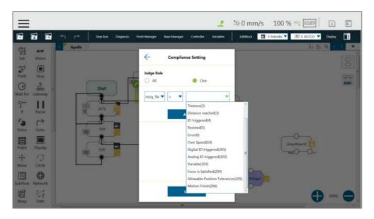
Figure 159: IF Node Stop Criteria Setting
