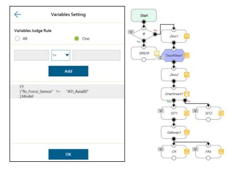
Figure 258: The Example of Making Parameterized Devices
