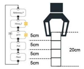
Figure 138: Plan for the Move Node
