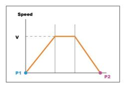
Figure 117: Speed of PTP Motion
