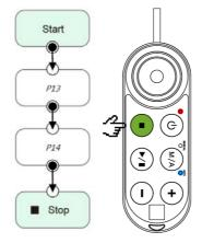
Figure 162: Stop Node Ends Project
