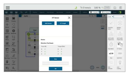
Figure 215: Read Values after Setting F/T Sensor
