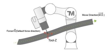
$\vec{X} := \overline{M.D.} \times \overline{Tool(Z)}$  (Tool(z) can't be parallel with  $\overline{M.D.}$ )  $\vec{Z} := \vec{X} \times \overline{M.D.}$  $\vec{Y} := \overline{M.D.}$
