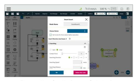
Figure 230: Linear Searching Parameter Setting Interface
