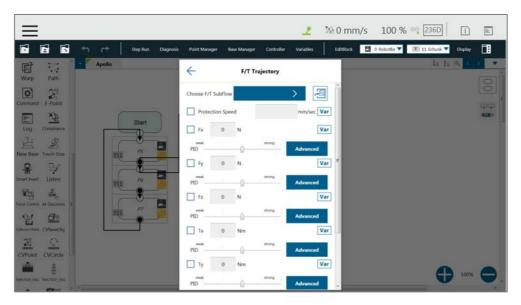
Figure 238: F/T Operation Modes – Trajectory (1/3)
