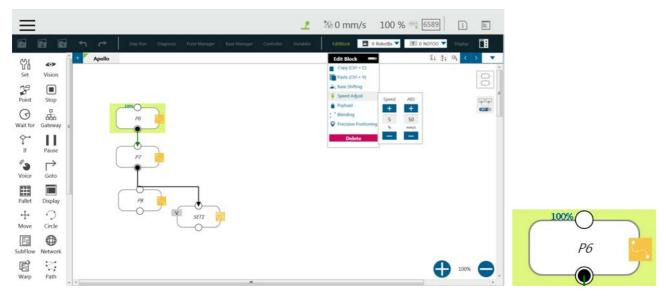
Figure 131: Speed Adjust and Speed Indication on the Node.
