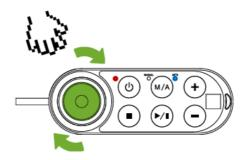
Figure 1: Release the Emergency Switch
