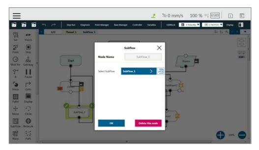
Figure 168: Select a subflow in the subflow node (1/2)
