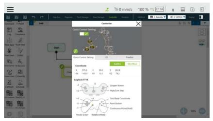
Figure 50: Controller (Quick Control Setting: JoyStick)
