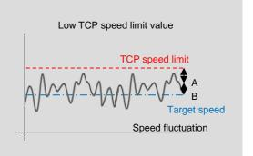
The custom values of the TCP speed and the Joint Speed are set in Setting>Safety>Performance Settings and Setting>Safety>Human-Machine Safety Settings>More Limit Setting for normal mode and collaborative mode, respectively.
