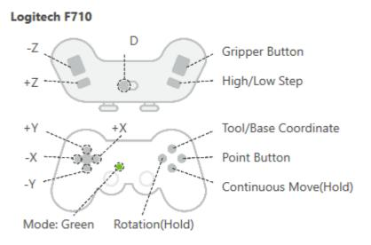
Figure 200: Joystick Functions
