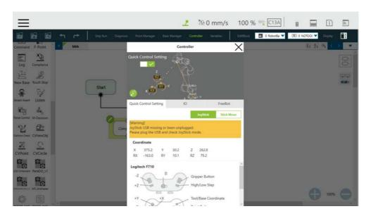
Figure 199: JoyStick without USB
