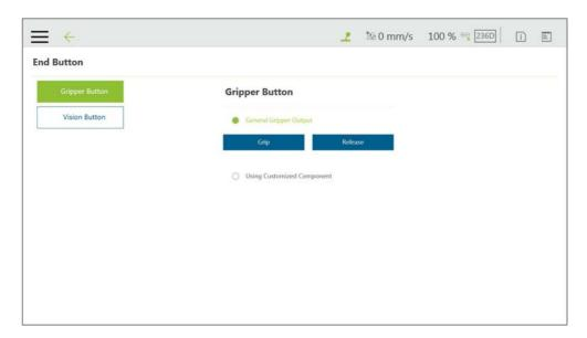
Figure 208: Gripper Button Setting Page
