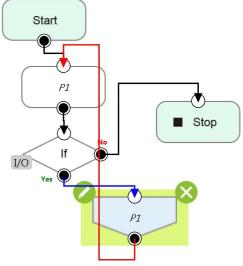
Figure 163: Goto Node Flow Transfer
