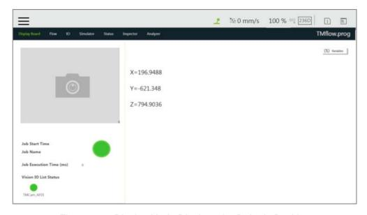
Figure 204: Display Node Displays the Robot's Position
