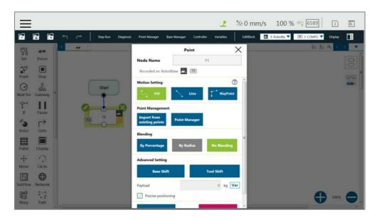
Figure 93: Shift Function of Point Node
