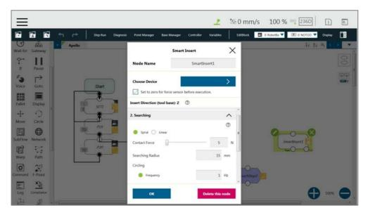
Figure 229: Spiral Searching Parameter Setting Interface
