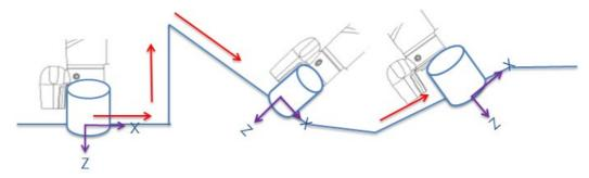
Figure 233: Tool Coordinate System
