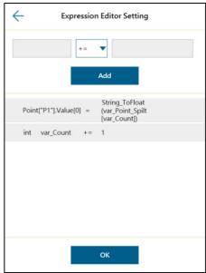
Figure 256: The Example of Point Parameterization Application (3/4)
