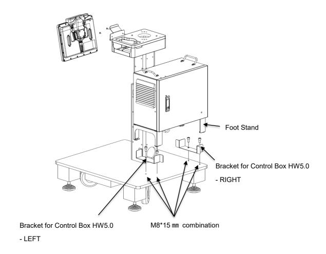
HW5.0 Robot Stick and its holder should be installed properly by the integrated applications or outside the safeguarded space based on the risk assessment. The distance of screw holes is 95 mm with M4\*5 mm screws
