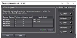
In the Belt object, a virtual encoder is needed for each part object (Part1 and Part2). Each virtual encoder will have an encoder association with the corresponding Belt object Encoder Channel of each controller, and the latch signal of the corresponding camera detecting that part object type as shown below in the figures below.
