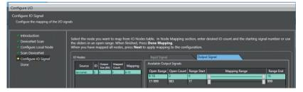
**17** Once all Input and Output are configured, click the **Next** Button to reboot the Controller and apply the updates to the I/O configuration. When the reboot finishes, click the **Finish** Button to close the *Configure IO* window.
