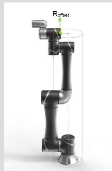
Figure 15: The Definition of R_{offset} .
