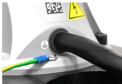
Figure 21: Securing the ground wire with the robot
