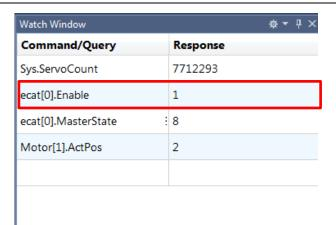
After making sure that correct communications are available, run the ECAT[0].Enable=0 command from the Terminal tab page to stop EtherCAT communications.
