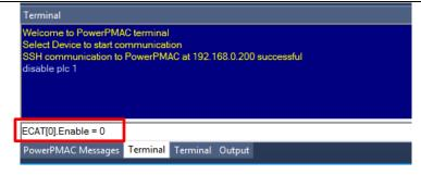
In the Terminal tab page or Watch Window, make sure that the ECAT[0].Enable value turns to 0.
