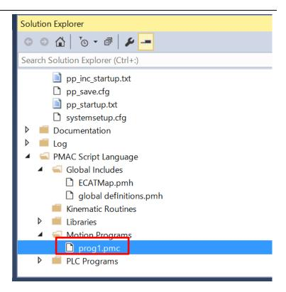
2 In the programming area of the prog1.pmc tab page, write a program as shown on the right.
