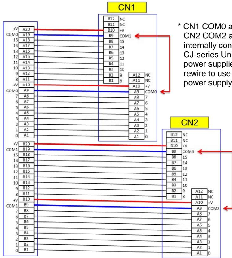
\* CN1 COM0 and COM1 and CN2 COM2 and COM3 are internally connected in the CJ-series Unit. When separate power supplies were used, rewire to use one common power supply.
