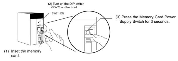
(4) Pressing the Memory Card Power Supply Switch for 3 seconds blinks the LED light (MCPWR) 1 time. The LED light blinks while the data is being transferred into the memory card. Once the data storage is completed, the LED light turns off.
