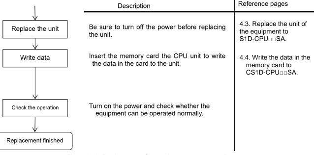
Figure 2-2: Replacement flow using a memory card
