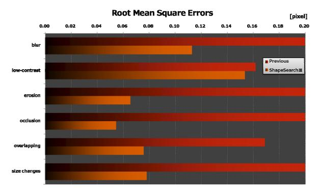
\* Input image size: VGA, Target: a cross pattern with translated by 0.1pix.
