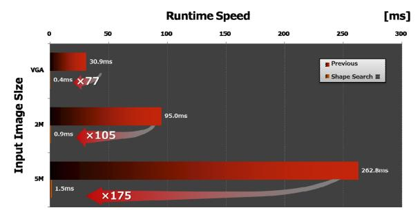
\* Target: a cross mark ("+"), Search area: whole image area, Rotation tolerance: +/- 10 degree Fig.3. runtime speed measurement results (on Intel Core<sup>TM</sup> i7 3770K)
