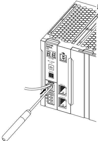
3. Pull out the flat blade screwdriver. Then, the cable is locked.
