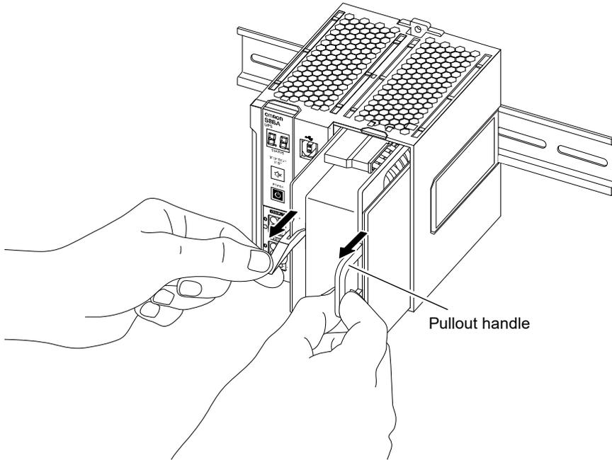
6. Arrange a new battery pack for replacement. Make sure that the new battery is connected to the connector of the battery board in place.
