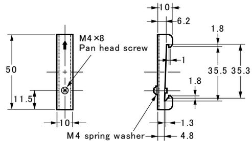
Note 1: If the DIN rail is subjected to vibration or shocks, scrap metal can be produced because of aluminum abrasion. In such a case, use a steel DIN rail instead.
