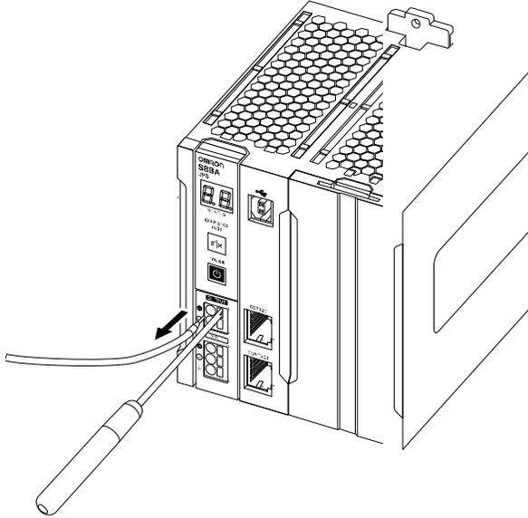
2. Pull out the flat blade screwdriver.
