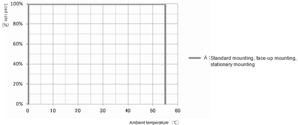
● Derating curve (Use as a UL compliant device)
