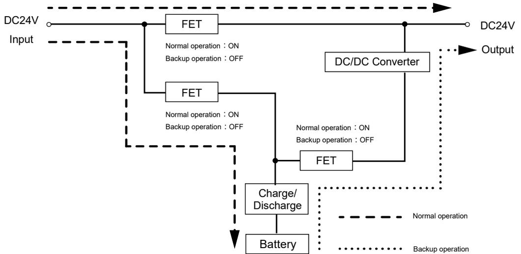
\*In normal operation, 24 VDC is output as-is for charging the battery and from the input power supply.
