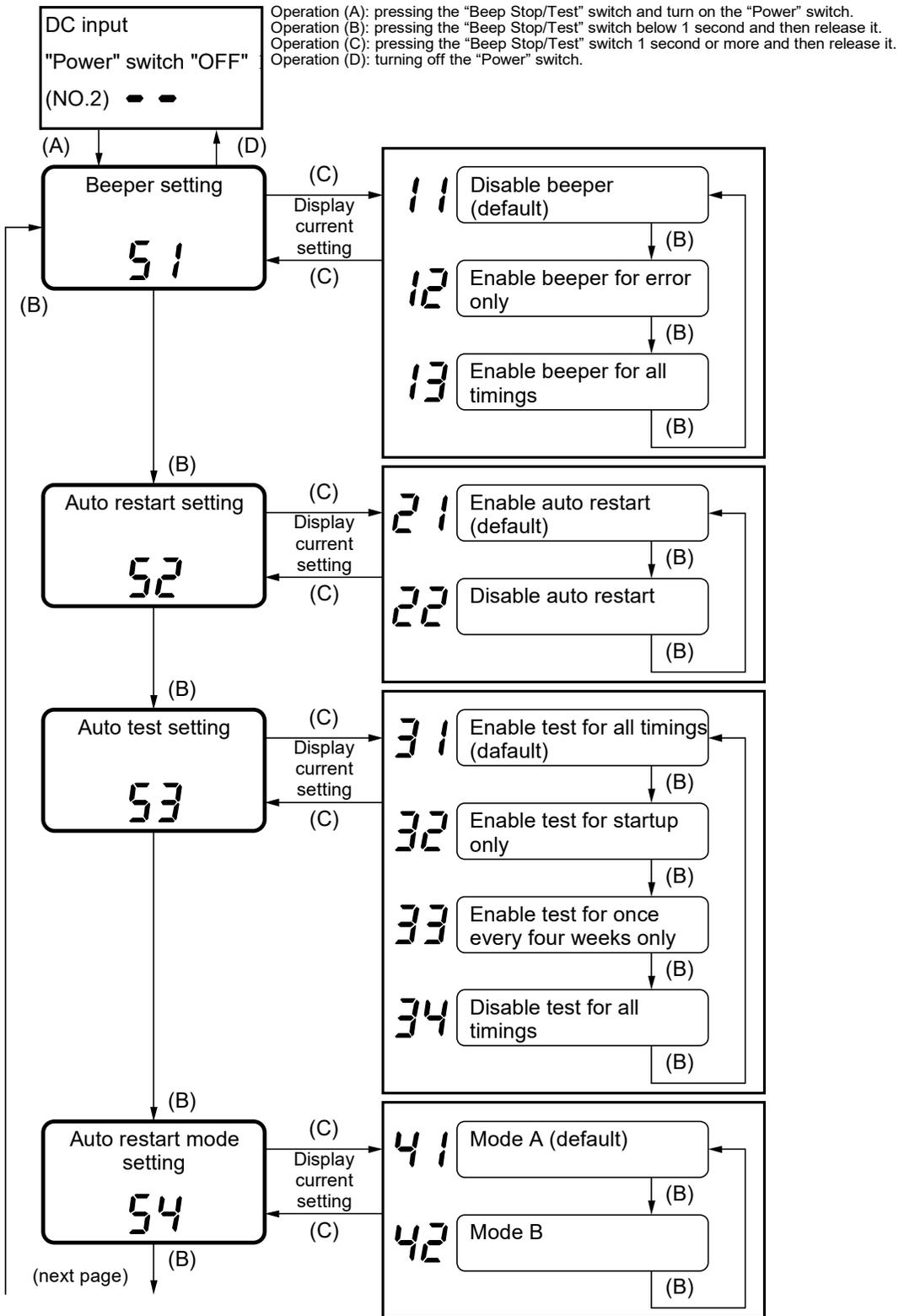
Operation (A): pressing the "Beep Stop/Test" switch and turn on the "Power" switch.
