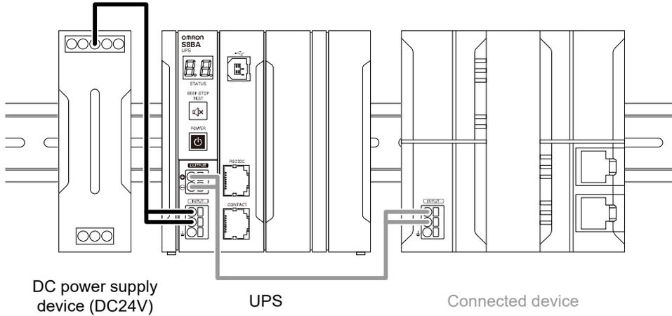
2. Connect the input cable to the DC power supply device.
