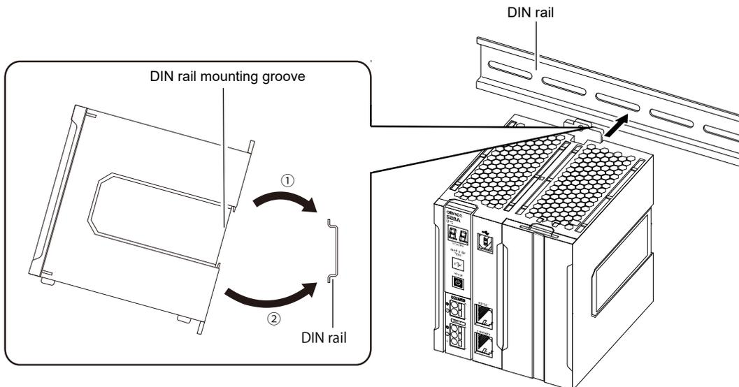
**3.** Close the "DIN rail mounting hooks" in the back of the UPS.
