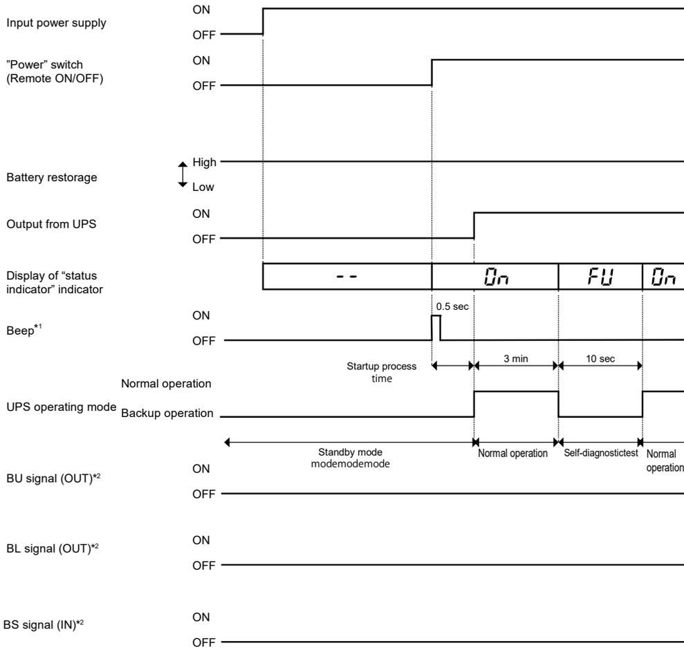
\*1 "Disable beeper" is set by factory default. Even when "Disable beeper" is set, the buzzer sounds at startup. For details, see "4-4 UPS operation mode settings".
