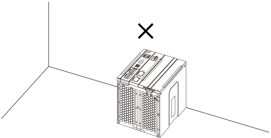
⊘ To mount UPS on floor with its top away from you, ensure that its top is not in contact with wall.
