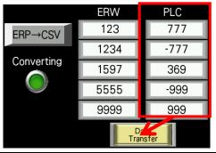
8. Press the "Data transfer" button to copy the PLC addresses into the ERW area. and then press the [ERP->CSV] button.
