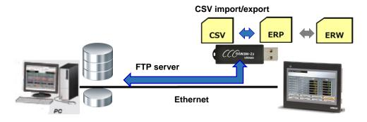
As an example, the following procedure shows how to transfer the CSV file onto PC, process, and overwrite it back to the external memory again. Perform this procedure after copying the data in the ERW area into the CSV file in the external memory as shown in the step 9 of Section 4-1-5 Operating the Sample Screens
