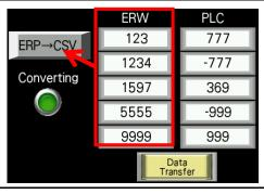
The data will be output to the CSV file. As shown on the right, consecutive PLC address areas and NB internal addresses can be output in the CSV format.
