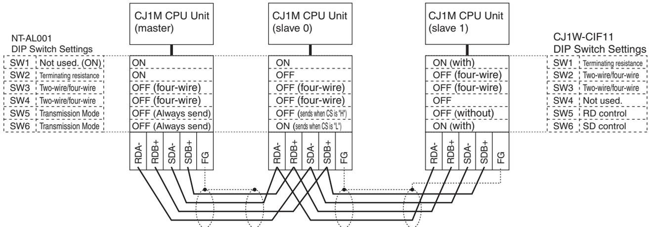
**Wiring for Two-wire Cable**
