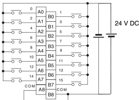
The polarity can be connected in either direction.
