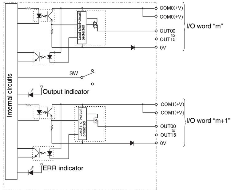
When the output current of any output exceeds the detection current, the output for that point will turn OFF. At the same time, the ERR indicator will light and the corresponding flag (one for each common) in the Basic I/O Unit Information Area (A050 to A069) will turn ON.
