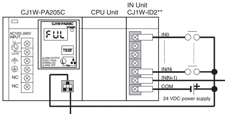
External Display Device Connection Example
