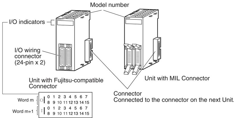
**64-point Units (2 x 40-pin Fujitsu-compatible Connectors or 2 x 40-pin MIL Connectors)**
