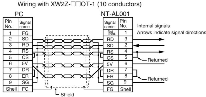
2. When the NT-AL001 Link Adapter is connected to the RS-232C port on the CPU Unit, 5 V is supplied from pin 6, eliminating the need for a 5-V power supply.
