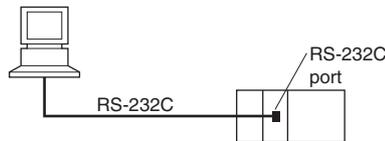
**Note** The maximum cable length for an RS-232C connection is 15 m. RS-232C communications specifications, however, do not cover transmissions at 19.2 Kbps. Refer to documentation of the device being connected when using this baud rate.
