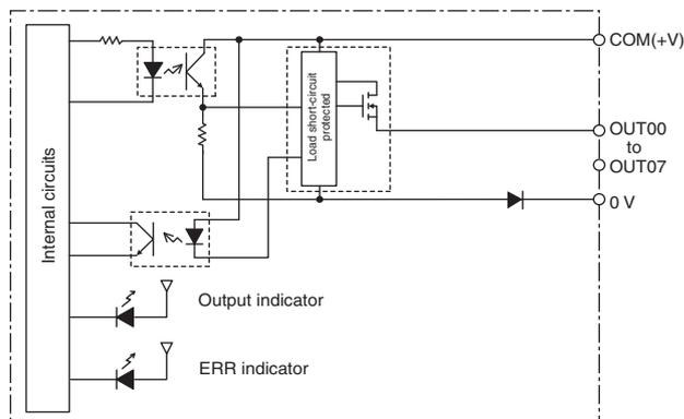
When overcurrent is detected, the ERR indicator will light, and the corresponding flag in the Basic I/O Unit Information Area will turn ON.
