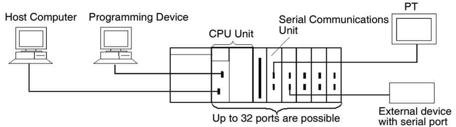
**Standard Serial Communications with External Devices**
