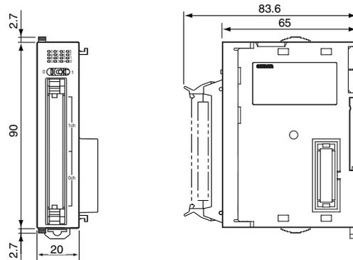
24-V DC Input/Transistor Output Units
