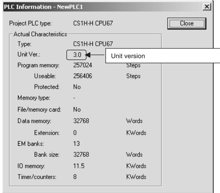
Use the above display to confirm the unit version of the CPU Unit.
