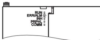
When the ERR/ALM indicator flashes, connect a Programming Console to the peripheral port and read the error message. If the message “BATT LOW” appears on the Programming Console\* and the Battery Error Flag (A40204) is ON\*, first check whether the battery is properly connected to the CPU Unit. If the battery is properly connected, replace the battery as soon as possible.
