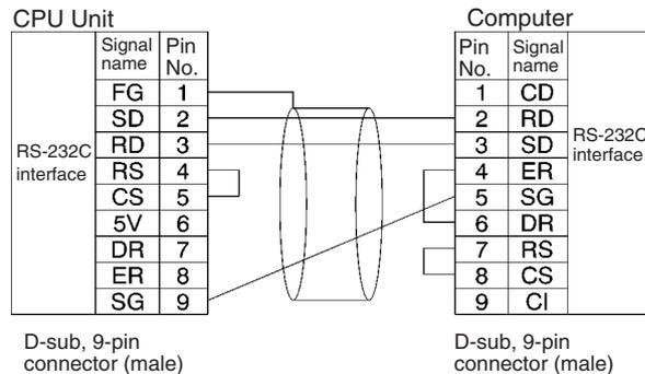
Although this wiring is different from that shown in the example above, it can be used to increase noise immunity if required.
