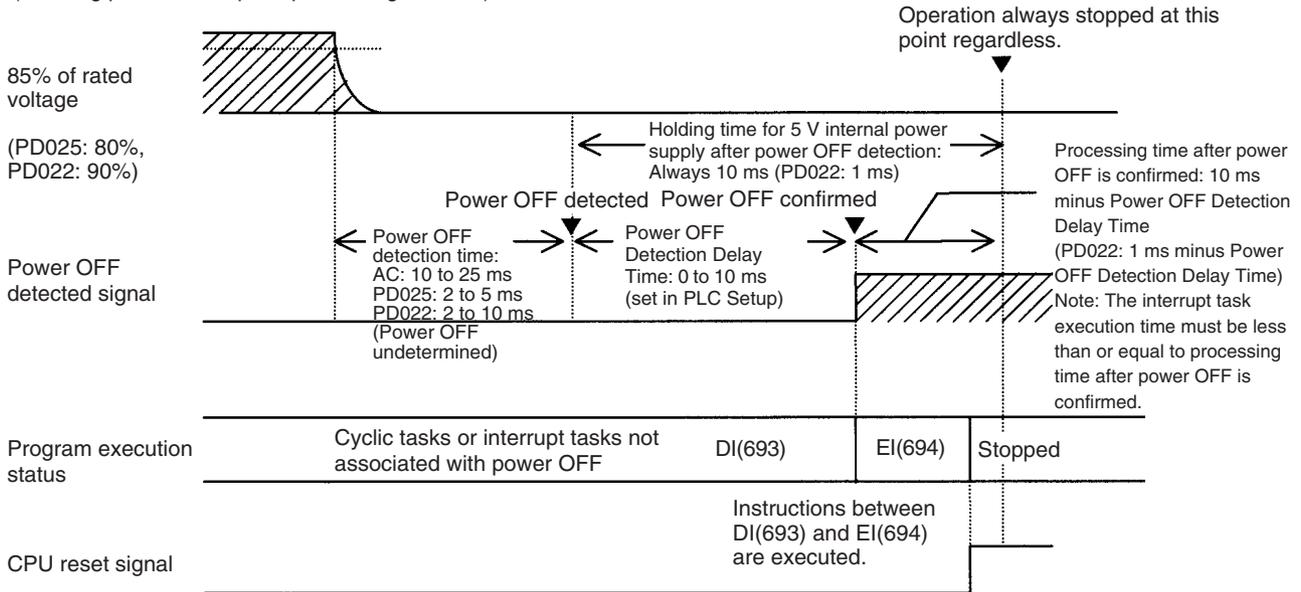
Interrupt processing is performed according to the contents of A530 and the PLC Setup as shown below.
