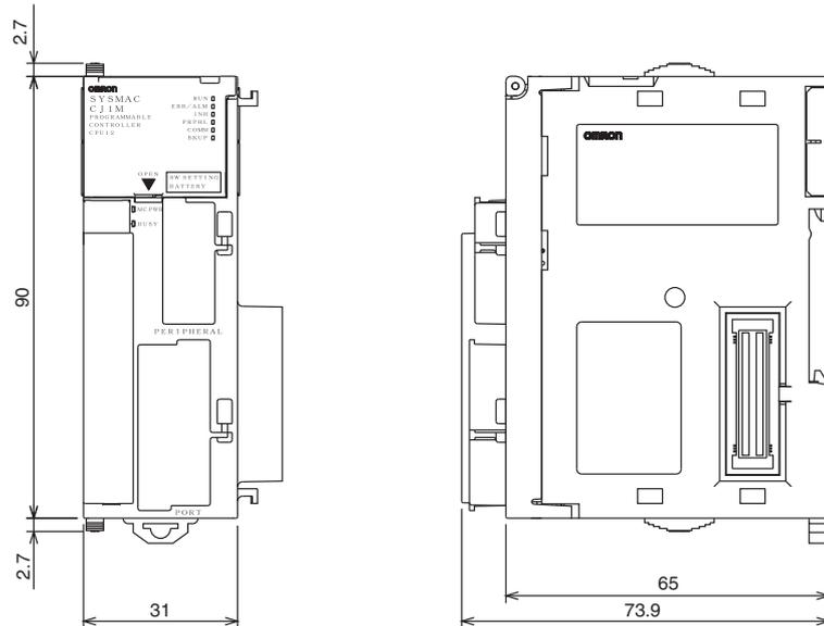
CPU Units with Built-in I/O (CJ1M-CPU2□)
