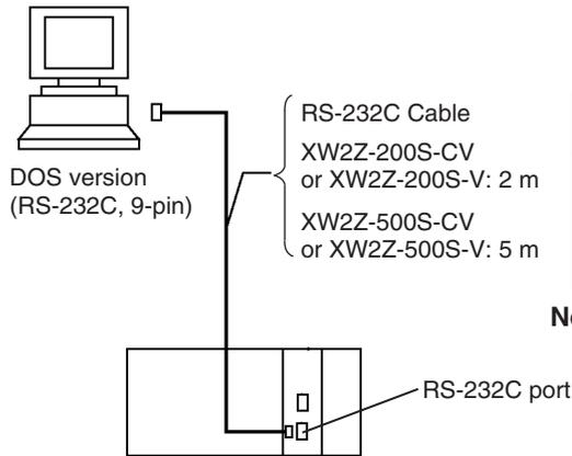
Connecting Cables for RS-232C Port
