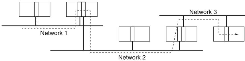
Seamless message communications are possible across Ethernet, Controller Link, and DeviceNet networks, enabling easy information integration on machine, machine-to-machine, and machine-to-host levels.
