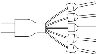
With four-wire cables, insert two signal lines into each crimp terminal together before crimping.
