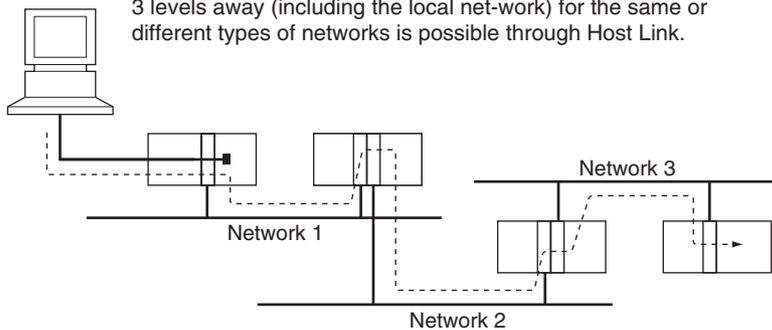
Message transfer between PLCs on a network 3 levels away (including the local network) for the same or different types of networks.
