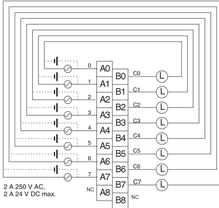
Polarity of the DC power supply can be connected in either direction because relay contacts are used.
