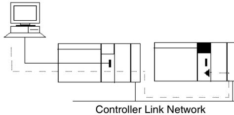
Remote programming/monitoring of a PLC on a network up to 3 levels away (including the local network) for the same or different types of networks is possible through Host Link.
