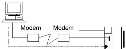
Remote programming/monitoring of a PLC on the network through Host Link
