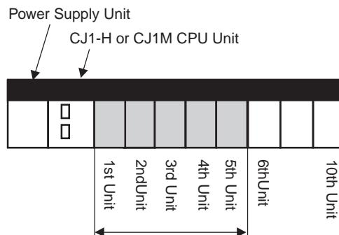
For CJ1-H CPU Units: External interrupt tasks can be activated only from these Units.
