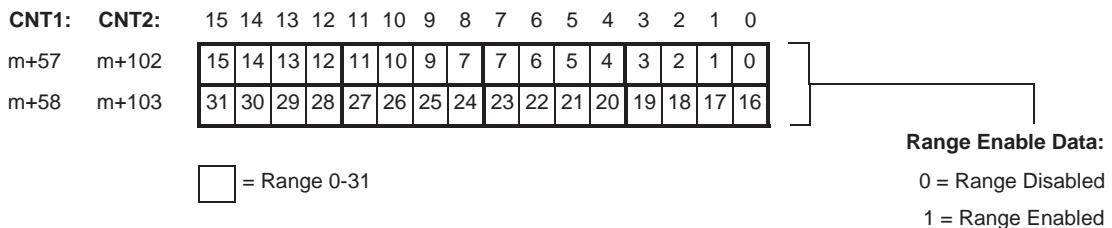
**Note** Enabling/Disabling of Ranges can also be done on the fly by using IOWR-instructions. Refer to 4-3 "IOWR-Instruction" for more details.
