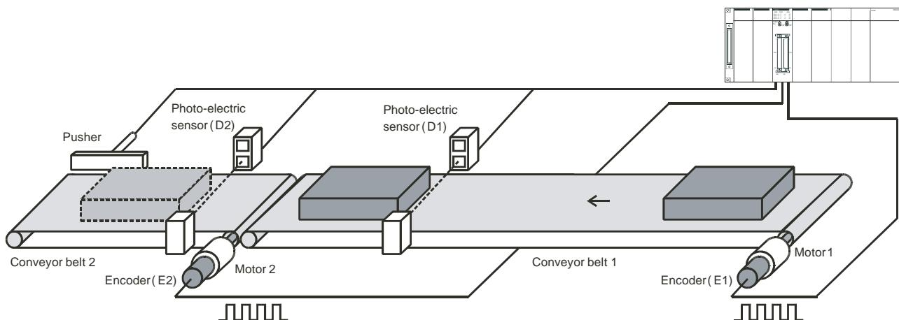
To measure the length of objects the pulses of encoder E1 are counted by Linear/Circular Counter 1 (corresponding DIP switch on the front of the Unit is in the ON-position). Photo-electric sensor D1 is connected to Digital Input I0. Digital Input I0 controls Counter 1 and is assigned Digital Input Function 11 (Reset, Stop, Capture and Continue).
