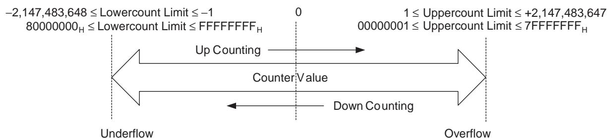
If the Counter Value goes above the Upper Count Limit or below the Lower Count Limit an Overflow- and Underflow flag will be set respectively. These are reported in CIO for the corresponding Counter.
