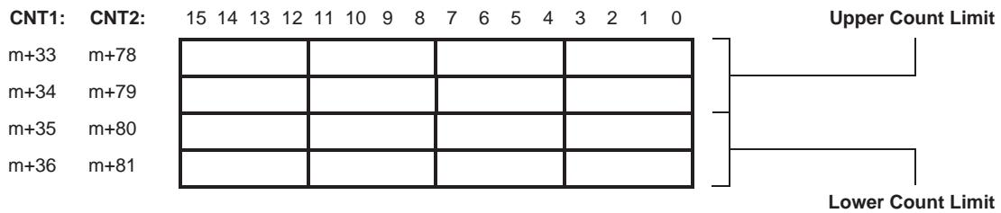
Set Upper Count Limit for Linear Counters between  $00000001_H$  and  $7FFFFFFF_H$ . By default ( $=00000000_H$ ) the Upper Count Limit is equal to  $7FFFFFFF_H$ . Set Lower Count Limit for Linear Counters between  $80000000_H$  and  $FFFFFFF_H$ . By default ( $=00000000$ ) the Lower Count Limit is equal to  $80000000_H$ .
