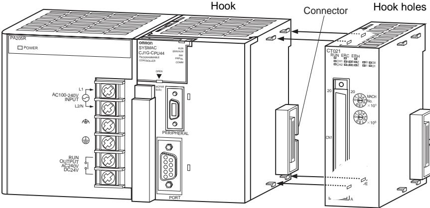
2. Slide the yellow sliders on the top and bottom of the Units until they click into place, firmly locking the Units together.
