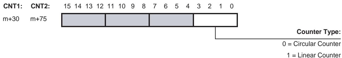
For Circular and Linear Counters all the functions and features of the High-speed Counter Unit are available and configurable. For Simple Counters only the default functions and features are supported since the Unit ignores the DM-settings for Simple Counters.
