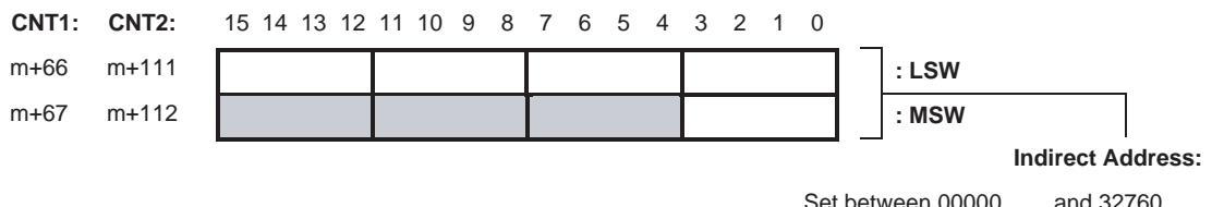
The least significant word (LSW) of the Indirect Address contains the four least significant digits and the most significant word (MSW) contains the most significant digit of the Indirect Address (refer to the examples on the following pages).
