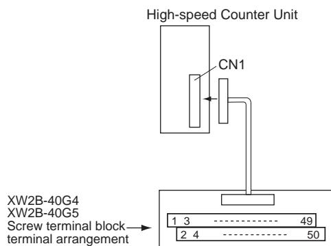
**Note** The top row of the Terminal Block Unit (numbered 1 to 39) corresponds to the pins numbered A1 to A20 of the associated connector (CN1) on the High-speed Counter Unit. The bottom row of the Terminal Block Unit (numbered 2 to 40) corre-
