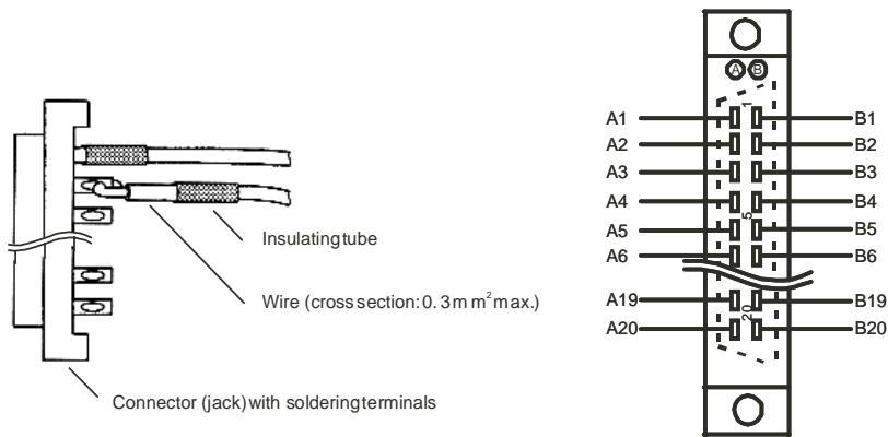
Numbering of the soldering terminals on connector (jack).
