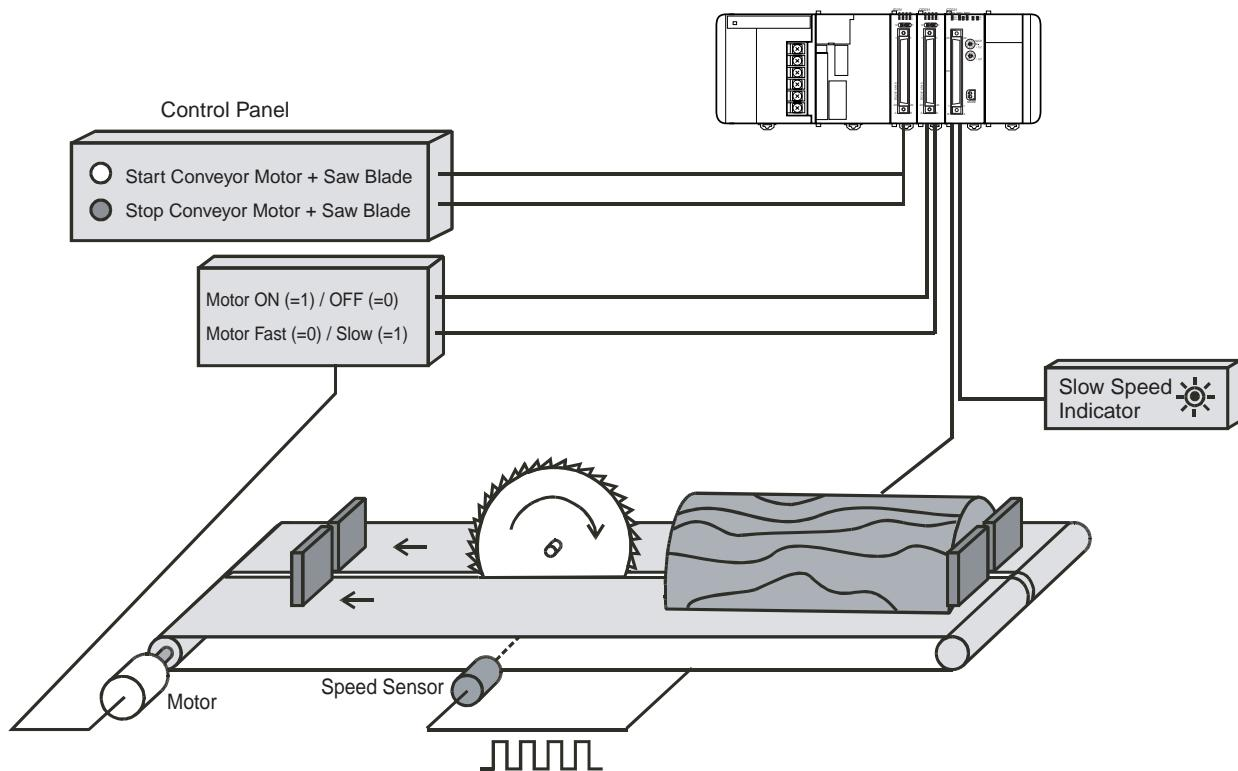
The speed sensor is connected to Circular Counter 1. The two Rate Ranges (Range 0 and 1) of Counter 1 are used to detect the speed of the saw blade. Turning the conveyor motor and the saw blade ON/OFF, using the control panel, is controlled via the PLC ladder program and a Digital Input- and Output Unit (e.g. CJ1W-OD231/ID231). The speed of the conveyor motor is controlled by Digital
