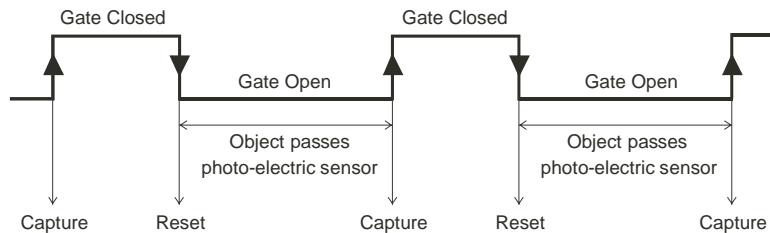
At the falling edge of Digital Input I0, when an object enters the beam of the photo-electric sensor, the Counter Value is reset, the gate is opened and Counter 1 starts counting pulses from zero. At the rising edge of Digital Input I0, when the object leaves the beam of the photo-electric sensor, the Counter Value of Counter 1 is captured and the gate is closed.
