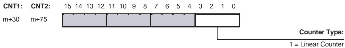
A Linear Counter has the full counting range (=32 bits) available to count up- or downwards over the positive and negative counting range between the Minimum Count Limit and the Maximum Count Limit. By default the Minimum and Maximum Count Limits are set to the maximum counting limits (i.e. -2,147,483,648 and +2,147,483,647 respectively).
