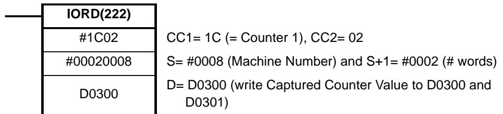
**Note** Reading the Captured Counter Value with IORD is also supported for Simple Counters (refer to 3-2-1 "Simple Counter").
