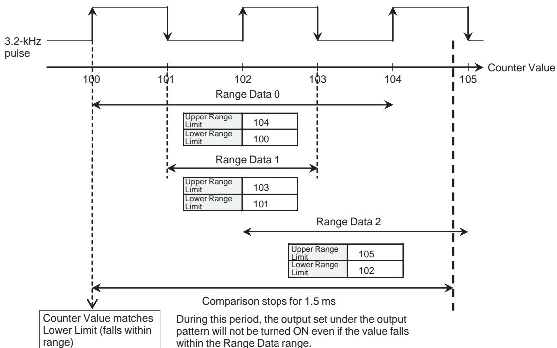
During this period, the output set under the output pattern will not be turned ON even if the value falls within the Range Data range.
