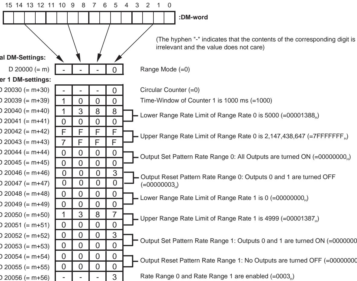
Transfer the DM-settings to the High-speed Counter Unit by restarting the Unit.
