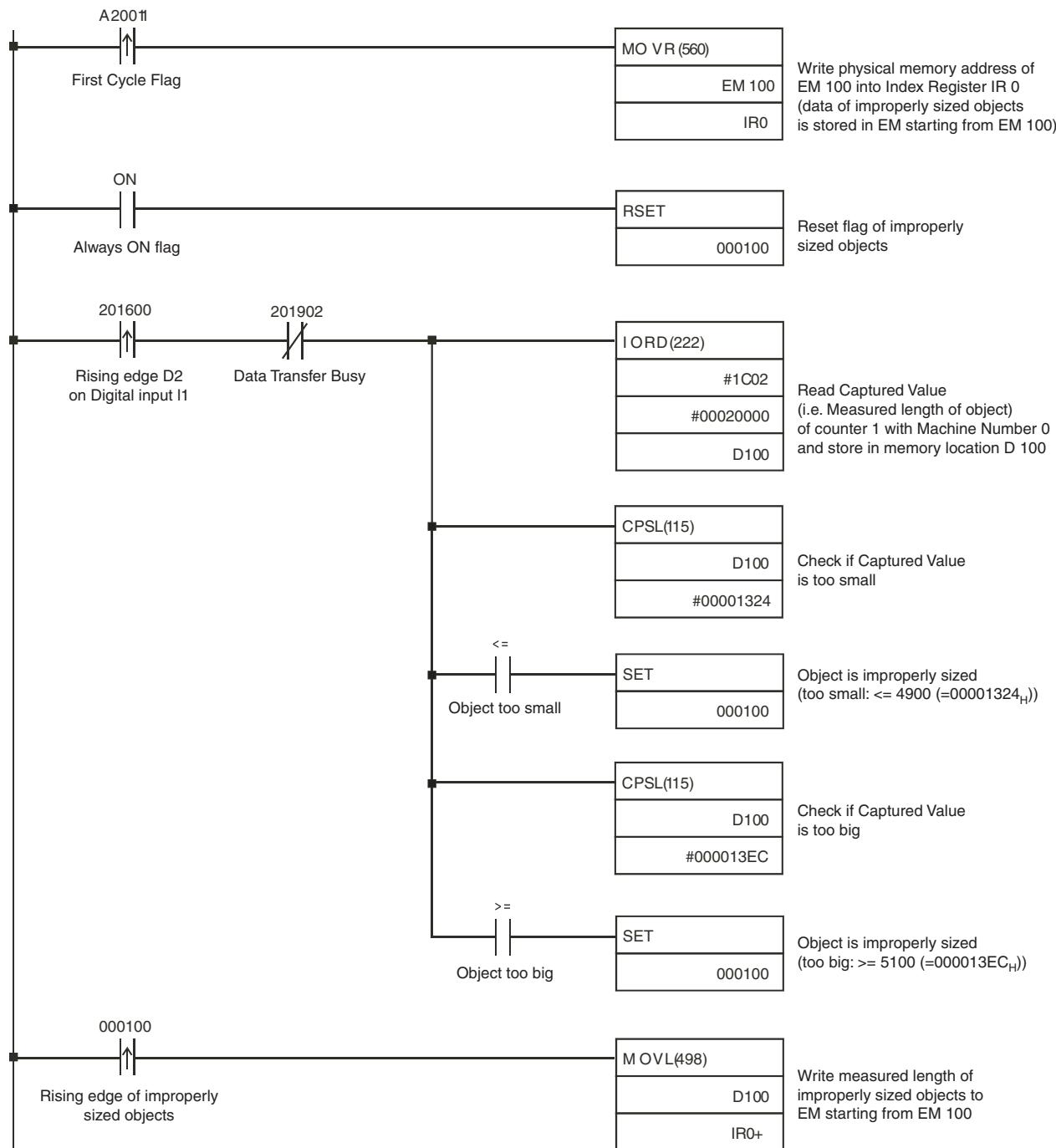
**Note** If the digital input I1 is set while the Data Transfer Busy is ON, the IORD-instruction may not be executed depending on timing. Therefore, please consider adding a self-holding circuit.
