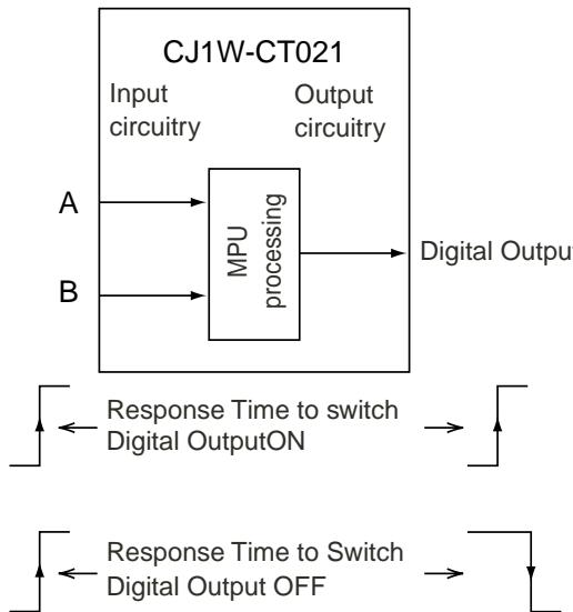
The Response Time can vary between 0.1 and 0.5 milliseconds, but is guaranteed to be less than 0.5 milliseconds. The following factor causes the Response Time to fluctuate:
