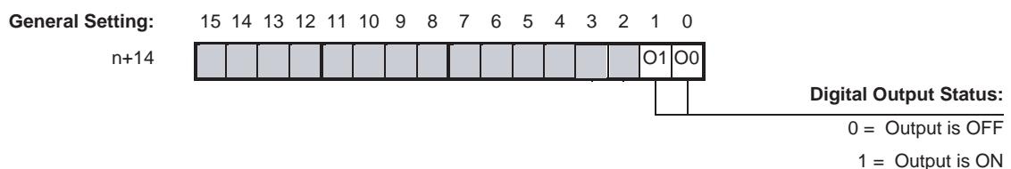
Bits 0 and 1 correspond to the Physical Digital Outputs O0 and O1.
