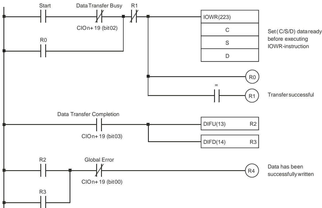
Please do not execute the IOWR-instruction when the Data Transfer Busy is ON. If an error occurs during the execution of the IOWR-instruction the ER-flag turns ON. The Data Transfer Completion bit (CIO n+19, bit 03) is toggled every time that data transfer is completed. The Global Error bit (CIO n+19, bit 00) turns ON when the Unit detects any error that causes this bit to be set (refer to 5-2 "Error codes").
