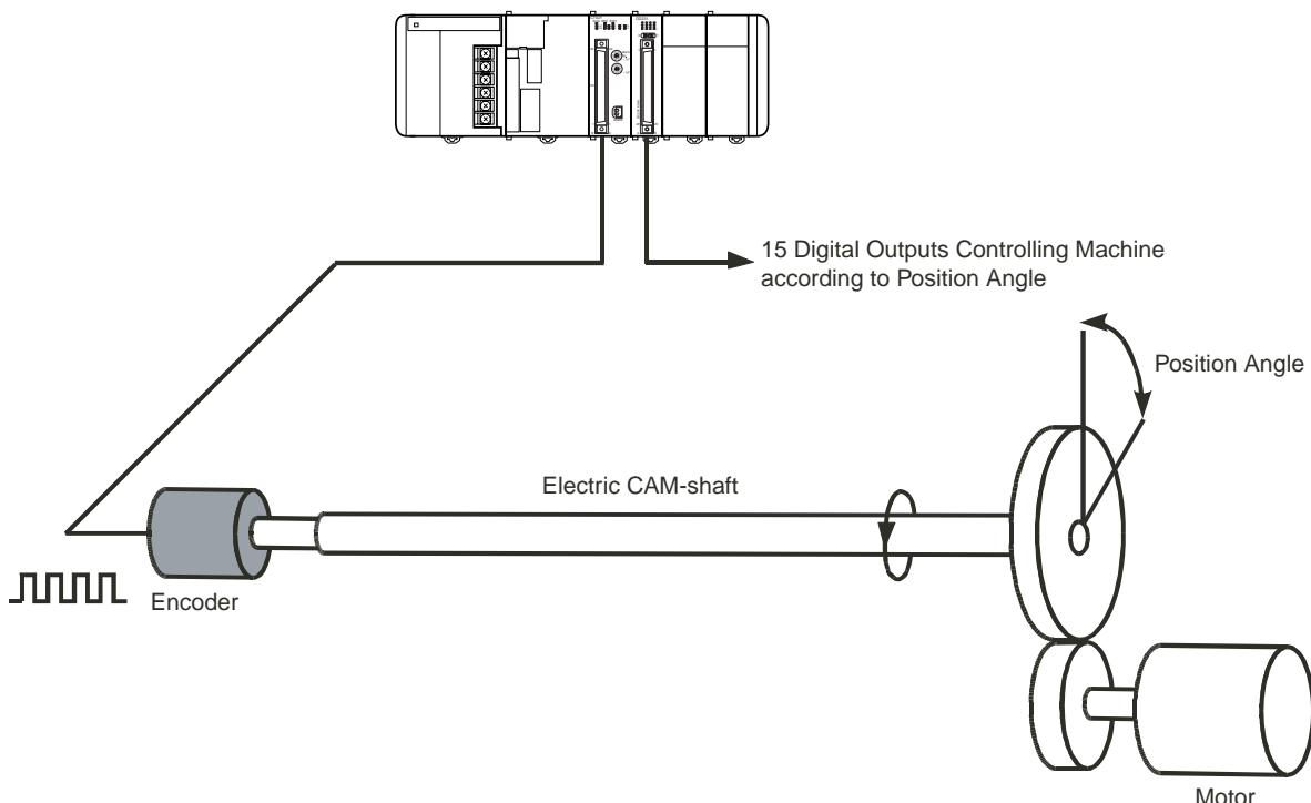
The encoder is connected to Circular Counter 1. The 15 outputs are controlled by 5 Ranges (Range 0 to 4). An Hysteresis of 20 counts is defined and will be applied to the Range Limits. The outputs are assigned to the Interrupt Tasks 10 to 39 respectively in the PLC ladder program (i.e. offset is 10). As a result the rising edge of (Digital) Output O0 is assigned to External Interrupt Task 10, the falling edge to External Interrupt Task 11 and so on.
