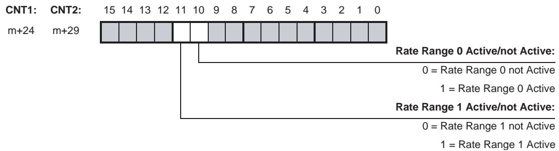
**Note** Rate Ranges may not overlap. If Rate Ranges overlap the Unit will generate an error (refer to 5-2 "Error codes" for more details).
