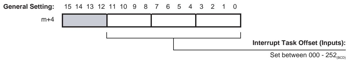
Since there are 256 External Interrupt Tasks available (numbered 0 to 255), the Offset can be maximum 252.
