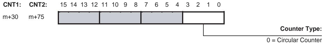
A Circular Counter has 32-bits (the full counting range) available to count up- or downwards over the positive counting range between 0 and the Upper Count Limit.
