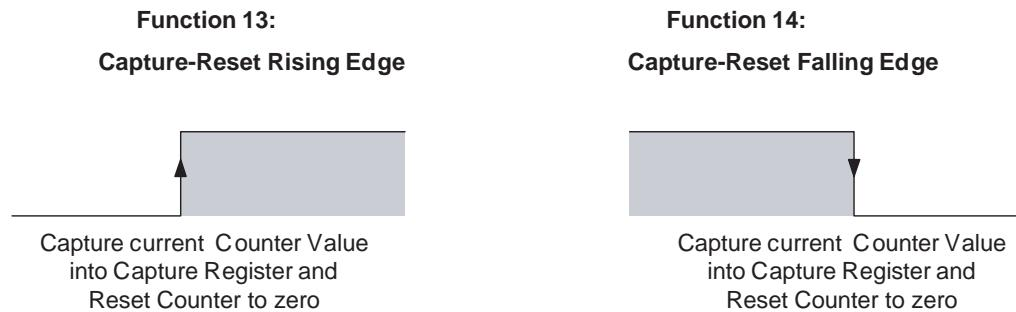
To reset a Counter with Function 13 or 14, the Software Enable Reset Bit must be set to 1. Refer to 3-6 "Reset Signals" for detailed information about resetting Counters.
