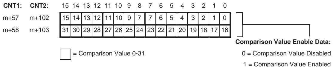
**Note** Enabling/Disabling of CV's can also be done on the fly by using IOWR-instructions. Refer to 4-3 "*IOWR-Instruction*" for more details.
