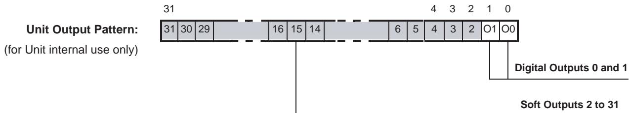
Digital Outputs 0 and 1 correspond with the Physical Digital Outputs O0 and O1.
