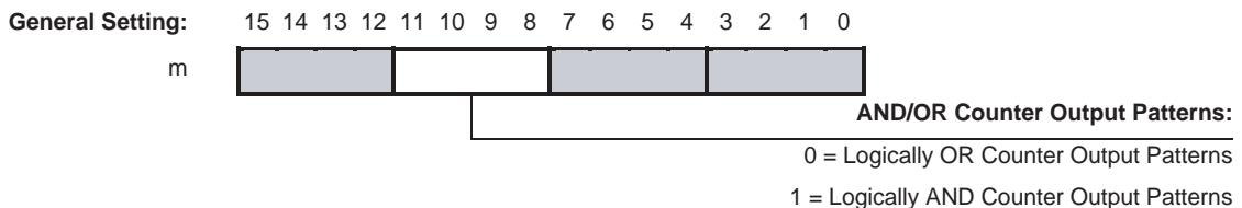
**Note** The Counter Output Patterns of Counters which are configured to use no (i.e. zero) Ranges, are ignored in the AND-calculation of the Unit Output Pattern. Like this, Counters that you do not want to use, do not influence the AND-calculation of the Unit Output Pattern. If both the Counters are configured to use no Ranges, the output patterns for both outputs will be all OFF.
