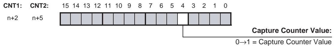
If you want to use the Captured Value in your Ladder Program, you must use the IORD-instruction. This instruction reads the Captured Value from the Unit into a specified location in the memory of the PLC. For more details on using the IORD-instruction and reading the Captured Value refer to 4-4 "IORD-Instruction".
