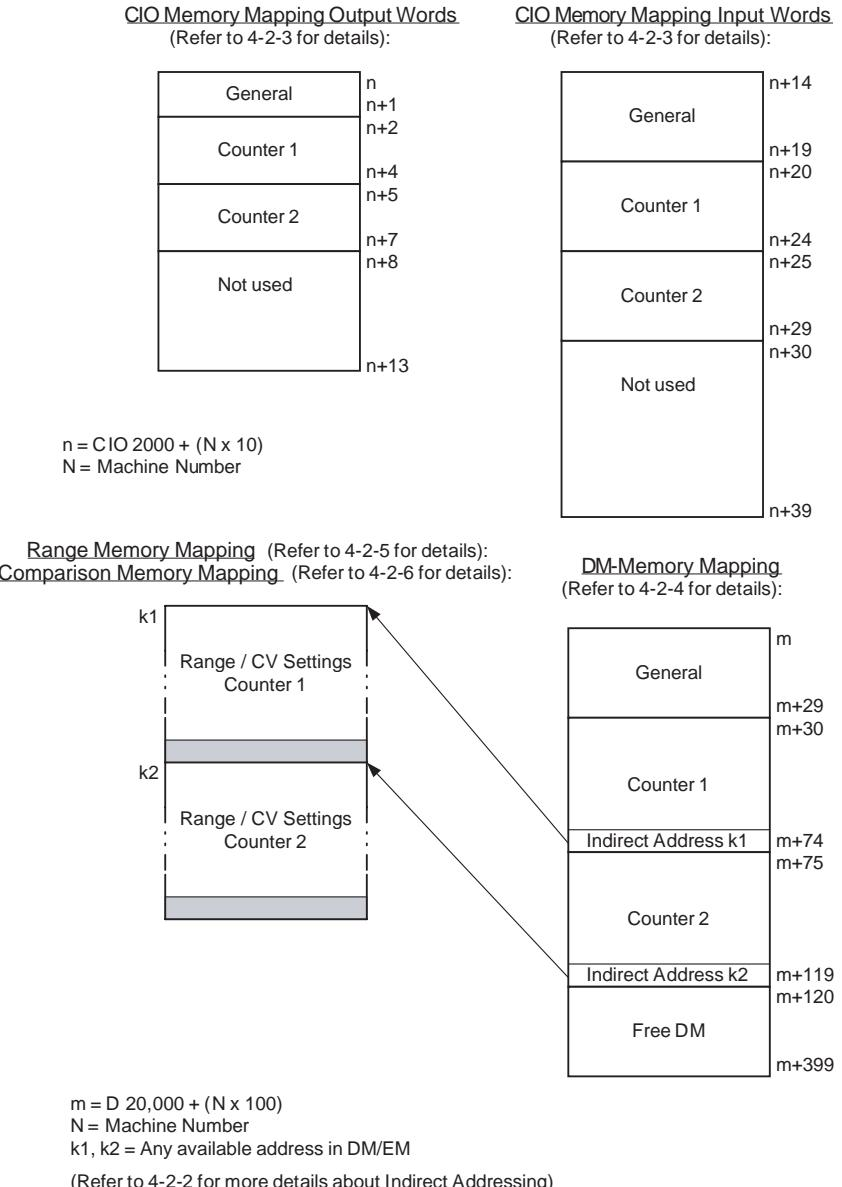
**Note** The Range/Comparison Data blocks that are allocated to the Counters do not necessarily have to be consecutive and can be in any area of DM/EM. In case they overlap the Unit reports this in CIO as a warning, but does not generate an error. This makes it possible to define only one block with Range/Comparison
