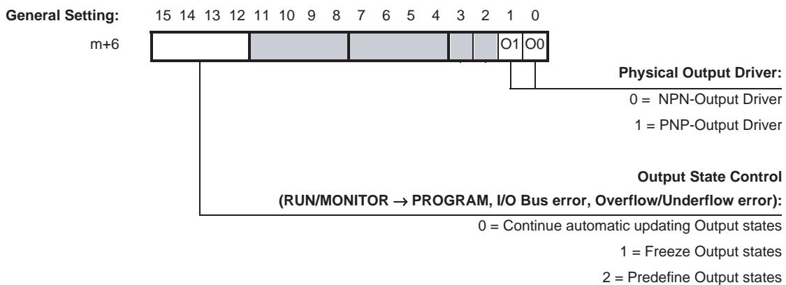
Bits 0 and 1 correspond to the Physical Digital Outputs O0 and O1.
