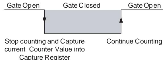
**Note** The Open Gate Bit, Close Gate Bit, Preset Counter Bit, Reset Bit, or the Counter Capture Bit in CIO may not be executed if turned ON for only one PLC cycle. Always keep these bits turned ON until the execution status changes for the corresponding flags in n+24 or n+29.
