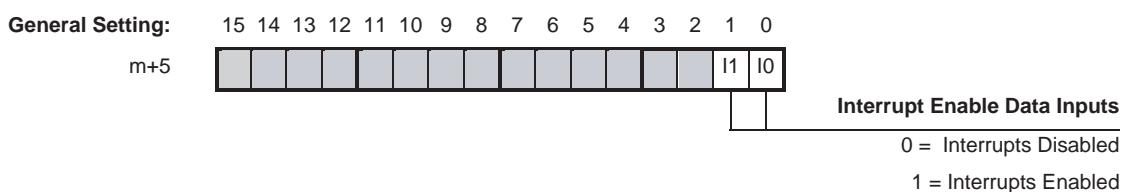
Bits 0 and 1 correspond with the Physical Digital Inputs I0 and I1.
