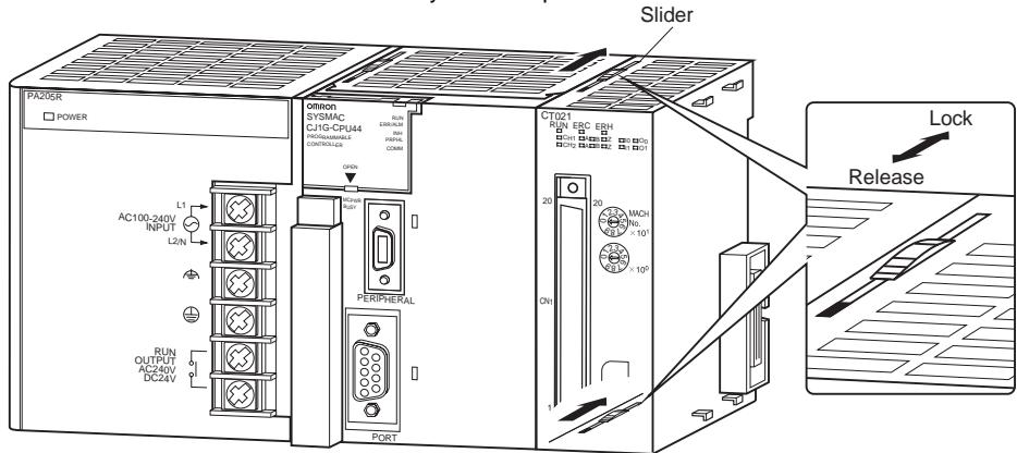
3. Attach an End Plate to the Unit on the right end of the Rack.
