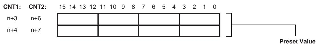
Set between 00000000<sub>H</sub> and FFFFFFFF<sub>H</sub> (Circular Counter)
