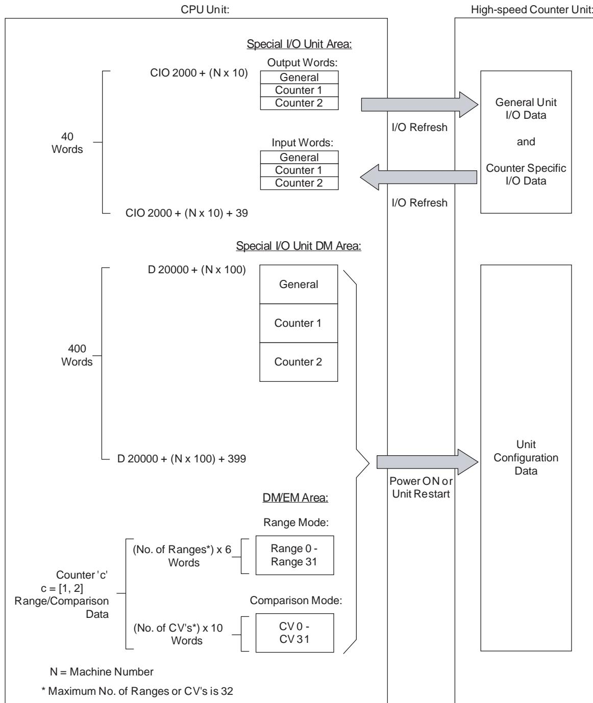
**Special I/O Unit Area and Special I/O Unit DM Area**
