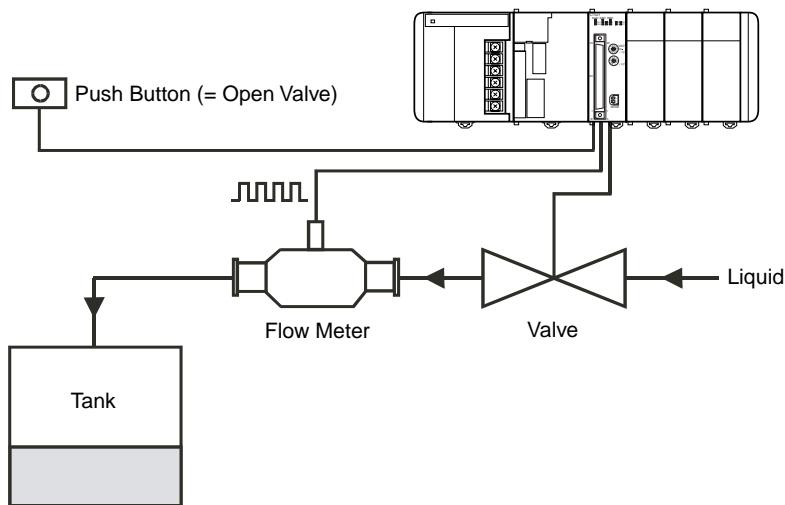
The push button is connected to Digital Input I0 and the valve is connected to Digital Output O0 of the High-speed Counter Unit. The pulses of the flow meter are counted by Counter 1 which is configured as Simple Counter (corresponding DIP switch at the front of the Unit is in the OFF-position).
