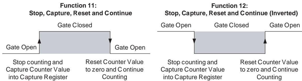
To reset a Counter with Function 11 or 12, the Software Enable Reset Bit must be set to 1. Refer to 3-6 "Reset Signals" for detailed information about resetting Counters.
