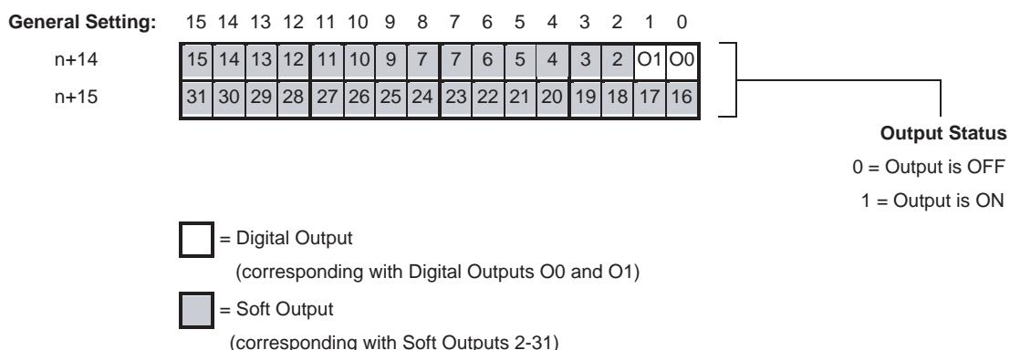
**Note** Every Soft and Digital Output can be configured to generate an Interrupt to the CPU. For details refer to 4-6-1 "Outputs Generating Interrupts".
