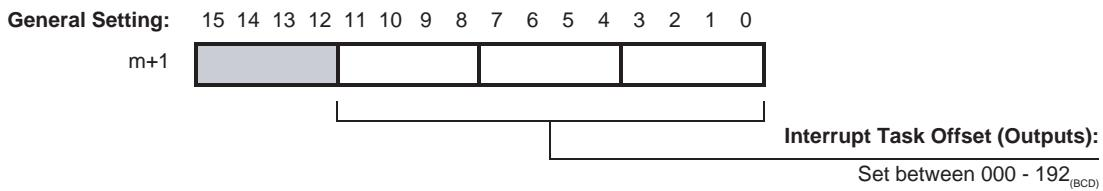
Since there are 256 External Interrupt Tasks available (numbered 0 to 255) the Offset can be maximum 192. With an Offset of 192 the last Output (31) will be assigned the last available External Interrupt Task 255 (=192+2x31+1).
