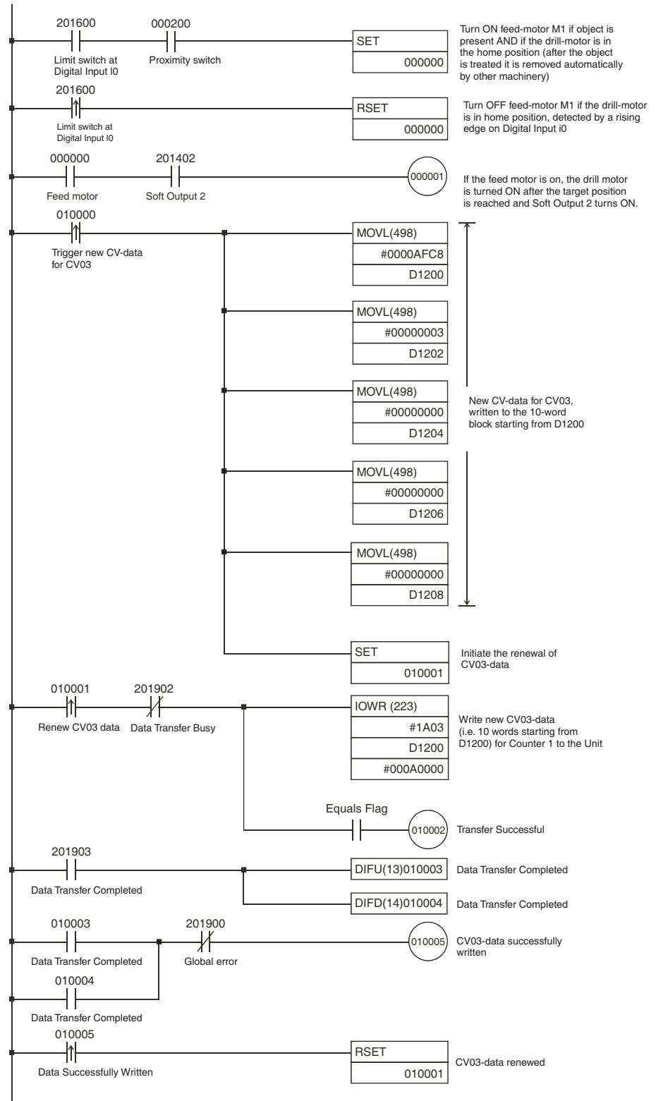
**Note** If CV03 data is renewed while the Data Transfer Busy is ON, the IOWR-instruction may not be executed depending on timing. Therefore, please consider adding a self-holding circuit.
