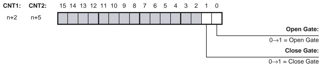
A rising edge of the "Open Gate Bit" opens the Gate regardless of the state of the "Close Gate Bit". A rising edge of the "Close Gate Bit" closes the Gate regardless of the state of the "Open Gate Bit". At a simultaneous rising edge of both bits, the state of the Gate is unchanged.
