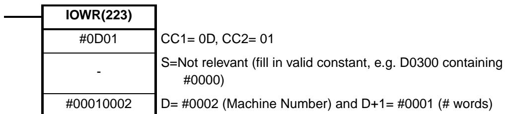
1. The configuration settings can also be transferred to the Unit by Powering Up the CJ-series PLC system or by restarting the Unit.
