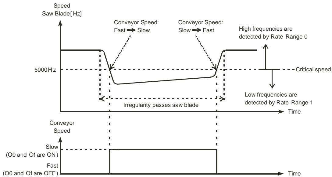
In order to use Counter 1 for Rate Measurement its Time-Window has been set to 1 second (=1000 ms). Rate Range 0 is used to detect frequencies that are above the critical speed and Rate Range 1 used to detect frequencies that are below the critical speed:
