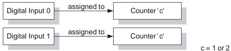
**Note** Every Digital Input can be configured to generate an Interrupt to the CPU. For details refer to 4-6-2 "Digital Inputs Generating Interrupts".
