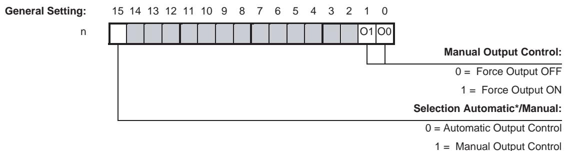
Bits 0 and 1 correspond to the Physical Digital Outputs O0 and O1.
