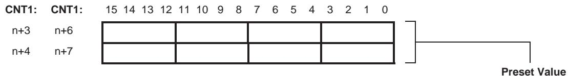
**Resetting a Simple Counter** For every Simple Counter the Software Reset Bit can be used to trigger a Reset. A rising edge of the Software Reset Bit triggers a Reset in the next I/O Refresh Cycle.
