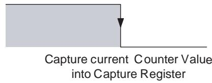
The Counter Value can also be captured by using the "Capture Counter Value Bit" in CIO.
