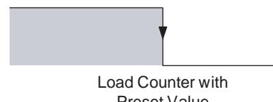
The Unit is equipped with a Preset Register for every Counter that contains the Preset Value. To change the Preset Value you can change the (32-bits) Preset Value in CIO of the corresponding Counter. The Counter Value is overwritten with
