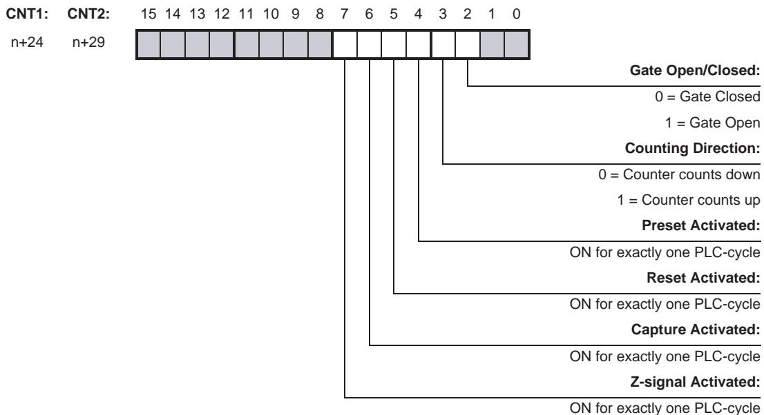
The Reset, Preset, Capture and Z-signal Activated Bits are ON for exactly one PLC-cycle after the occurrence of a (short) pulse which was detected since the previous I/O Refresh.
