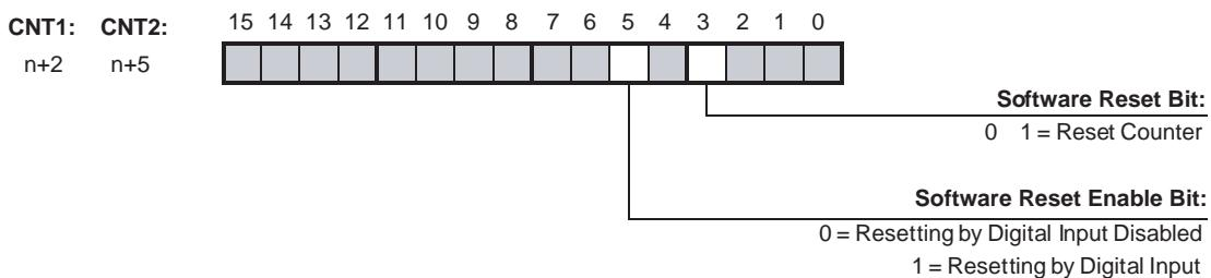
**Note** Resets from an External Control Input signal will be executed within 300 μs.
