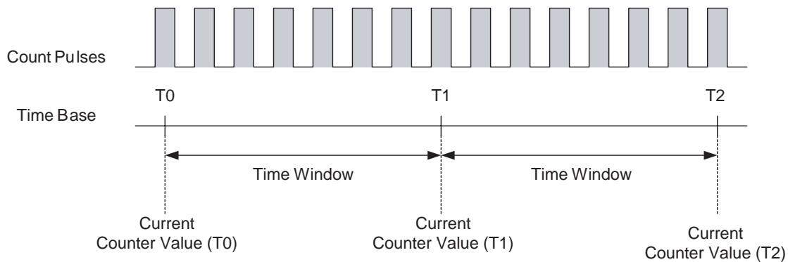
$$\text{Rate Value 1} = \text{CCV}(\text{T1}) - \text{CCV}(\text{T0})$$
