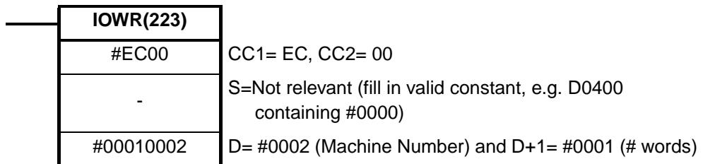
**Note** Writing the Error Clear Command with IOWR is also supported for Simple Counters (refer to 3-2-1 "Simple Counter"). This enables you to clear IORD/IOWR-instruction errors that occurred after you have issued the IORD-instruction "Captured Counter Value" or the IORD/IOWR-instruction "Counter Value" to a Simple Counter.
