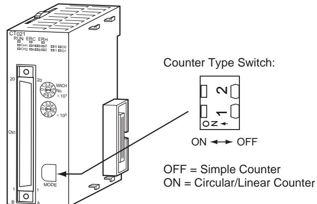
2. Set the Machine Number. Refer to 2-1-4 "Machine Number Switch" for further details.
