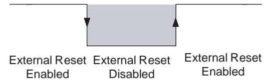
In order to be able to reset a Counter with Function 5, 6, 11, 12, 13 or 14, resetting must be Enabled by setting the Software Enable Reset Bit. Refer to 3-6 "Reset Signals" for detailed information about resetting Counters.
