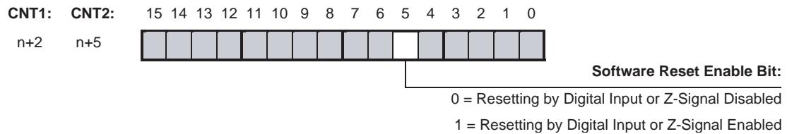
**Digital Input as Reset Enable Source** In order to use a Digital Input as Reset Enable Source you must assign Function 15 or 16 (= Enable/Disable Reset) to the corresponding Digital Input. Refer to 3-4 "Digital Input Functions" for more information.
