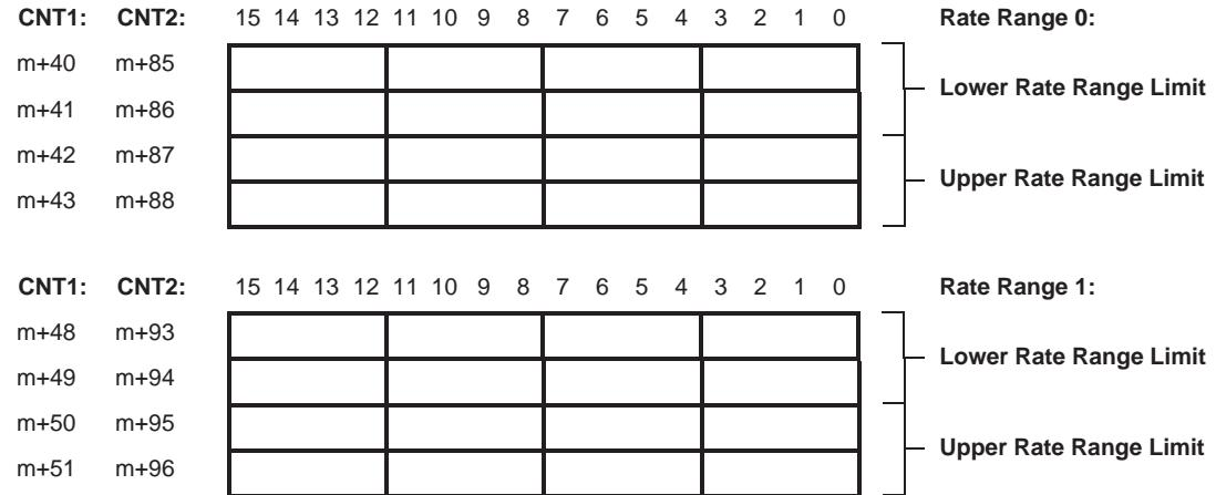
Set Lower- and Upper Range Rate Limits as a signed hexadecimal number between 80000000<sub>H</sub> and 7FFFFFFF<sub>H</sub> (i.e. -2,147,483,648 and +2,147,483,647 respectively). Make sure that the Upper Rate Range Limit > Lower Rate Range Limit.
