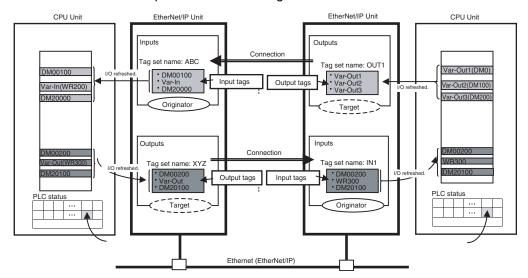
For communications between PLCs, the connection information is set in the EtherNet/IP Unit or built-in EtherNet/IP port of the PLC that receives data (i.e., the originator).
