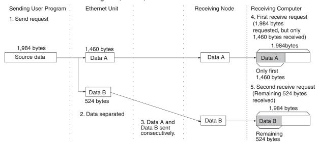
When using TCP protocol, the fragmented data is passed to the user program. Therefore, the receiving user program must be able to evaluate the end of the data transmission, and repeatedly send receive requests until all data has been received. The receive request is sent twice in the example shown above, but the data would be even more fragmented if a router was included in the communications path, and the number of receive requests would need to be increased accordingly.
