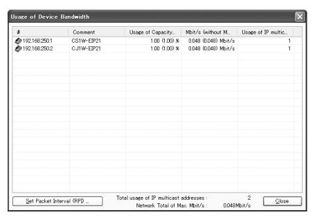
The *Usage of Capacity* column will show the percentage of the allowed tag data link bandwidth being used, and the *Mbit/s* column will show the network bandwidth being used.
