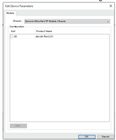
3. Select the slot number *00* in the *Configuration* from the Module Tab Page and then click the *Edit* Button. The Edit Module Parameters Dialog Box is displayed.
