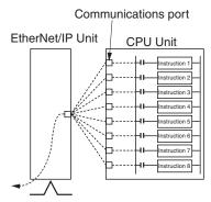
There are eight communications ports, so up to eight communications instructions can be executed at a time. The number of messages that can be sent or received with a single CPU Bus Unit service, though, is not more than two each for the CPU Unit to the EtherNet/IP Unit and for the EtherNet/IP Unit to the CPU Unit.
