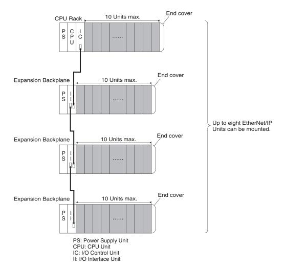
Note The CJ1W-EIP21/EIP21S EtherNet/IP Unit's maximum current consumption is 410 mA/650 mA. Be sure that the total current consumption of all the Units connected to the same CPU Backplane or Expansion Backplane does not exceed the output capacity of the Power Supply Unit.
