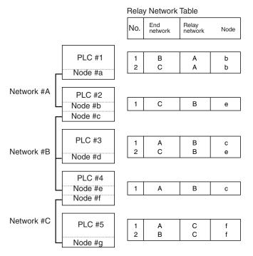
In the table for PLC #3, for example, if network #A is taken as the end network, then network #B becomes the relay network and node #c becomes the relay node. If network #C is taken as the end network, then network #B still becomes the relay network and node #e becomes the relay node.
