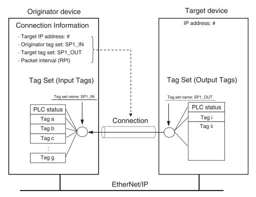
There are both input and output tag sets. Each tag set can contain only input tags or only output tags. The same input tag cannot be included in more than one input tag set.
