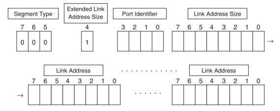
Always set the Link Address to an even number of bytes. If there is an odd number of bytes, pad the Link Address with "00" so that it has an even number of bytes.
