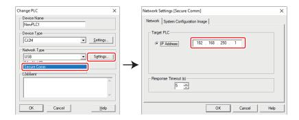
To open the Change PLC Dialog Box of the PLC Backup Tool, follow the steps below.
