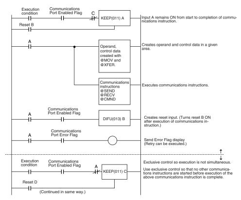
The execution status of the SEND(090), RECV(098), and CMND(490) instructions is always reflected by the communications flags (i.e., the Communications Port Enabled Flag and the Communications Port Error Flag). The CS/CJ-series CPU Unit's communications flags are allocated in the Auxiliary Area as shown in the following table.
