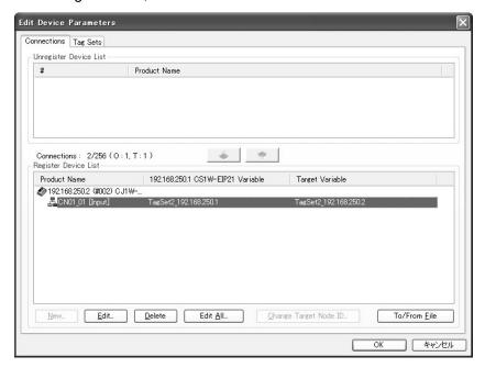
d. The device's Edit Connections Dialog Box will be displayed. Input a new RPI value, and click the **OK** Button.
