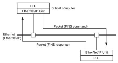
In the FINS communications service, both an IP address for IP (the Internet layer) and a FINS node address for FINS (the application layer) are used for the remote device. Also, 9600 is used as the default setting for the local UDP or TCP port number (i.e., the transport layer) for identifying the application layer, i.e., the FINS communications service. (Another number can be set for the FINS/UDP port from the Setup Tab Page in the Unit Setup.)
