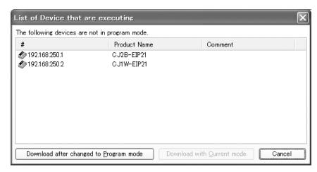
When the **Download after changed to Program mode** Button is clicked, all CPU Units will be changed to PROGRAM mode and the parameters will be downloaded. Confirm safety for all controlled equipment if the CPU Units are changed to PROGRAM mode. The operating mode can be returned to the previous setting after the parameters have been downloaded.
