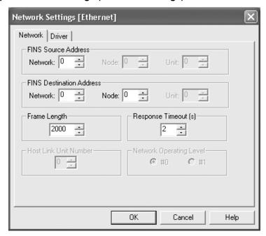
**Note** When FinsGateway is selected as the network type, make sure that the frame length is set to 2,000 bytes max.
