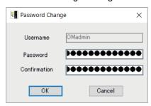
After completing the settings, click the **OK** Button. The changes are reflected immediately and enabled. Then, the EIP21S User Management Tool changes from online to offline.
