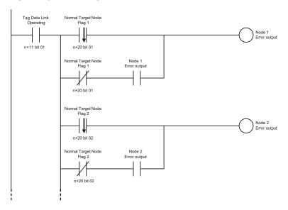
Programming to Detect Errors: Example 2
