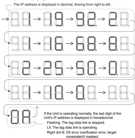
If an error occurs, the error code will be displayed alternately with the right-most byte of the affected device's IP address. For details on error codes, refer to SECTION 16 Troubleshooting and Error Processing.
