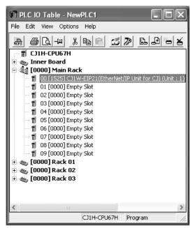
Note Creating I/O tables is not required if the built-in EtherNet/IP port of a CJ2 CPU Unit is used. It is registered as a built-in port/Inner Board with a model number of CJ2B-EIP21 for the CJ2H and a model number of CJ2M-EIP21 for the CJ2M. You cannot delete a built-in port from the I/O tables.
