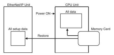
This operation will read the EtherNet/IP Unit or built-in EtherNet/IP port setup data file from the Memory Card and restore the data in the EtherNet/IP Unit or built-in EtherNet/IP port.
