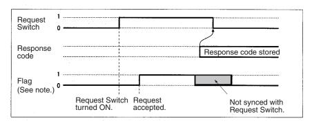
**Note** The Sending Flag and Receiving Flag will not turn ON if the highspeed socket service option is selected. Therefore, the program can be controlled only by setting the Send Request Switch and Receive Request Switch to OFF.
