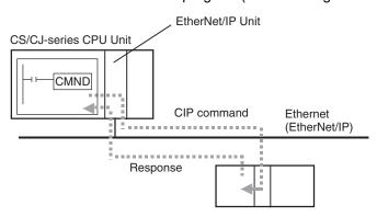
CIP messages (CIP commands and responses) can also be transferred to another CIP-based network via the EtherNet/IP Unit or built-in EtherNet/IP port using the CIP routing function for message communications.
