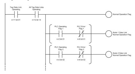
Programming to Detect Errors: Example 1
