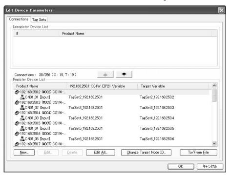
Information about the connection with device 192.168.250.20 is registered in the Register Device List. Double-click this connection to edit the settings.
