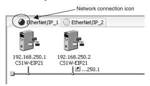
The connecting network can be switched by selecting **Network - Change Connect Network**.
