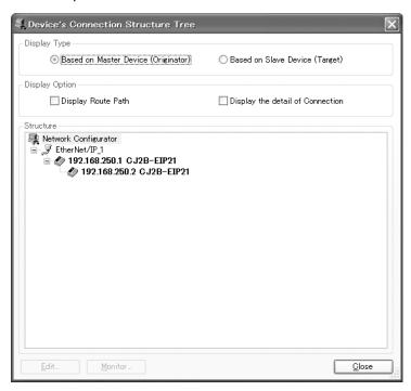
5. Use the device connection structure tree as required to change the RPI and timeout settings.
