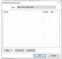
4. Select *Input Only (Tag type)* or *Input & Output (Tag type)* from *Type* and click the **New** Button. The Edit Variable Dialog Box is displayed.
