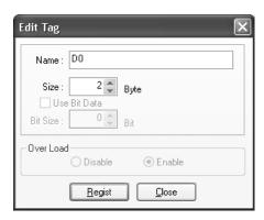
5. In the Name Field, enter the character string for the CPU Unit's I/O memory address or a network symbol (e.g., 100, W100, D0, Input\_signal). Addresses in the following I/O memory areas can be set.
