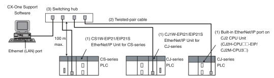
The devices shown in the following table are required to configure a network with CS1W-EIP21/EIP21S and CJ1W-EIP21/EIP21S EtherNet/IP Units or the built-in EtherNet/IP port in CJ2H-CPU□□-EIP/CJ2M-CPU3□ CPU Units.
