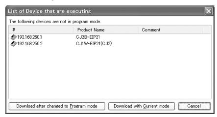
If the **Download after changed to Program mode** Button is clicked, all CPU Units will be changed to PROGRAM mode and the parameters will be downloaded. Confirm safety for all controlled equipment if the CPU Units are changed to PROGRAM mode. The operating mode can be returned to the previous setting after the parameters have been downloaded.
