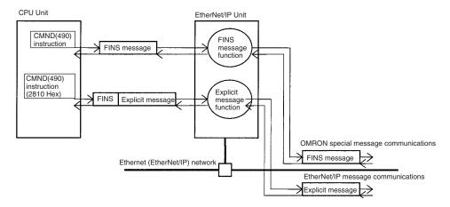
**Note** With the EtherNet/IP Unit or built-in EtherNet/IP port, message communications are possible even if the I/O link function is disabled.
