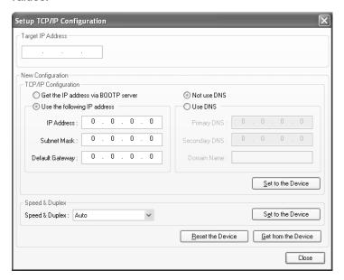
Enter the IP address to set and press the Get from the Device Button. The
