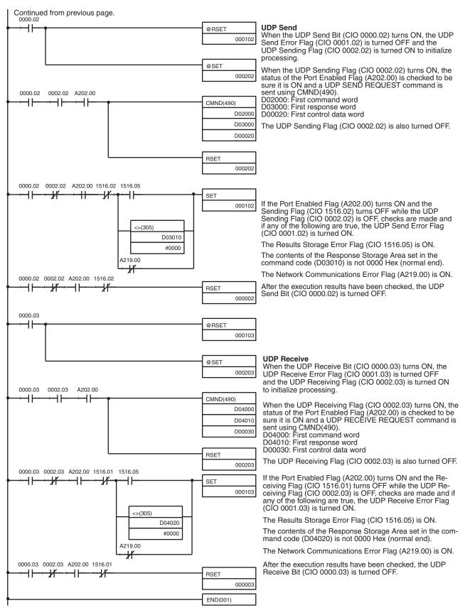
**Note** When using the above programming example, change the bit and word addresses as necessary to avoid using the same areas used by other parts of the user program or the CPU Bus Unit.
