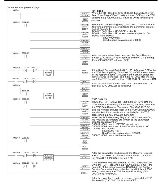
**Note** When using the above programming example, change the bit and word addresses as necessary to avoid using the same areas used by other parts of the user program or the CPU Bus Unit.
