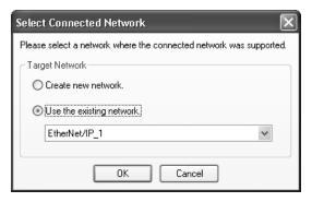
The Network Configurator will connect to the EtherNet/IP network. If the Network Configurator is connected online properly, *On-line* will be displayed in the status bar at the bottom of the window. The network connection icon will be displayed in blue in the Network Tab Page in which the Network Configurator is connected.
