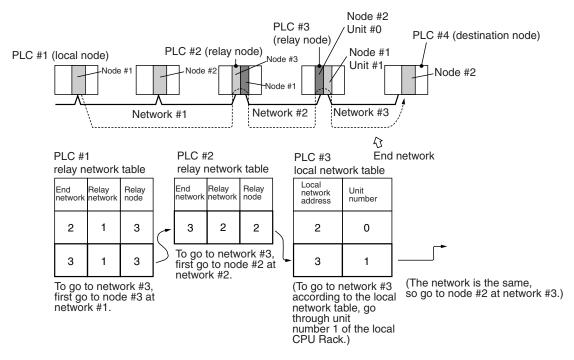
Note In the above example, the routing tables required for a message to reach PLC #4 from PLC #1 are shown. Additional settings would be required in the routing tables for a message to reach PLC #1 from PLC #4. Refer to 8-4-3 Rout-
