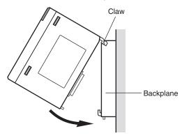
2. Insert the Unit into Backplane connectors and securely tighten the screw at the bottom of the Unit. Tighten the screws to a torque of 0.4 N·m.
