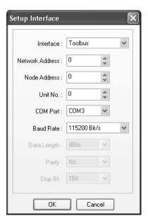
Input the EtherNet/IP Unit's unit number in the Unit No. Field, select the connecting COM port number, and click the OK Button. Usually, the Baud Rate is left at this setting. The following dialog box will be displayed.
