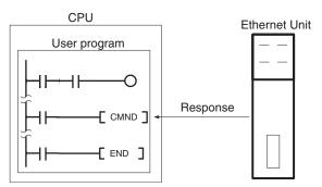
3. The Ethernet Unit starts the process requested by the parameters in the socket service request command.
