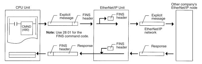
When sending an explicit message, set the local node's EtherNet/IP Unit or built-in EtherNet/IP port as the destination of the FINS command, and not the actual destination (other company's EtherNet/IP node). Specify the node address of the actual destination in the command data of the explicit message send command.
