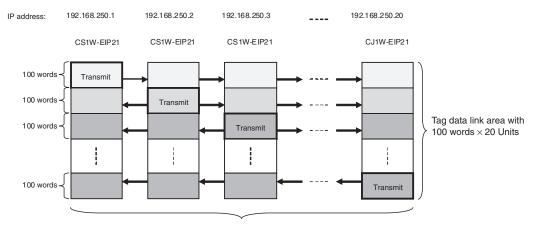
10 CS1W-EIP21 Units + 10 CJ1W-EIP21 Units = 20 Units total The RPI is 10 ms (Ethernet default) for all connections.
