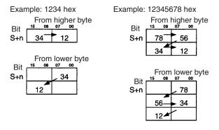
Similarly, when the additional status data and service response data in the response block is in word (2-byte) or double-word (4-byte) units, such as word
