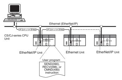
Various control operations (such as the reading and writing of I/O memory between PLCs, mode changes, and file memory operations) can be executed from the host computer by sending the corresponding FINS command with a UDP/IP or TCP/IP header attached.
