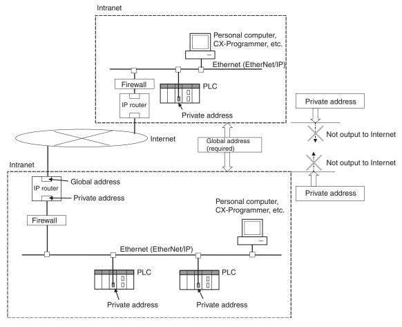
Communications Services That Require Global Addresses for EtherNet/IP Units and built-in EtherNet/IP ports A global address is required for the IP addresses of the EtherNet/IP Units and built-in EtherNet/IP port when the following communications services are used over the Internet.
