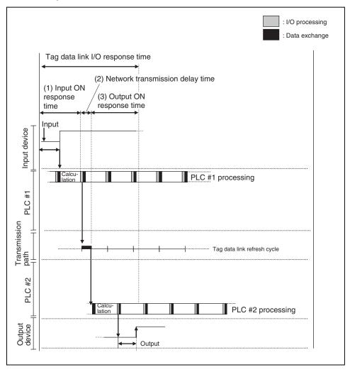
The minimum tag data link I/O response time, which occurs when there are no processing delays, is calculated as follows.
