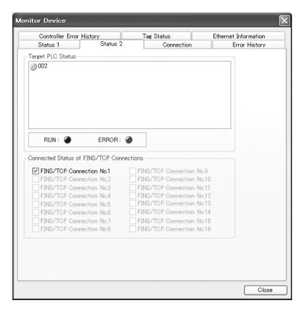
**Note** The target PLC status can be used when the PLC status is selected for all the target sets for both originator and target connections. For those that are not selected, the status will be grayed-out.
