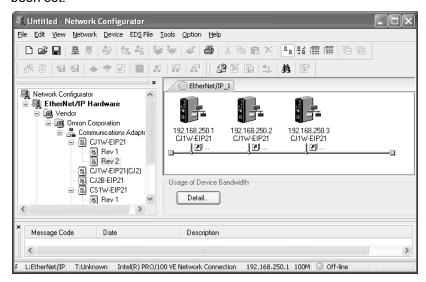
7. Connect the Network Configurator to the EtherNet/IP network and select **Network** – **Download** from the menus. The data link settings will be downloaded to the EtherNet/IP Units, and the data links will operate.
