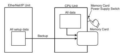
This operation will create an EtherNet/IP Unit or built-in EtherNet/IP port settings file, and write that file to the Memory Card along with the other backup files. When the Memory Card Power Supply Switch is pressed, the MCPWR indicator on the front of the CPU Unit will flash once and then remain lit while data is being written. If the data is written normally, the MCPWR indicator will turn OFF. The BUSY indicator will flash while the data is being written.
