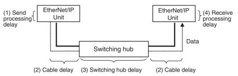
The lengths of these delays depend on many factors, such as the tag data link connection settings (number of connections and data sizes), number of nodes, the switching hub being used, and cable lengths. Each delay is described in detail below.
