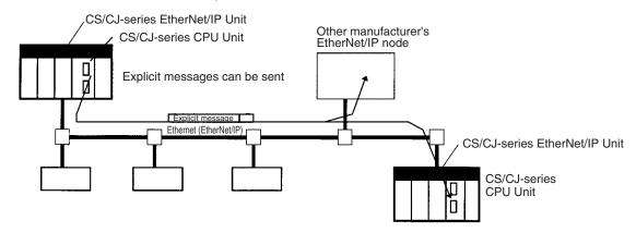
When the destination is another company's EtherNet/IP node, an explicit message can be sent to the EtherNet/IP Unit or built-in EtherNet/IP port using FINS command code 28 01 or 28 10, through the Connection Manager class's Unconnected Send service, as shown in the following diagram.
