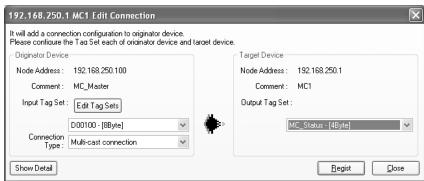
Select the output tag set from *Target Device* Area on the right side of the Edit Connection Dialog Box, and then select the input tag set to receive the output tag set in the *Originator Device* Area on the left.
