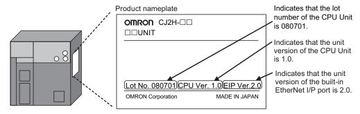
In this manual, the version of the EtherNet/IP port built into the CJ2H-CPU□□-EIP/CJ2M-CPU3□ CPU Unit is given as the unit version.
