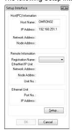
Click the Setup Button in the Setup Interface Dialog Box. The Registration of the connection Dialog Box will be displayed. Enter the network information for the connection destination, and then click the Add Button to register the settings.
