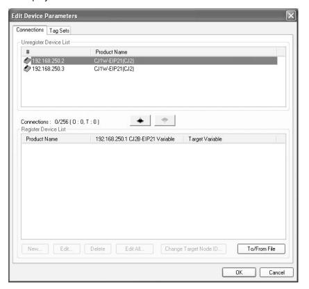
3. In the Unregister Device List, select the target device that requires connection settings by clicking the device so its color changes to gray, and click
