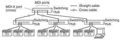
Some switching hubs can automatically distinguish between MDI and MDI-X. When this kind of switching hub is being used, straight cable can be used between switching hubs.
