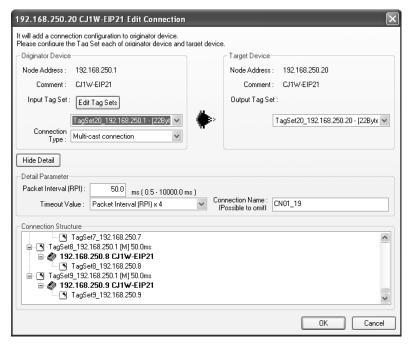
In the Edit Connection Dialog Box, input 1.0 ms as the new RPI value, and click the **OK** Button. The tag data link bandwidth being used by device 192.168.250.1 (Usage of Capacity) increases to 54.67%, which indicates that a RPI is set to a higher speed for this device.
