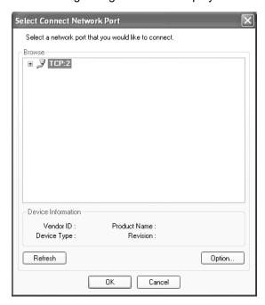
4. After clicking **TCP:2**, click the **OK** Button. The Network Configurator will be connected to the EtherNet/IP network. If the Network Configurator is connected online properly, *On-line* will be displayed in the status bar at the bottom of the window.
