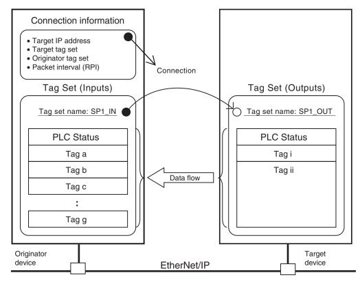
Note (1) In this example, a connection is established with the originator's tag list containing tags a to g (inputs), which are grouped in a tag set called SP1\_IN, and the target's tag list containing tags i and ii (outputs), which are grouped in a tag set called SP1\_OUT.
