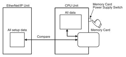
This operation will compare the data in the EtherNet/IP Unit or built-in EtherNet/IP port setup file in the Memory Card with the device parameters in the EtherNet/IP Unit or built-in EtherNet/IP port.
