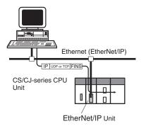
The FINS gateway function enables access to PLCs on not only the same Ethernet network but on various other networks, including SYSMAC LINK and Controller Link.
