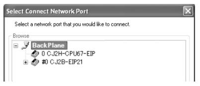
6. Click the + icon to the left of the EtherNet/IP Unit or built-in EtherNet/IP port (CJ1W-EIP21(CJ2)/CJ1W-EIP21S(CJ2) or CJ2B-EIP21). The TCP ports on the EtherNet/IP Unit will be displayed as shown below.
