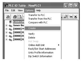
Executing the I/O table creation command causes the EtherNet/IP Unit to be restarted. After the EtherNet/IP Unit is restarted, perform transfer operation in the dialog box that is displayed.
