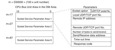
Turn ON the Socket Service Request Switches in the CPU Bus Unit Area in the CIO Area.
