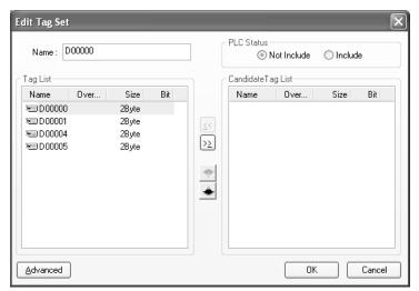
Up to 8 tags can be registered in a tag set, or up to 7 tags can be registered and two byes will be added to the size if the PLC status is included in the tag set.
