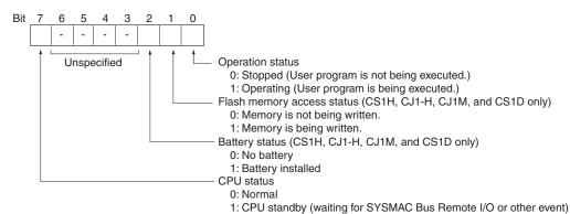
• **Operating mode:** Returns the operating mode of the CPU Unit in 1-byte (2-digit) hexadecimal.
