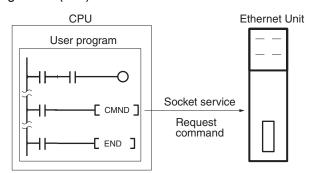
2. CMND(490) ends normally when the socket service request command is received and a response is returned (response code: 0000).
