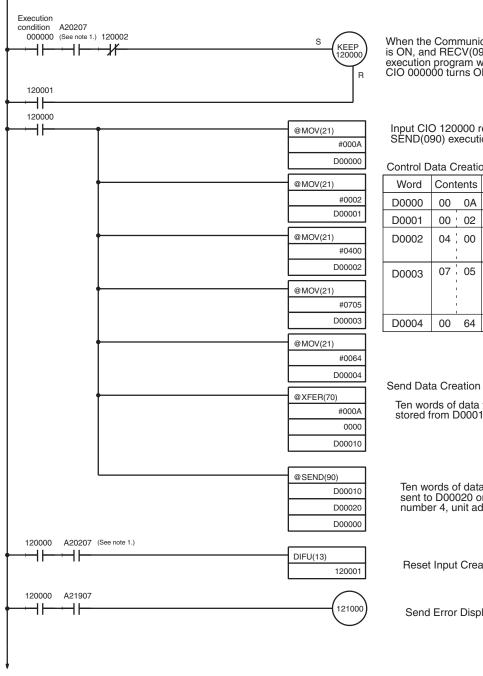
When the Communications Port Enabled Flag for port 7 is ON, and RECV(098) is not being executed, the send execution program will start when execution condition CIO 000000 turns ON.
