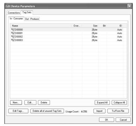
12. If an input tag has already been registered in an input tag set, and you want to change its registration to a different input tag set, it is necessary to delete the tag from the tag set in which it was originally registered.
