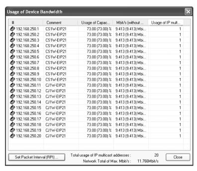
Method 2: Changing the Packet Interval (RPI) of Only Specific Devices
