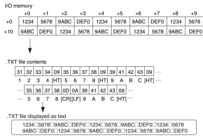
□...[HT]: Used to display tab space when displayed as text.
