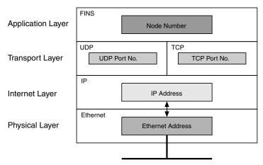
The FINS communications service is a communications method based on UDP/IP, and it is supported by most OMRON Ethernet-related products. (In this manual it is called the FINS/UDP method.) In addition to supporting the FINS/UDP method, the CS1W-EIP21, CS1W-EIP21S, CJ1W-EIP21, CJ1W-EIP21S, CJ2H-CPU□□-EIP, and CJ2M-CPU3□ support FINS communications using TCP/IP. (In this manual, this is called the FINS/TCP method.)
