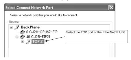
Select the port for the EtherNet/IP Unit and then click the **OK** Button. The Network Configurator will be connected to the EtherNet/IP network. If the Network Configurator goes online normally, "On-line" will be displayed in the status bar at the bottom of the window. **Note**
