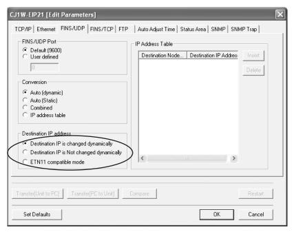
Note If the ETN11-compatible mode is used, the internal table will retain the same content from when it was created after the EtherNet/IP Unit was turned ON or restarted. This feature provides protection from access via FINS/UDP from computers that dynamically change their IP address.
