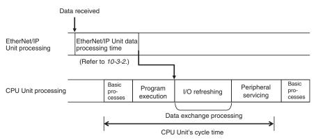
If there is an interrupt for data transmission processing, the CPU Unit's cycle time is extended by that interrupt processing time. Refer to 10-3-2 EtherNet/IP Unit or CJ2H Built-in Port Data Processing Time for details.
