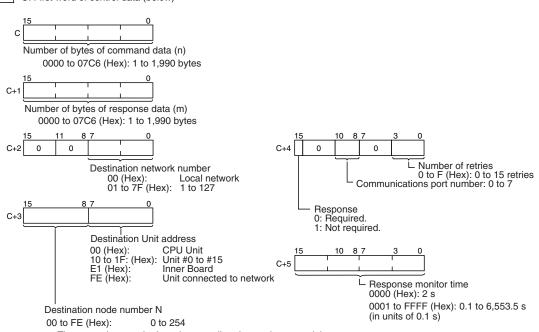
The same data can be broadcast to all nodes on the network by setting the destination node number to FF (Hex).
