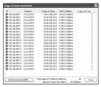
In this case, if there is no multicast filter, the value becomes 106.33%. If there is no multicast filter for a switching hub, communications errors may occur depending on the communications load of the EtherNet/IP Unit or built-in EtherNet/IP Unit port.
