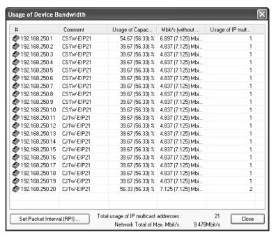
In this case, the tag data link bandwidth being used by device 192.168.250.20 (Usage of Capacity) also increases (from 39.67% to 56.33%).
