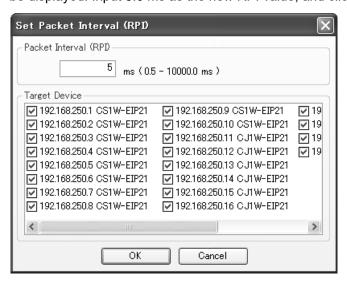
If the packet interval for all connections has been set to the same setting, the dialog box will show that the usage of capacity for the tag data link's allowable communications bandwidth is 73.00% and the fastest set value is 5.0 ms.
