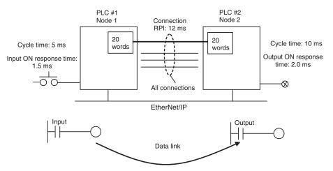
For example, the maximum and minimum I/O response times would be as follows for the above system.
