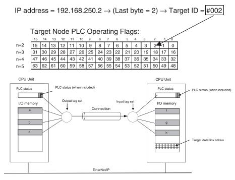
Note The target ID may be duplicated depending on the IP addresses of the target nodes. In this case, it is necessary to change the target ID with the Network Configurator. For information on how to change the device number, refer to step 4 under Registering Devices in the Register Device List on page 174.
