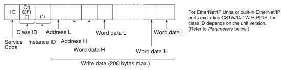
Note A body format of either 8 bits or 16 bits is possible.
