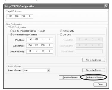
4. Press the **Set to the Device** Button. The IP address will be transferred to the device. The applicable device is the device specified in the *Target IP Address* Box. The device must be reset to enable the transferred setting. If the device is not reset when the new IP address is transferred, click the **Reset the Device** Button.
