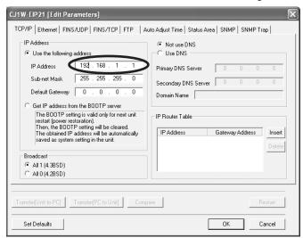
If the IP address is set in the TCP/IP Tab Page, that IP address setting will be displayed in the IP Address Display/Setting Area (words m+98 and m+99) in the DM Area words allocated to the Unit/port.
