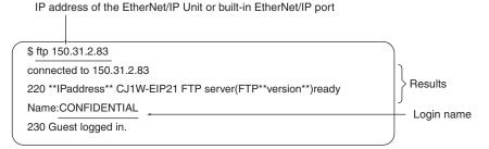
3. Enter FTP commands (underlined in the following diagram) to read and write files. The following directory tree is used in this example.
