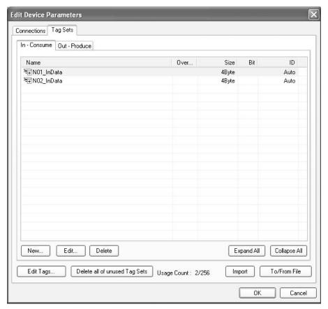
To place more than one input symbol (input tag) imported from the CX-Programmer into one tag set, you must delete the input tags that were registered to separate input tag sets.
