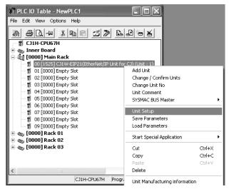
2. Right-click the EtherNet/IP Unit or built-in EtherNet/IP port in the I/O table and select *Edit - Unit Setup* from the menus. The Edit Parameters Dialog Box will be displayed.
