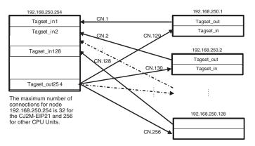
Another EtherNet/IP Unit must be mounted to the PLC to increase the maximum number of connections. (Refer to the following figure.)
