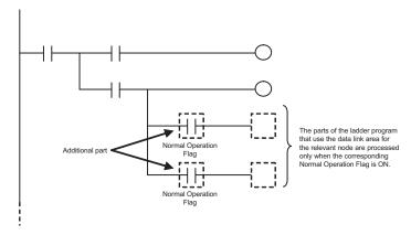
Interlocks (IL and ILC instructions) and jumps (JMP and JME instructions) can also be used to process data only when the data links are operating normally as shown below.
