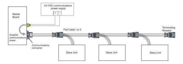
The BS+ and BS- terminals of a 24-VDC communications power supply are connected to the communications power supply connector provided on the Master Board. This connection provides all Slave Units on the trunk line, which are connected to the Master Board via round cables II, Flat Cable I or Flat Cable II, with the communications power.
