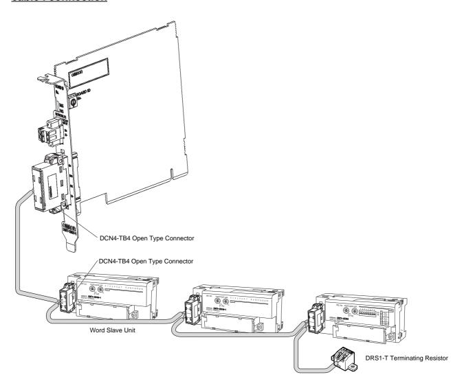
**Note** A commercially available relay terminal block can make a T-branching connection.
