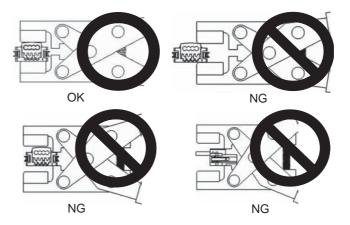
3-3 Confirm that it is properly pressure-welded as shown below:
