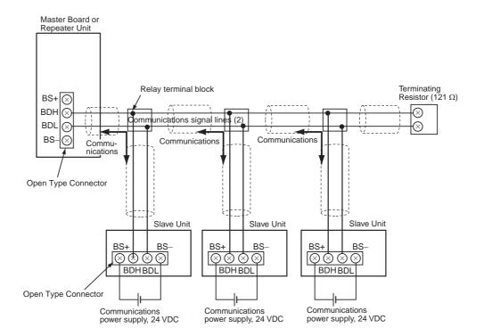
Master Board or Repeater Unit Terminating Resistor (121 Ω) BS+ BDH BDL  $\otimes$ BS-Communications Open Type Connector Communications Communications Slave Unit Slave Unit Slave Unit BS. BS BS-BDH BDL BDH BDL BDH BDL Open Type Connector
