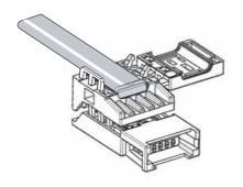
3-2 Hold the cable to prevent dislocation. Close the cover to sandwich the cable.
