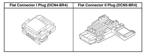
Align the Plug face with the color seals (red, white, blue and black) matching the signal names (red and BS+) on the connector. Press the plug until it clicks into place.
