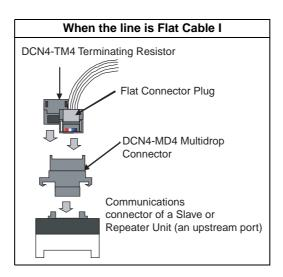
Method 3 Connect a Terminating Resistor to the trunk line or a sub-trunk line cable.
