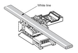
For Cable extension or connecting a Terminating Resistor
