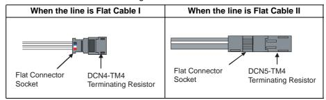
Method 2 Attach a Multidrop Connector on the communications connector (or an upstream port) provided on a Slave Unit or Repeater Unit.
