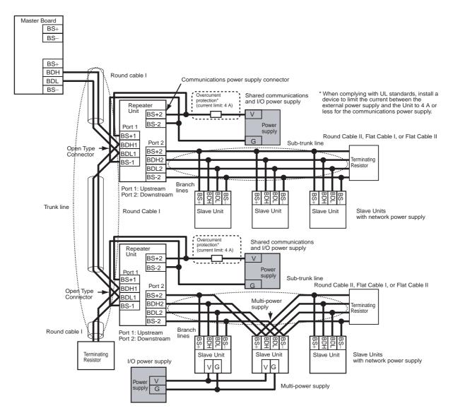
Note Depending on the I/O device to which the Slave Unit is connected, an I/O power supply connected to a multi-power supply Slave Unit may be a source of noise. Even when the communications power is supplied collectively to all Slave Units, a separate I/O power supply must be provided so that noise does not affect the network.
