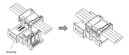
**Note** Once it is attached, the housing cannot be removed from the cover. If you attempt to remove it forcibly, you may damage the connector.
