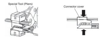
4-3 Confirm that the cable is properly pressure-welded as shown below:
