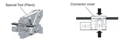
5-2 Squeeze the Pliers firmly until the lock on Connector clicks into place.
