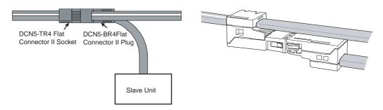
**Note** The same type of cable must be used for the trunk line and branch lines.
