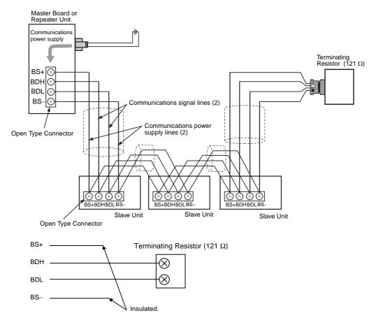
You can also use the DRS1-T Terminating Resistor for termination. If you do, insulate the ends of the BS+ and BS- lines.
