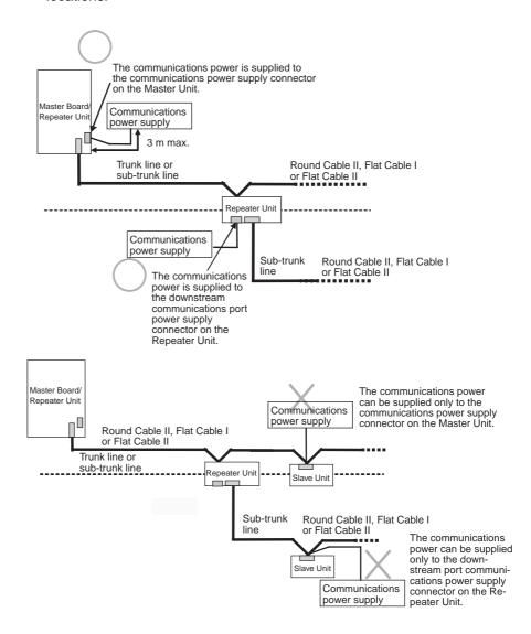
• Provide a separate power supply each for the Master Board trunk line, for the upstream, and for the downstream trunk line of a Repeater Unit.
