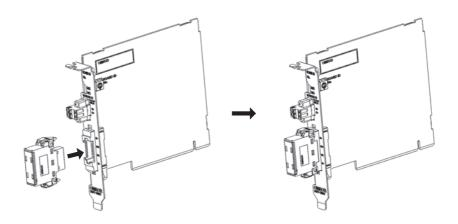
**Note** To remove the inserted Connector, hold the latches on both sides and pull out the Connector.
