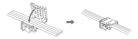
For Cable extension or connecting a Terminating Resistor Insert the tip of the cable all the way into the cable stopper in the cover.
