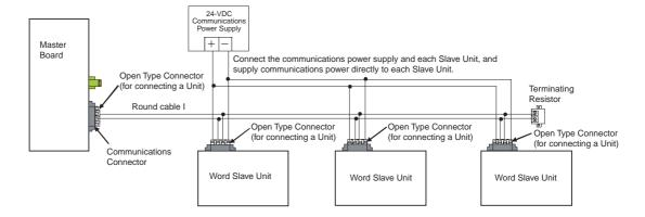
The BS+ and BS- terminals of a 24-VDC communications power supply are connected directly and individually to all Slave Unit and Repeater Unit\*. The power supply is not connected to the Master Board.
