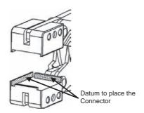
3-2 Squeeze the Pliers firmly until the lock on the Connector clicks into place.
