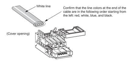
2-2 Hold the Cable to prevent dislocation. Close the cover to sandwich the Cable.
