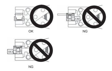
5-3 Confirm that it is properly pressure-welded as shown below:
