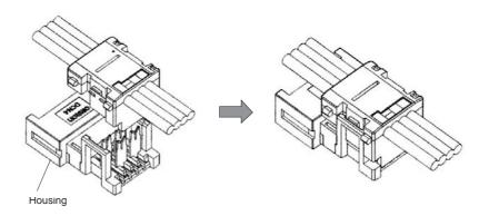
**Note** Once it is attached, the housing cannot be removed from the cover. If you attempt to remove it forcibly, you may damage the connector.
