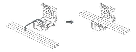
3-2 lose the cover and sandwich the cable. Secure the hook.
