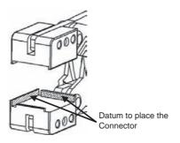
4-2 Squeeze the Pliers firmly until the lock on the Connector clicks into place.
