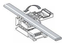
**Note** When it is for cable extension or for connecting a Terminating Resistor, be sure to insert the cable tip all the way to the cable stopper in the cover. Be sertain the cable won't come out.
