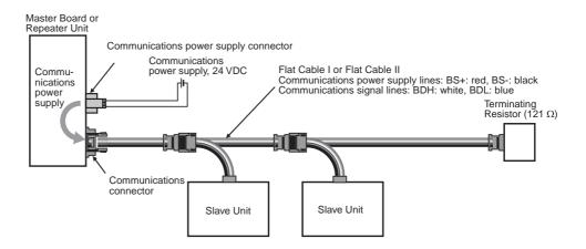
When Flat Cable I is used, Slave Units can be connected in parallel also by multidrop connections. A DCN4-MD4 Multidrop Connector is used for this connection.
