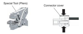
3-2 Squeeze the Pliers firmly until the lock on the Connector clicks into place.
