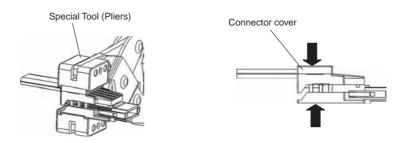
3-3 Confirm that the cable is properly pressure-welded as shown below.
