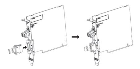
**Note** To remove the inserted Plug, hold the latches on both sides and pull out the Plug
