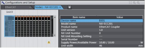
However, the Sysmac Studio determines excess and insufficiency in the supplied power for an NX Unit power supply capacity of 10 W max. It does not consider the power supply restrictions of the NX Unit power supply in actual application conditions and I/O power supply design conditions. When actually designing the power supply, refer to 5-2-1 Procedure for Designing the NX Unit Power Supply System on page 5-6 and 5-3-2 Designing the I/O Power Supply from the NX Bus on page 5-10.
