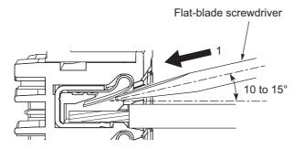
**2** Leave the flat-blade screwdriver pressed into the release hole and pull out the wire.
