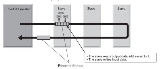
The data exchanges that are cyclically performed between the EtherCAT master and EtherCAT slaves use EtherCAT datagrams that are stored directly in the Ethernet frames.
