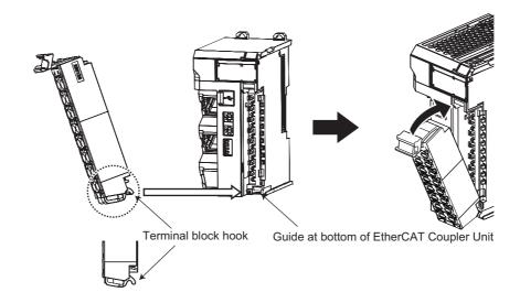
Mount a terminal block that is applicable to the model of the EtherCAT Coupler Unit. Refer to *4-5 Terminal Blocks* on page 4-14 for the applicable terminal blocks.
