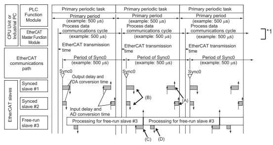
\*1. For a built-in EtherCAT port that can perform process data communications with a Slave Terminal in more than one periodic task, this is called process data communications cycle 1.
