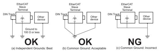
If the DIN Track is made of steel and the surface is not treated to produce an insulating material, you can omit grounding the functional ground terminal on any Unit that has one, as shown in the following figures.
