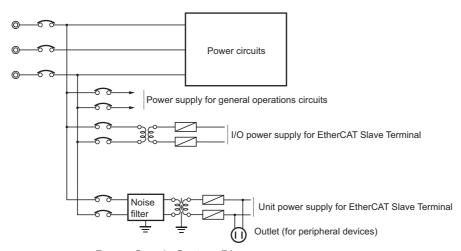
Power Supply System Diagram
