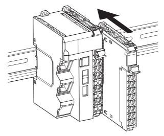
Press the NX Unit with a certain amount of force against the DIN Track until you hear the DIN Track mounting hook lock into place.
