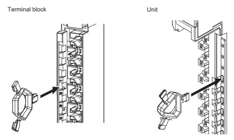
Rotate the runner to break off the Coding Pin.
