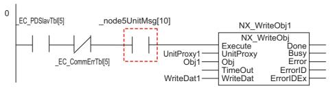
\_node5UnitMsg[10]: This is a device variable for the EtherCAT Coupler Unit (with node address 5) to which the NX Unit Message Enabled Status (NX Unit number 10) is assigned.
