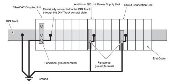
If the DIN Track is made of steel and the surface is not treated to produce an insulating material, you can omit grounding the functional ground terminal on any Unit that has one, as shown in the following figures.
