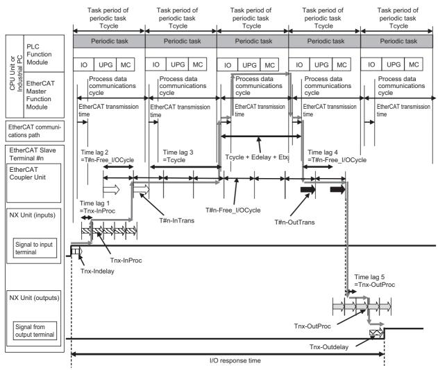
The maximum and minimum values of the I/O response time are calculated as shown below. The minimum value occurs when the time lags that are shown in the above figure do not occur.
