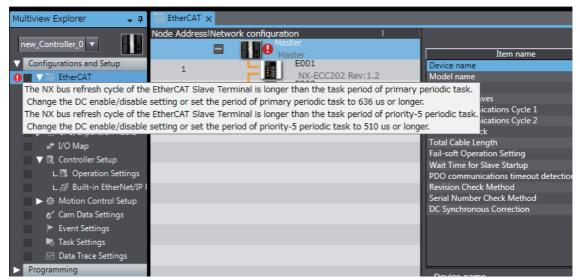
With the task period of the primary task or priority-5 periodic task in Configurations and Setup – Task Settings, select the task periods from the lists for the Period/Execution Conditions for both the primary task and priority-5 periodic task.
