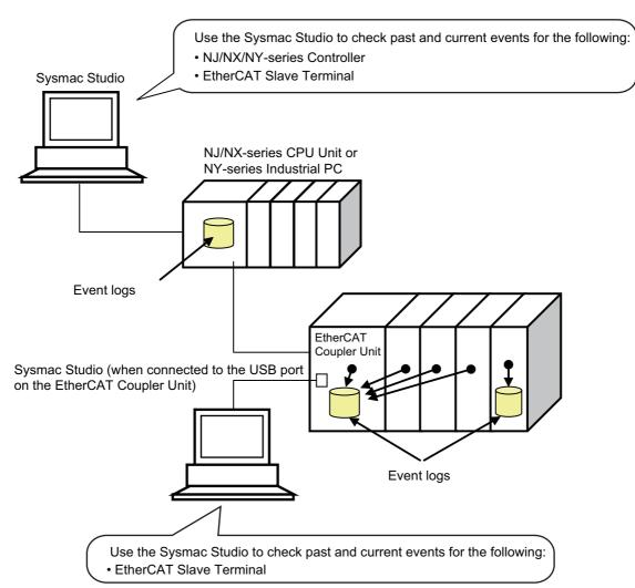
"Event" for an EtherCAT Slave Terminal is a generic term for an unexpected error or for information that does not indicate an error but for which the user must be notified.
