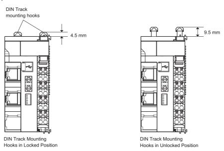
If the DIN Track mounting hooks are pressed down, they are in the locked position.
