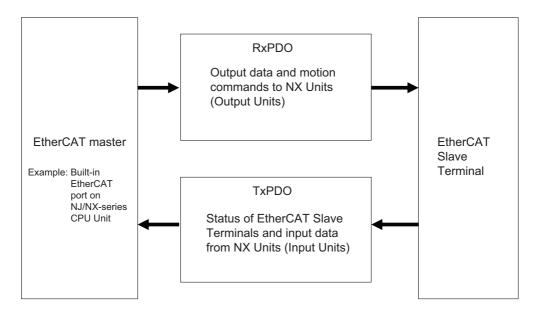
The EtherCAT application layer can hold more than one object to enable the transfer of various process data of the EtherCAT Slave Terminal.
