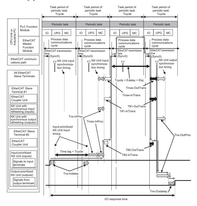
The maximum and minimum values of the I/O response time are calculated as shown below. The minimum value occurs when the time lag that is shown in the above figure does not occur.
