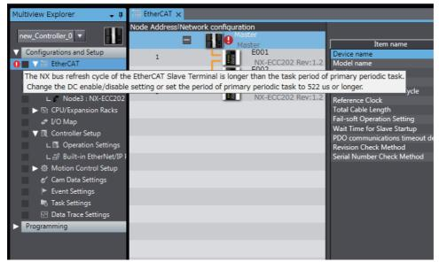
With the primary periodic task in Configurations and Setup - Task Settings, select the task period from the list for the Period/Execution Conditions.
