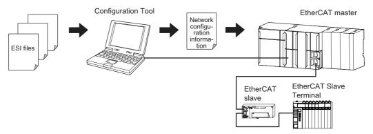
Communications are started according to the communications settings and the network configuration based on the ESI files that are installed.
