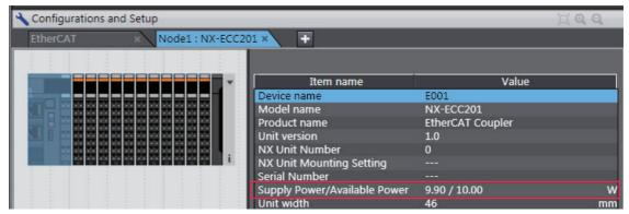
If the power to supply exceeds the NX Unit power supply capacity of the Unit that is selected to supply the NX Unit power, a yellow warning icon is displayed by the first NX Unit for which there is not sufficient capacity and also by all the remaining NX Units.
