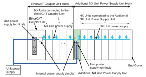
The total of the required Unit power supply capacity for these two blocks is the required power supply capacity of the Unit power supply for the EtherCAT Slave Terminal.
