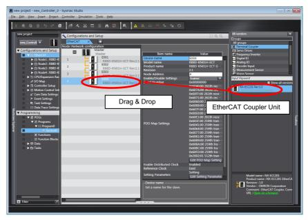
Select the EtherCAT Coupler Unit on the EtherCAT Configuration Edit Tab Page. The slave parameters of the EtherCAT Coupler Unit as an EtherCAT slave are displayed in the Slave Parameters Pane on the right side of the EtherCAT Configuration Edit Tab Page.
