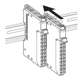
Press the NX Unit with a certain amount of force against the DIN Track until you hear the DIN Track mounting hook lock into place.
