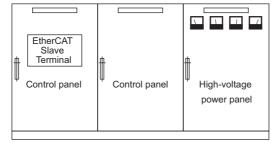
**Example of Poor Equipment Arrangement**
