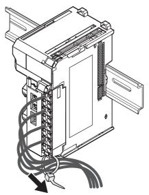
Secure wires within the range of 30 mm from the screwless clamping terminal block.
