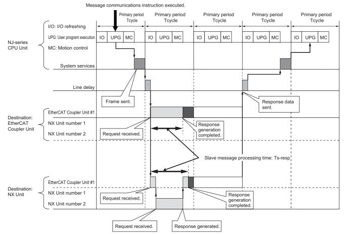
The definitions and values of Ts-resp are the same as the definitions and values for the calculation formula when connected to the built-in EtherCAT port on an NX-series CPU Unit.
