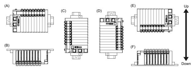
However, there are restrictions on the installation orientation of the EtherCAT Coupler Unit due to the ambient operating temperature and the NX Unit power supply capacity.
