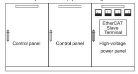
Examples of Equipment Arrangement in Panel with High-voltage Devices
