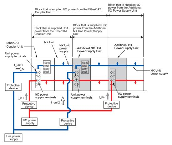
However, fewer protective devices may be required when the current consumption of each block does not exceed the rated current. An example of this is provided below.
