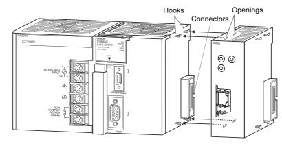
**2** Move the yellow sliders on the top and bottom of the Unit until they click into position, to lock.
