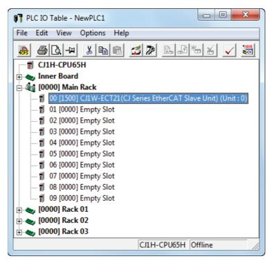
2 Right-click the EtherCAT Slave Unit in the I/O table and select *Unit Setup* from the menus.
