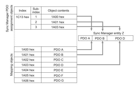
In this example, three PDOs (PDO A, PDO B, and PDO D) are assigned to index 1C13 hex (for the TxPDOs).
