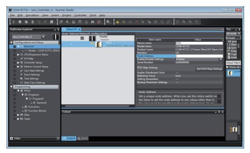
4 Set the PDO mapping of the EtherCAT Slave Unit. Assign the PDOs of the same size as the setting value of the IN and OUT data area size in the I/O Communication Area Setting Table of the EtherCAT Slave Unit.
