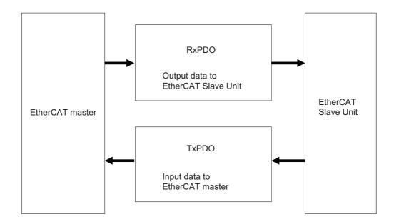
The EtherCAT application layer can hold more than one object to enable the transfer of various process data of the EtherCAT Slave Unit.
