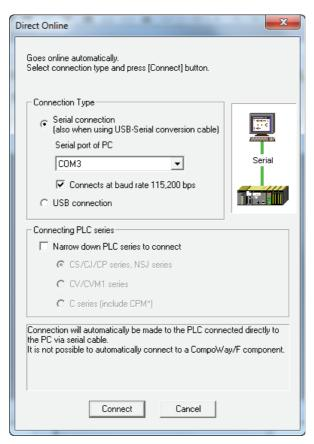
If the connection process is successful, the system will be connected online. Here, check the operating mode of the PLC. If the operating mode is not PROGRAM mode, change the mode by selecting *PLC - Operating Mode - Program* from the menus.
