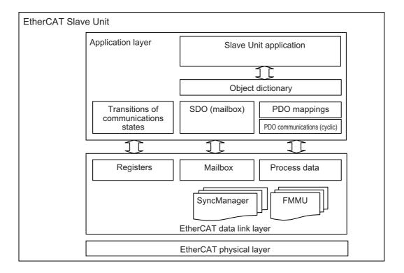
The object dictionary for the CAN application protocol is broadly divided into PDOs (process data objects) and SDOs (service data objects).
