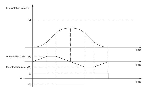
Vt: Specified interpolation velocity, At: Specified acceleration rate, Dt: Specified deceleration rate, Jt: Specified jerk
