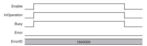
The following timing chart is for when an unused axis is specified or when an MC Test Run is in progress.
