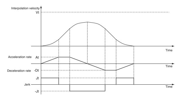
Vt: Specified interpolation velocity, At: Specified acceleration rate, Dt: Specified deceleration rate, Jt: Specified jerk
