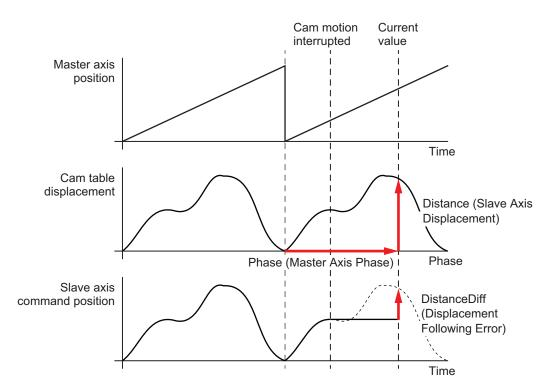
The command current position of the slave axis can be moved onto the cam profile curve by using the monitored *DistanceDiff* (Displacement Following Error).
