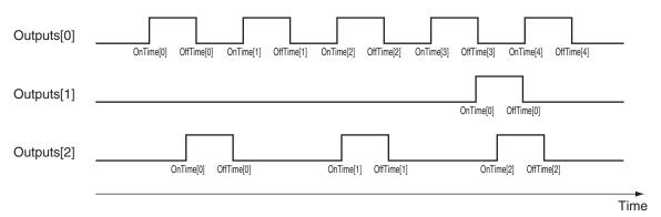
The NX\_AryDOutTimeStamp instruction turns the actual digital outputs ON or OFF according to *OnTime* (ON Time) and *OffTime* (OFF Time) in the parameter that is specified for *SetDOut* (Output Pulses).
