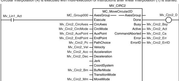
Circular interpolation (4) is executed with multi-execution of instructions after linear interpolation (1) is started.
