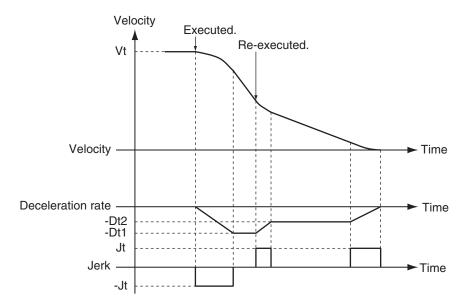
Vt: Velocity when deceleration starts, Dt: Specified deceleration rate, Jt: Specified jerk
