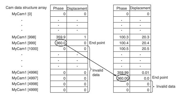
If this instruction is not executed even though the phases for MyCam1[1000] to MyCam1[4997] were overwritten to values other than 0, cam operation will be executed between MyCam1[0] to MyCam1[999].
