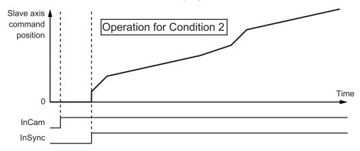
If *SlaveOffset* is set to -80, the slave axis starts synchronization from a displacement of *MasterStartDistance* (Master Following Distance) and rapid acceleration is prevented.
