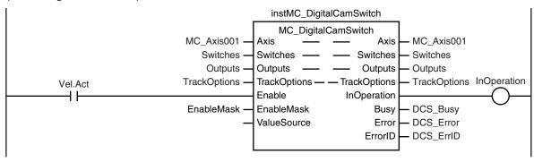
After the MC\_DigitalCamSwitch (Enable Digital Cam Switch) instruction for axis 2 starts operating, the NX\_AryDOutTimeStamp (Write Digital Output Array with Specified Time Stamps) instruction is executed.
