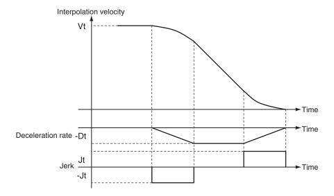
Vt: Velocity when deceleration starts, Dt: Specified deceleration rate, Jt: Specified jerk
