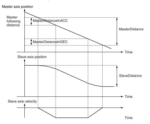
The relationship between the travel distance of the master axis and the travel distance of the slave axis is shown in the following table.
