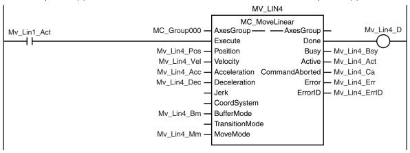
Linear interpolation (5) is executed with multi-execution of instructions after linear interpolation (1) is started.
