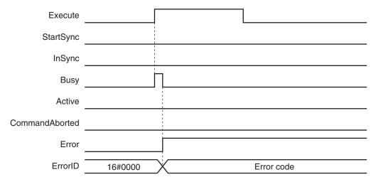
The slave axis is not affected by the error status of the master axis during synchronized control. After the error status of the master axis is cleared, the slave axis continues electronic gear operation when the master axis operates.
