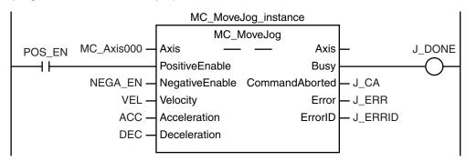
To use the master control instructions (MC and MCR) for the MC\_MoveJog (Jog) instruction, do not program the instructions as shown below. If you do, master control is applied only to *PositiveEnable* (Positive Direction Enable), i.e., it is not applied to *NegativeEnable* (Negative Direction Enable).
