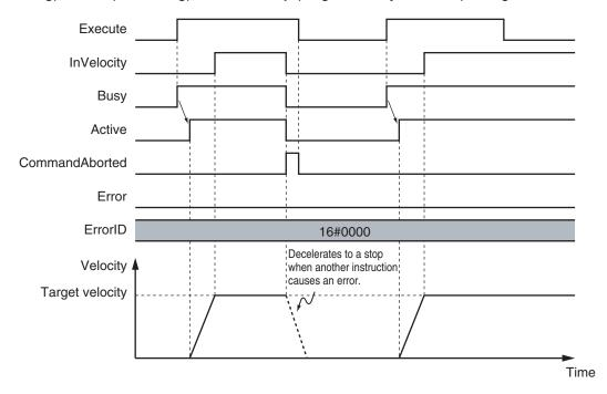
The *InVelocity* (Target Velocity Reached) output variable indicates when the velocity has reached the same velocity for this instruction and the re-executed motion control instruction. Therefore, after *InVelocity* (Target Velocity Reached) changes to TRUE, even if the velocity is changed by the override factor, *InVelocity* (Target Velocity Reached) will not change to FALSE.
