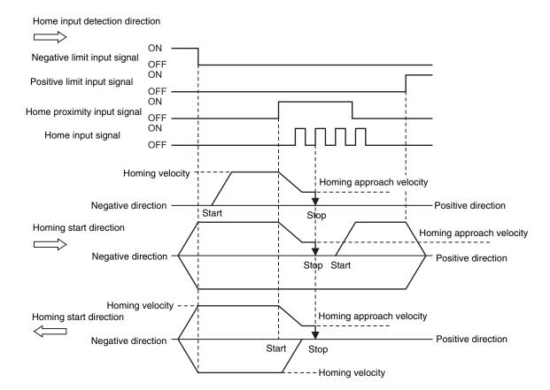
• If you start homing while the home proximity input signal is ON, the axis performs the following operation depending on the setting of the homing start direction.
