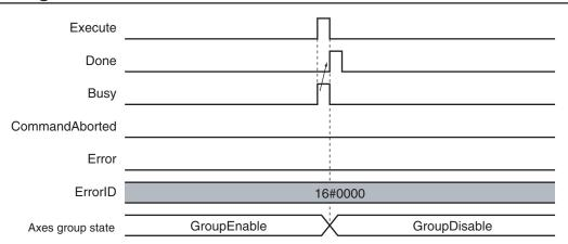
If you execute the MC\_GroupDisable instruction for an *AxisGroup* that is under multi-axes coordinated control, *CommandAborted* of multi-axes coordinated control instruction will change to TRUE. *CommandAborted* of any buffered multi-axes coordinated control instruction will also change to TRUE. If the axes are moving, they will decelerate to a stop at the maximum deceleration rate for each axis.
