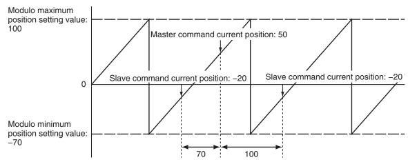
IDeviatedValuel is 70 (because 70 is less than 100). The sign is positive because the command current position of the *Master* is greater than or equal to the command current position of the *Slave*, so the *DeviatedValue* is +70.
