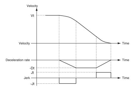
Vt: Velocity when deceleration starts, Dt: Specified deceleration rate, Jt: Specified jerk
