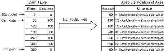
Slave axis 0 + Absolute position of slave axis at start point of cam table 200 + Absolute position of slave axis at start point of cam table 100 + Absolute position of slave axis at start point of cam table 300 + Absolute position of slave axis at start point of cam table 100 + Absolute position of slave axis at start point of cam table 200 + Absolute position of slave axis at start point of cam table 0 + Absolute position of slave axis at start point of cam table
