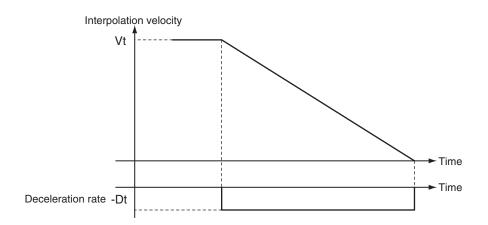
Vt: Velocity when deceleration starts, Dt: Specified deceleration rate
