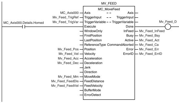
If home is defined for axis 2 and interrupt feeding is completed for axis 1, absolute positioning is performed for axis 2.
