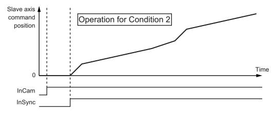
Example 2: Differences in Slave Axis Operation for Differences in *StartPosition* and *MasterStartDistance*
