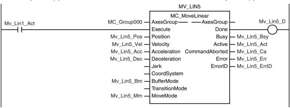
Linear interpolation (6) is executed with multi-execution of instructions after linear interpolation (1) is started.
