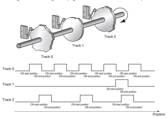
*TrackNumber* corresponds to the cam number. The values of the *FirstOnPosition* (ON Start Position) and *LastOnPosition* (ON End Position) correspond to the shape of the cam.
