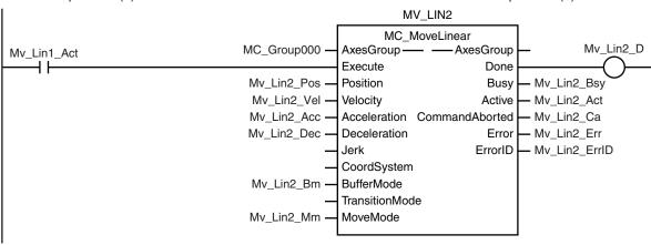
Linear interpolation (3) is executed with multi-execution of instructions after linear interpolation (1) is started.
