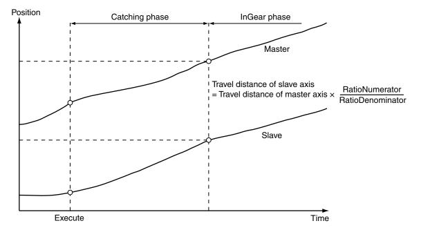
If the gear ratio is negative, Slave (Slave Axis) and Master (Master Axis) move in the opposite directions.
