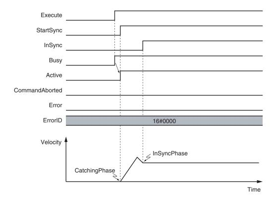
The slave axis follows the master axis position before the InSync phase as well. An example of this is shown below.
