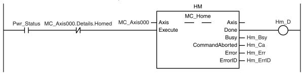
After home is defined, absolute positioning 1 is executed to move to 290.0°. The shortest way is specified for the motion direction.
