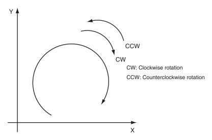
Specify the axes to use as the X axis and Y axis with *CircAxes* (Circular Axes). Use logical axes (axis A0 to A3) for the axes, and not axis numbers.
