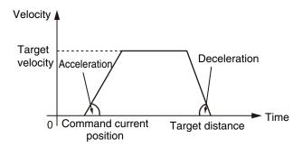
When the *Acceleration* (Acceleration Rate) or *Deceleration* (Deceleration Rate) is 0 and the instruction is executed, the axis will reach the target velocity without accelerating or decelerating.
