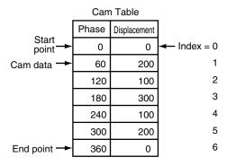
The command positions for the master and slave axes are linear interpolations between two cam data where the slave axis displacement corresponding to the master axis phase is calculated.
