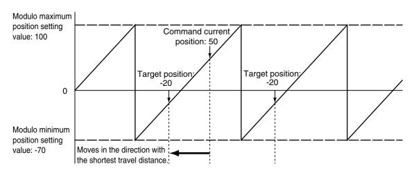
Movement is in the same direction as **3:** \_mcCurrentDirection (Current direction) if the travel distance is the same in the positive and the negative direction.
