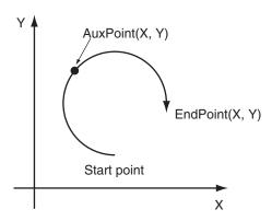
If the start point, border point, and end point are along the same line, if the border point and the end point are at the same point, or if the start point and the border point are the same point, linear interpolation is performed from the start point to the end point.
