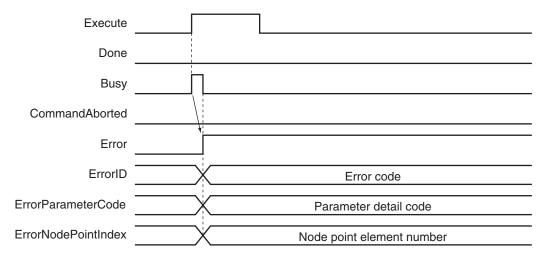
Even if an error occurs during execution of the instruction, the cam data variable specified for *CamTable* retains the same values as before the execution.
