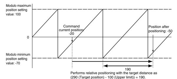
When **1:** \_mcShortestWay (Shortest way) is specified for *Direction*, positioning starts in the direction with the shortest distance between the command current position and the target position.
