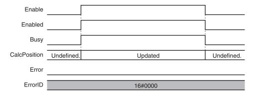
The following timing chart is for when an unused axis is specified or when an MC Test Run in progress.
