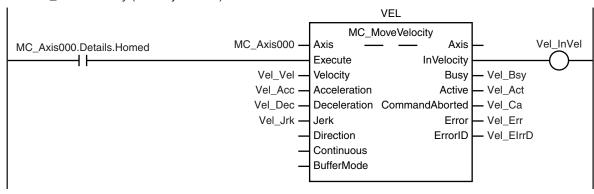
Latch processing is executed after the MC\_MoveVelocity (Velocity Control) instruction is started.
