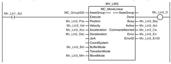
Linear interpolation (4) is executed with multi-execution of instructions after linear interpolation (1) is started.
