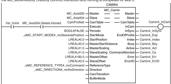
The MC\_CamIn (Start Cam Operation) instruction is executed for axis 5 (slave axis) if *Vel\_InVel* is TRUE for the MC\_MoveVelocity (Velocity Control) instruction and homing is completed for axis 5.
