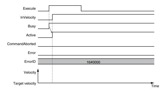
When the *Acceleration* (Acceleration Rate) or *Deceleration* (Deceleration Rate) is 0 and the instruction is executed, the axis will reach the target velocity without accelerating or decelerating.
