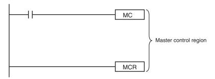
If a motion control instruction is located in the master control region, and the MC input condition is FALSE, the following will occur.
