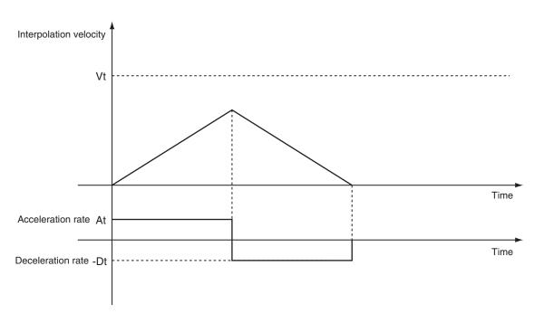
Vt: Specified interpolation velocity, At: Specified acceleration rate, Dt: Specified deceleration rate.
