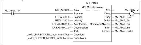
Absolute positioning 3 is executed with multi-execution of instructions to move from  $90.0^{\circ}$  to  $120.0^{\circ}$ . The shortest way is used for the motion direction.
