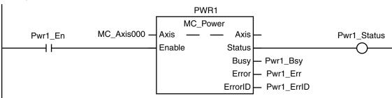
Checking to See If the Specified Axis Exists
