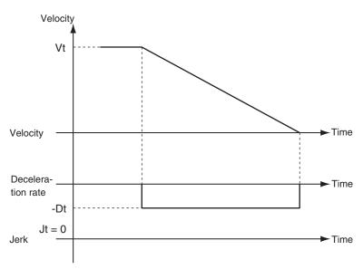
Vt: Velocity when deceleration starts, Dt: Specified deceleration rate, Jt: Specified jerk
