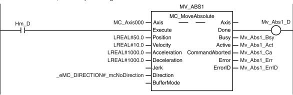
After absolute positioning 1 is started, absolute positioning 2 is started with multi-execution of instructions.
