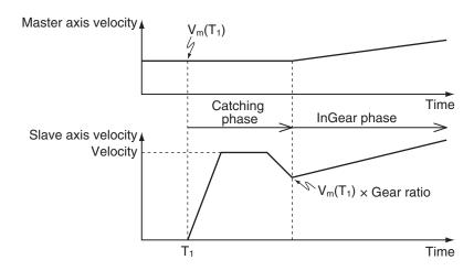
For the *Slave* (Slave Axis) to catch up with the *Master* (Master Axis) for the *MasterSyncPosition* (Master Sync Position) and *SlaveSyncPosition* (Slave Sync Position), the following condition must be met for the *Velocity* (Target Velocity).
