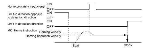
An error occurs and the axis stops if the axis is set to Reverse turn for the limit input operation in both directions and home cannot be detected after moving from the limit input opposite to the home input detection direction to the other limit input.
