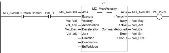
After the MC\_MoveVelocity (Velocity Control) instruction is executed for axis 1, the MC\_DigitalCamSwitch (Enable Digital Cam Switch) instruction is executed for axis 2.
