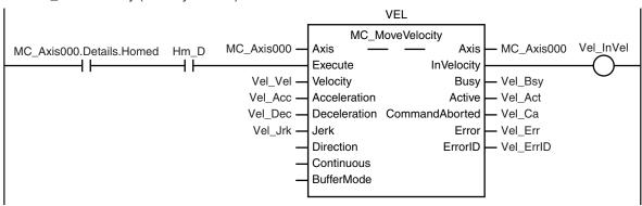
After the MC\_MoveVelocity (Velocity Control) instruction is executed for axis 1, the MC\_TimeStampToPos (Time Stamp to Axis Position Calculation) instruction is executed for axis 2.
