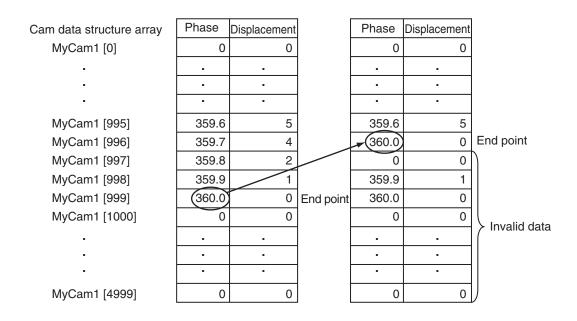
If this instruction is executed for a cam table after the phases for MyCam1[1000] to MyCam1[4997] are changed to anything other than 0, *EndPointIndex* will be 4997.
