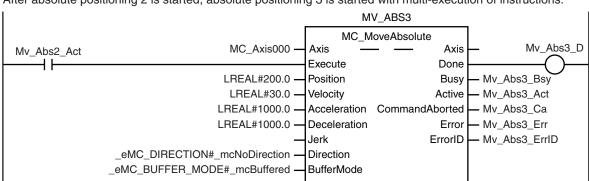
After absolute positioning 2 is started, absolute positioning 3 is started with multi-execution of instructions.
