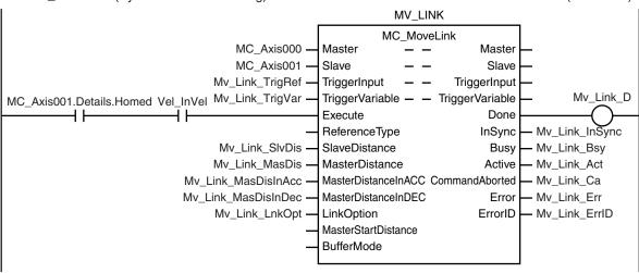
Actuator is TRUE while the axes are synchronized.
