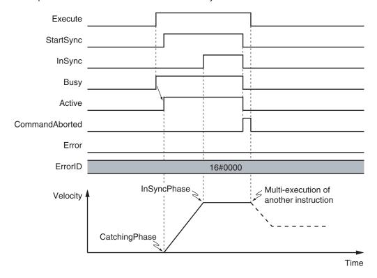
Depending on the setting of the *SlaveSyncPosition*, the axis may not reach the target velocity. An example of this is shown below.
