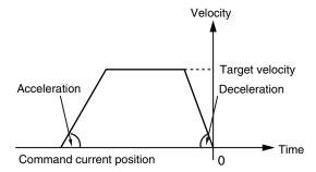
When the *Acceleration* (Acceleration Rate) or *Deceleration* (Deceleration Rate) is 0 and the instruction is executed, it will reach the target velocity without accelerating or decelerating.
