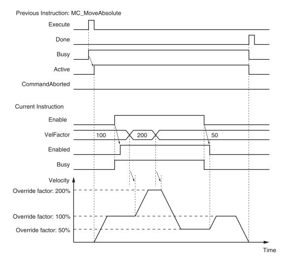
If the MC\_SetOverride instruction is disabled, the target velocity returns to an override factor of 100%.
