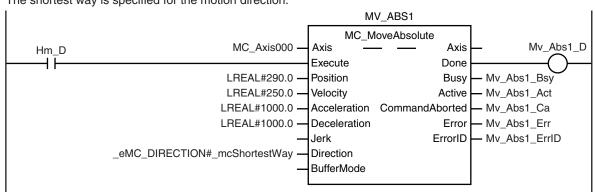
Absolute positioning 2 is executed with multi-execution of instructions to move from  $290.0^{\circ}$  to  $90.0^{\circ}$ . The shortest way is used for the motion direction.
