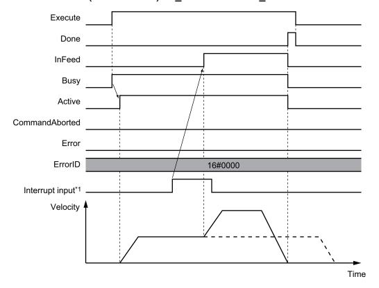
\*1. There may be a delay of up to several control periods from when the interrupt input turns ON until *InFeed* changes to TRUE.
