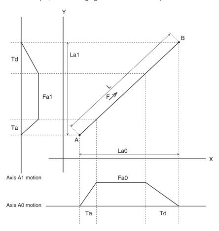
For linear interpolation of four axes, the interpolation velocity and travel distance of each axis determine the target velocities as shown below.
