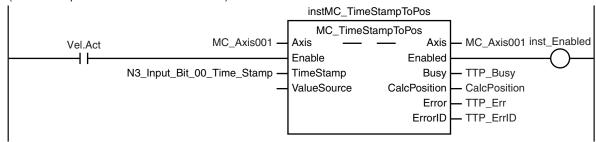
The number of rotations of the encoder axis is counted. (If the current value is less than the previous value, it is assumed that the modulo maximum position has been exceeded.)
