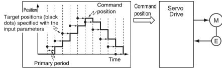
• If this instruction is executed in the priority-16 periodic task, the target position that is specified in the input parameters is output to the Servo Drive in the next periodic task.
