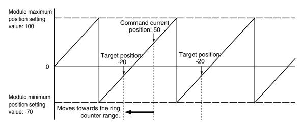
When **4:** \_mcNoDirection (No direction specified) is specified for *Direction*, you can specify a *Position* (Target Position) outside the range specified by the modulo maximum position and modulo minimum position setting values.
