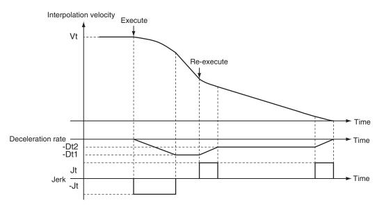
Vt: Velocity when deceleration starts, Dt: Specified deceleration rate, Jt: Specified jerk
