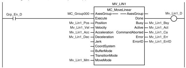
Linear interpolation (2) is executed with multi-execution of instructions after linear interpolation (1) is started.
