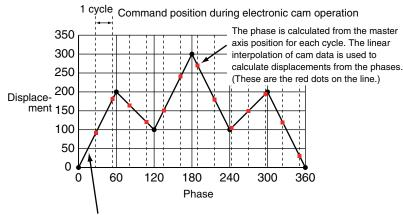
Linearly interpolate between cam data (black dots on the line).
