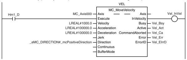
The MC\_CamIn (Start Cam Operation) instruction is executed if *Vel\_InVel* is TRUE for the MC\_MoveVelocity (Velocity Control) instruction.
