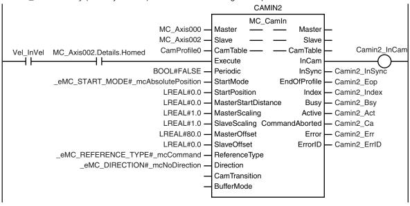
The MC\_CamIn (Start Cam Operation) instruction is executed for axis 4 (slave axis) if *Vel\_InVel* is TRUE for the MC\_MoveVelocity (Velocity Control) instruction and homing is completed for axis 4.
