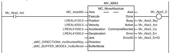
Absolute positioning 4 is executed with multi-execution of instructions to move from 120.0° to 0.0°. The shortest way is used for the motion direction.
