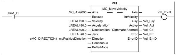
After homing is completed for axis 2 (slave axis), MC\_GearInPos (Positioning Gear Operation) is executed to start gear operation if *Vel\_InVel* of MC\_MoveVelocity is TRUE.
