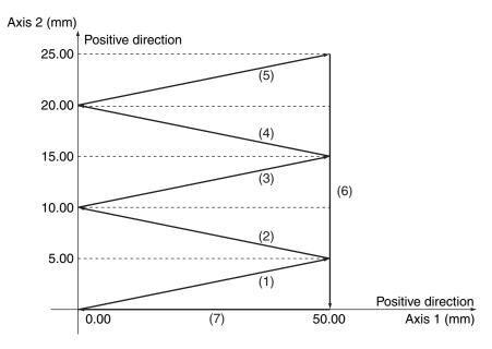
Positioning is performed using linear interpolations in the order (Axis1, Axis2) = (50.00 mm, 5.00 mm)  $\rightarrow$  (0.00 mm, 10.00 mm)  $\rightarrow$  (50.00 mm, 15.00 mm)  $\rightarrow$  (0.00 mm, 20.00 mm)  $\rightarrow$  (50.00 mm, 0.00 mm)  $\rightarrow$  (0.00 mm, 0.00 mm), then stop.
