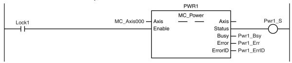
If the Servo Drive for axis 2 is ready, the Servo is turned ON.
