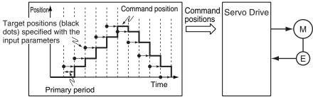
• If this instruction is executed in the priority-16 periodic task, the target positions that are specified in the input parameters are output to the Servo Drive in the next periodic task.
