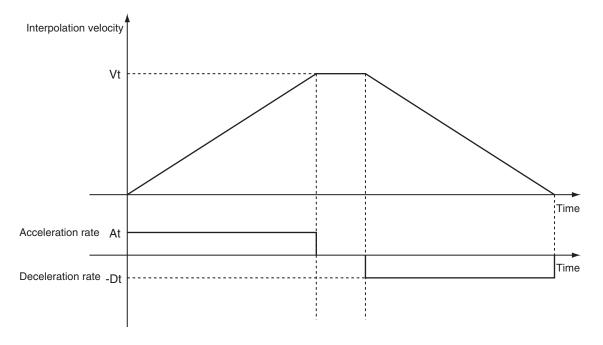
Vt: Specified interpolation velocity, At: Specified acceleration rate, Dt: Specified deceleration rate.
