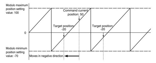
Positioning starts towards the target position within the ring counter range when **4: \_mcNoDirection** (No direction specified) is specified for *Direction*. Therefore, the size relationship between the command current position and the target position determines the direction of travel.
