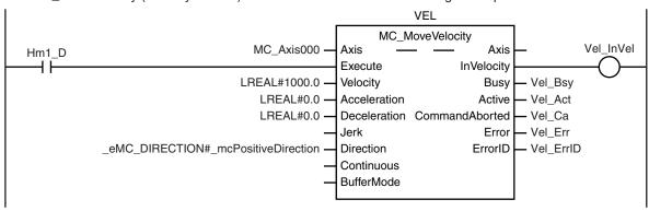
The MC\_CamIn (Start Cam Operation) instruction is executed for axis 2 (slave axis) if *Vel\_InVel* is TRUE for the MC\_MoveVelocity (Velocity Control) instruction and homing is completed for axis 2.
