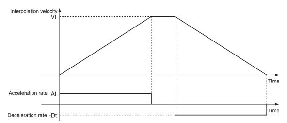
Vt: Specified interpolation velocity, At: Specified acceleration rate, Dt: Specified deceleration rate.
