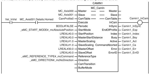
The MC\_CamIn (Start Cam Operation) instruction is executed for axis 3 (slave axis) if *Vel\_InVel* is TRUE for the MC\_MoveVelocity (Velocity Control) instruction and homing is completed for axis 3.
