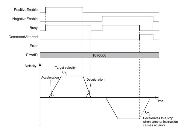
You can specify the *Velocity* (Target Velocity), *Acceleration* (Acceleration Rate), and *Deceleration* (Deceleration Rate) as input variables.
