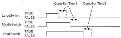
When CompBanTime1 = T#0s and CompBanTime2 = T#0s, the WeightVal value and FixWeightSet-Val value are compared immediately after the valve is opened or closed.
