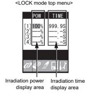
2. Move the cursor to the irradiation power/time to change for each channel using the keys, and press the SET key to apply the setting.
