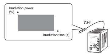
This section describes the procedures from setting the irradiation power to "65%" and the irradiation time to "60 seconds" up to irradiating UV light.
