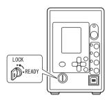
4. Set the power switch on the controller rear to OFF.
