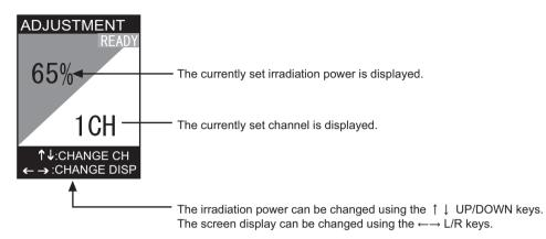
Adjusting the irradiation power in the irradiation power adjustment screen
