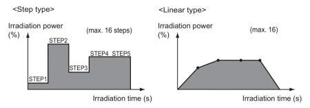
This section describes the procedures for creating a step-type pattern and using that pattern to irradiate UV light.
