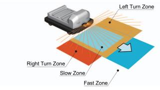
Fig. 1-9 Automated Guided Vehicles, Multiple Zones (AGV)
