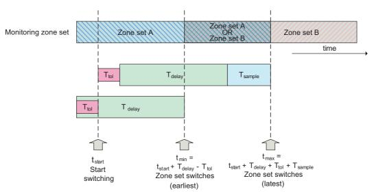
Fig. 2-12 Zone set select input switching and zone set switch.
