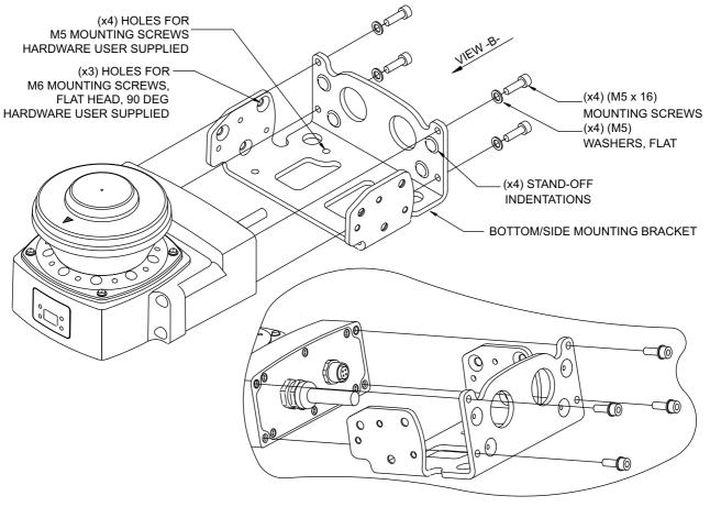
Fig. 4-27 Assembly drawing of OS32C with OS32C-BKT1
