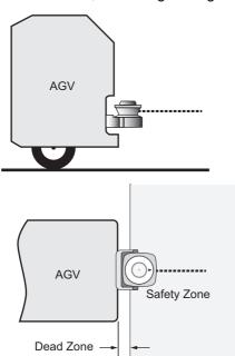
Fig. 4-13 Projecting Installation at Front of Vehicle
