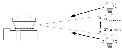
Fig. 4-1 Angle between scan plane and light source
