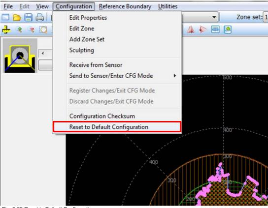
Fig. 3-93 Reset to Default Configuration
