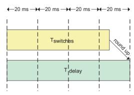
Fig. 2-11 Zone Delay configuration.
