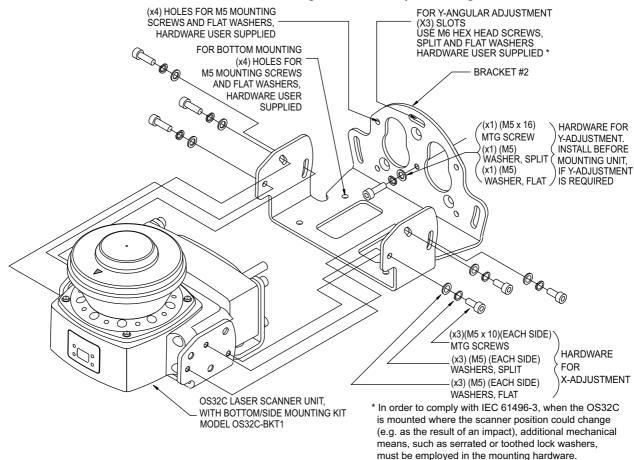
Fig. 4-31 Assembly drawing of OS32C with OS32C-BKT1 and OS32-BKT2
