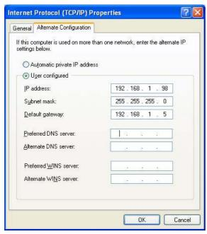
Fig. 3-10 Alternate Configuration
