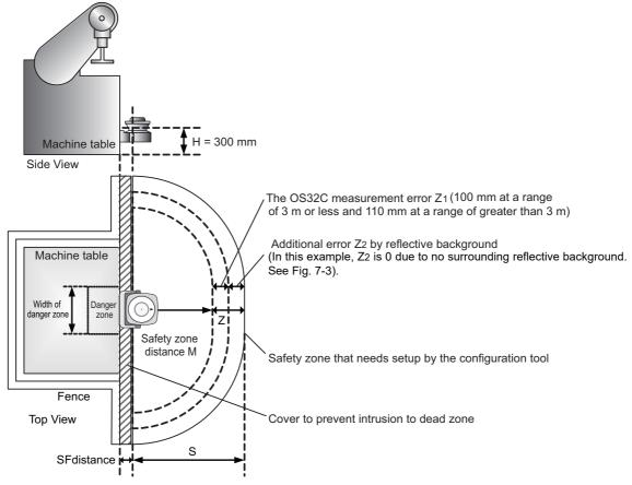
Fig. 4-7 Installation on a Machine
