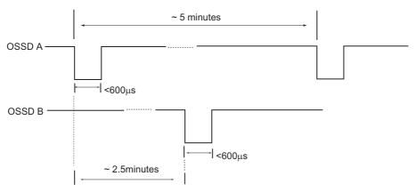
Fig. 2-1 OSSD Test Pulses
