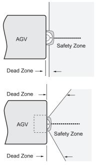
Fig. 4-14 Installation with Bodywork of AGV
