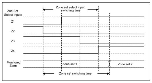
Fig. 2-9 Zone Switching example
