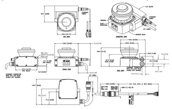
Fig. 4-19 OS32C with Side Cable Entry Dimensional Drawing
