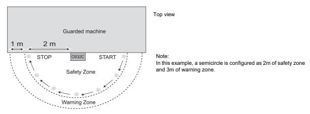
Fig. 6-1 Testing a Horizontal Safety Zone
