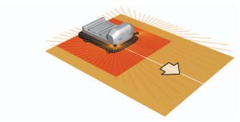
Fig. 1-10 Automated Guided Vehicles (AGV), Two Scanners, Three Sided
