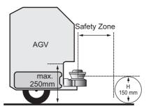
Fig. 4-12 Installation on Automated Guided Vehicle
