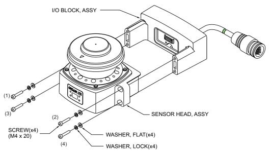
Fig. 7-9 Sensor Block Replacement
