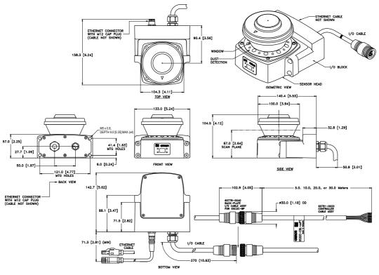
Fig. 4-18 OS32C with Back Cable Entry Dimensional Drawing
