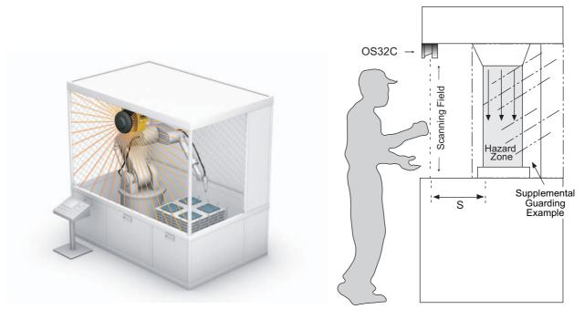
Fig. 4-11 Hand Detection Protection
