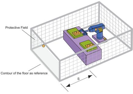
Fig. 4-10 Perpendicular Approach Installation
