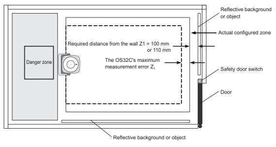
Fig. 7-5 Installing Door on Entrance
