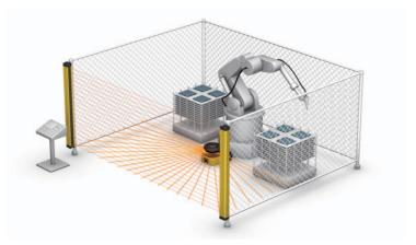
Fig. 1-4 Internal Robot Cell Guarding
