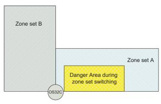
Fig. 7-19 Danger area during zone set switching
