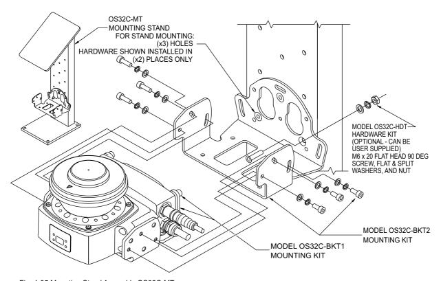
Fig. 4-35 Mounting Stand Assembly OS32C-MT
