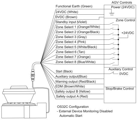
Fig. 5-4 Connecting to AGV Controls
