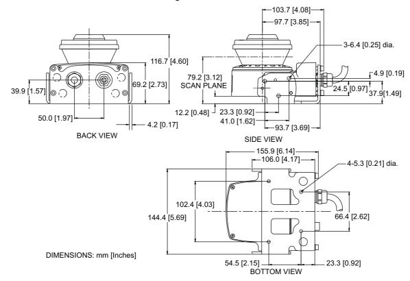
Fig. 4-26 External dimensional drawing of OS32C with OS32C-BKT1
