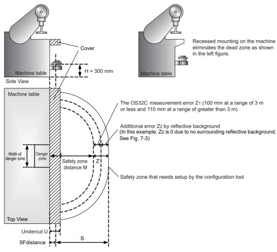
Fig. 4-9 Installation on a machine with cover
