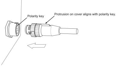
Fig. 4-38 Aligning to polarity key
