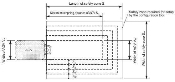
Fig. 4-17 Installation on AGV
