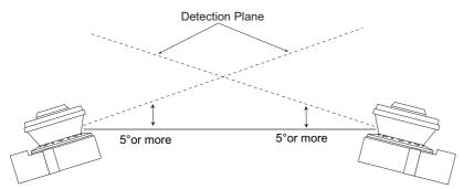
Fig. 4-2 Offset Scanning Level by Tilting
