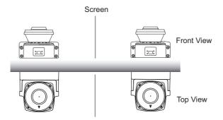
Fig. 4-4 Separation using a screen
