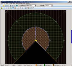
Fig. 3-92 Detection Zone in Intruding Parts
