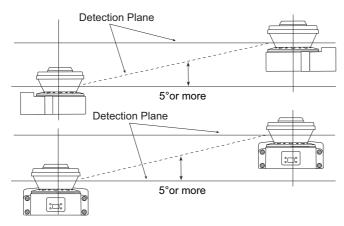
Fig. 4-3 Offset Parallel Scanning Levels by Different Installation Height
