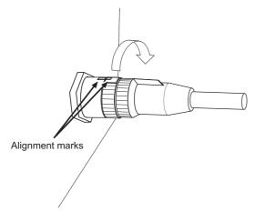
Fig. 4-40 Aligning the XS5 Plug
