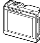
Used to check images and set the judgement parameters. It can also be used to save measurement results and check status during operation.
