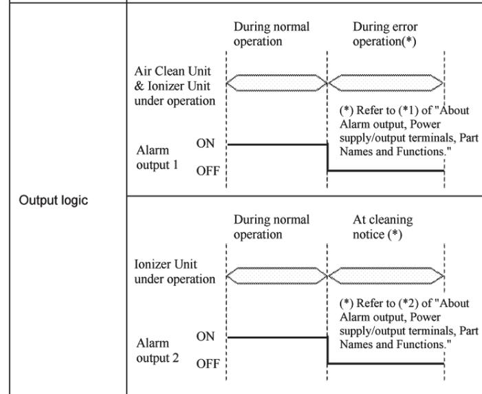
Alarm output is ON, when the power for a ZN-A is OFF.
