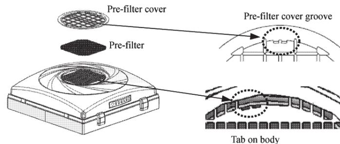
2. Replacing HEPA Filter
