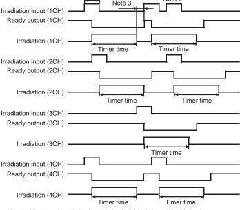
Note 1: All-channel irradiation input during individual channel irradiation is not accepted Note 2: Irradiation input during irradiation (at Ready output ON) is not accepted. Note 3: An interval for the next irradiation input after an irradiation stop must be at least
