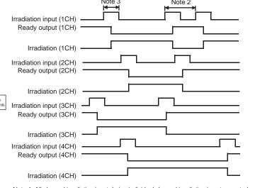
Note 1: All-channel irradiation input during individual channel irradiation is not accepted Note 2: An interval between signal inputs must be at least 400 ms.
