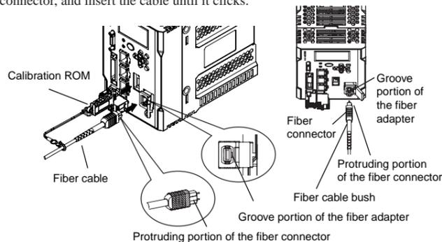
Grip the bush portion of the fiber cable (black) on the right-hand figure, align the groove portion of the fiber adapter with the protruding portion of the fiber connector, and insert the cable until it clicks.
